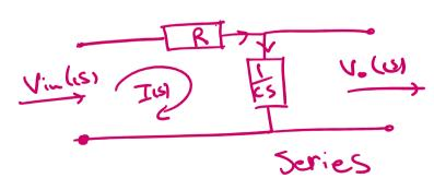
$$V_{in}(s) = I_{(s)} \times Z_{equ} = I_{(s)} \times (\frac{1}{cs} + R)$$
