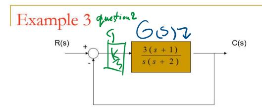
If r(t) = (2+3t)u(t), find the steady state error  $(e_{ss})$  for the given system.
