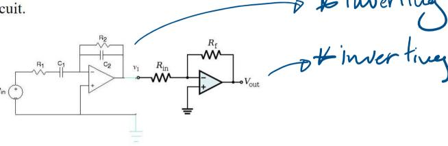
$$Tf_{1} \times Tf_{2} = -\frac{1}{R_{2}} + \frac{1}{c_{5}} \times -\frac{RP}{Riw}$$
