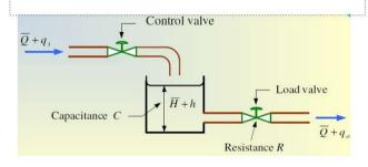
$\overline{H}=$  steady-state head (before any change has occurred), m. h= small deviation of head from its steady-state value, m.
