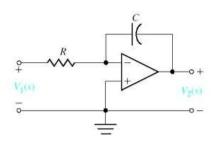
$$\frac{V_2(s)}{V_1(s)} = \frac{-1}{RCs}$$
