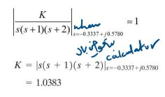
The third closed loop pole at K=1.0383 can be obtained as
