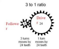
number of teeth of input gear \_ Input Torque \_ Output Speed  $\frac{1}{number\ of\ teeth\ of\ ouput\ gear} = \frac{1}{number\ Torque} = \frac{1}{nput\ Speed}$
