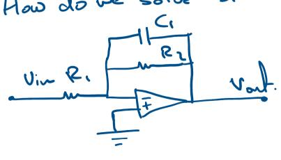
1. we determine the type of amplifier - in this case, inverting.
