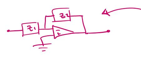
$$\frac{Z_1 = R_1}{Z_2} = \frac{1}{CS} + \frac{1}{R_2} = \frac{R_2 + CS}{CSR_2}$$
