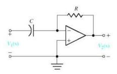
$$\frac{V_2(s)}{V_1(s)} = -RCs$$
