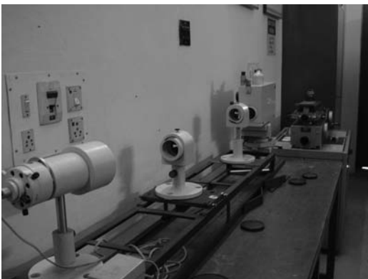
Fig. C.23 Autocollimator for the measurement of straightness
