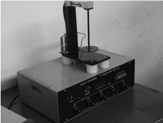
Fig. C.51 Typical set-up for strain measurement
