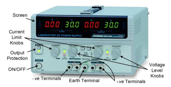
When connecting the DC power supply to the breadboard use suitable wires to connect both the "+ terminal" (high voltage terminal) and the "- terminal" (low voltage terminal) to your circuit. "Real GND" is for earth grounding and it is connected to the device chassis. In this Lab we will not use the earth grounding terminal.
