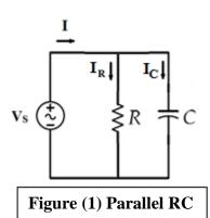
\* Now we know that resistor current  $I_R$  and resistor voltage  $V_R$  (which equals  $V_S$ ) are in phase or have the same phase angle (there zero crossings are the same on the time axis) and  $V_R$  is greater than  $I_R$  in magnitude.
