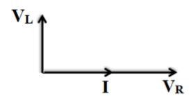
\* Finally, the source voltage  $V_S$  equals the <u>vector summation</u> of  $V_R$  and  $V_L$ : Step4
