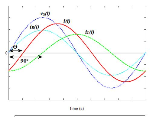
Figure (3) Parallel RL Circuit Time Domain Representation
