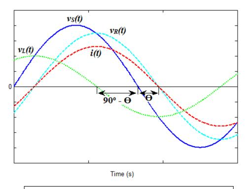
Figure (3) Series RL Circuit Time Domain Representation
