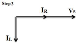
\* Finally, the source current I equal the <u>vector summation</u> of  $I_R$  and  $I_L$ :
