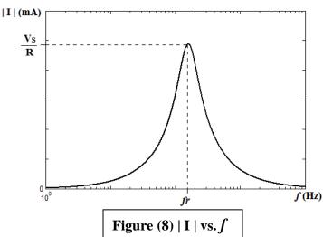
\* Because **I** is inversely proportional  $|V_{L}|, |V_{C}|, |V_{R}|$  (V) to **Z**, the total current **I** will increase before *f* reaches *fr* then decrease when *f* exceeds *fr* and it's value is maximum at resonance frequency *fr* and equals  $V_{s}/R$  as shown in figure (8).
