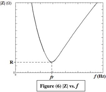
\*  $\Theta$  ranges from -90° to 90° (-90° <  $\Theta$  < 90°). And since  $|\Theta| = \tan^{-1} \frac{|X_L - X_C|}{R}$  and the  $\tan^{-1}$  function is increasing on the interval from -90° to 90°, the phase shift  $\Theta$  (or the current angle  $\overset{\checkmark}{\rightarrow}$  I) will decrease before *f* reach *fr* then increase when *f* exceeds *fr* and it's value is minimum at resonance frequency and equals **zero** as shown in figure (7).
