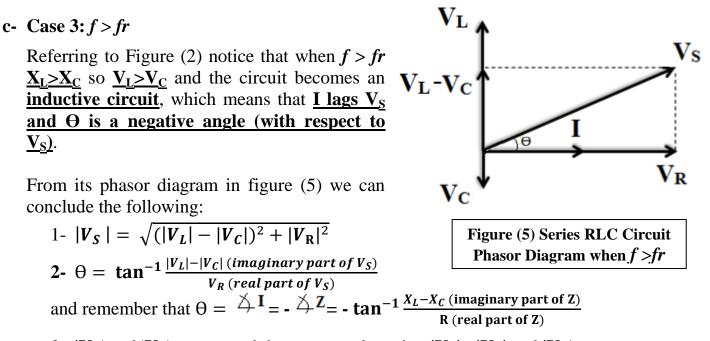
3-  $|V_C|$  and  $|V_L|$  can exceed the source voltage but  $|V_L|$  -  $|V_C|$  and  $|V_R|$  cannot.
