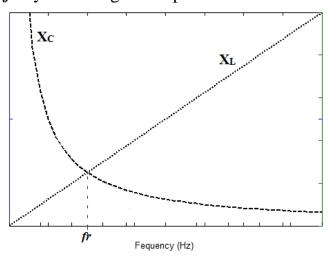
\* Figure (2) shows important plot of how capacitor impedance  $X_C$  and inductor impedance  $X_L$  change with frequency and the place of *fr* on the plot (in this case when  $X_C$  equal  $X_L$ ).
