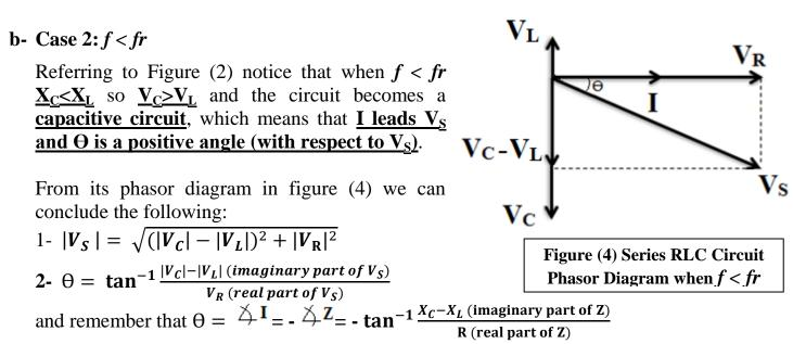
3-  $|V_C|$  and  $|V_L|$  can exceed the source voltage but  $|V_C|$  -  $|V_L|$  and  $|V_R|$  cannot.
