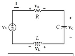
Figure (1) Series RLC circuit
