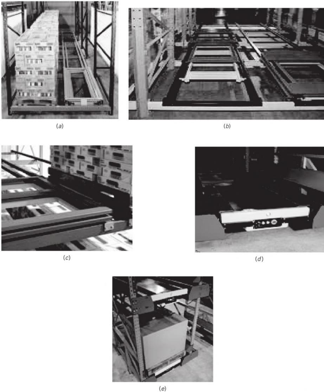
Figure 10.37 Examples of shuttles used for deep lane storage. (a) Courtesy of Ridg-U-Rak Inc. (b) Courtesy of King Material Handling, Inc. (c), (d), and (e). Courtesy of Konstant Products, Inc.
