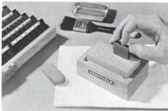
Fig. 4-17. The use of a dressing stone to remove minute burrs from the wringing surface of gage blocks.
