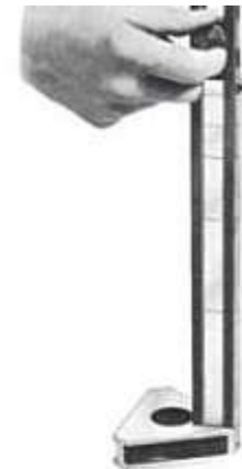
Fig. 4-14. (Left) Gage blocks assembled with foot plate and scriber jaw for surface plate layout work.
