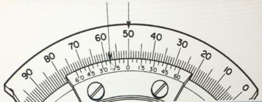
The reading of the vernier bevel protractor is -----
