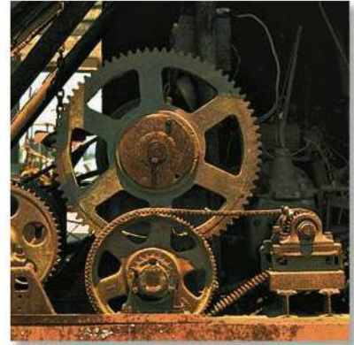
The gears used in the operation of a crane all rotate about fixed axes. Engineers must be able to relate their angular motions in order to properly design this gear system.
