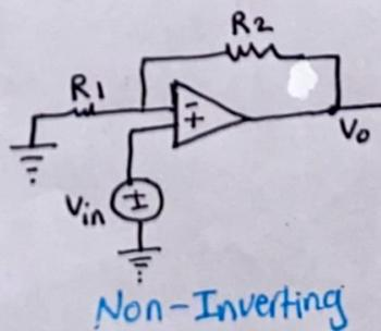
$$TF = \frac{V_o}{V_{in}} = 1 + \frac{R_2}{R_1}$$
