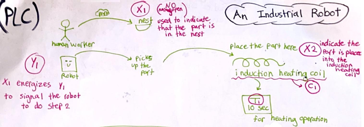
$X_1$  energizes  $Y_1$  to signal the robot to do step 2
