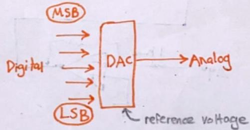
$$V_{out} = V_R (b_{12}^{-1} + b_{22}^{-2} + \dots + b_{n2}^{-n})$$
