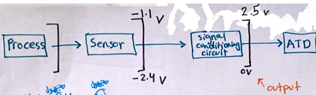
$$V_{out} = mV_{in} + V_0$$
