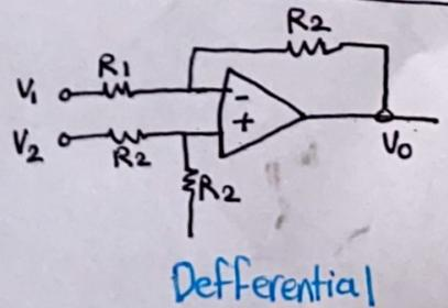
$$TF = \frac{V_o}{V_{in}} = \frac{R_2}{R_1} (V_2 - V_1)$$
