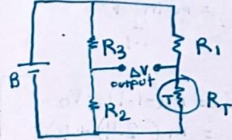
$$\Delta V = E \left( \frac{R_2}{R_2 + R_3} - \frac{R_T}{R_T + R_1} \right)$$
