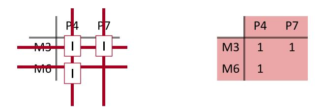
Cell #3 will produce parts P4 and P7 with Machines M3 and M6
