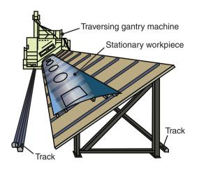
**Figure 16.55:** Schematic illustration of a peen-forming machine to shape a large sheet-metal part, such as an aircraft-skin panel. Note that the sheet is stationary and the peening head travels along its length. *Source:* Metal Improvement Company.
