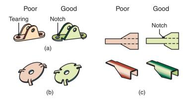
**Figure 16.62:** Application of notches to avoid tearing and wrinkling in right-angle bending operations. *Source:* Courtesy of Society of Manufacturing Engineers.
