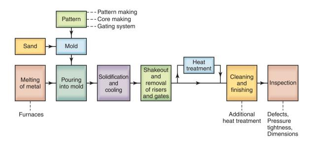
Figure 11.2: Outline of production steps in a typical sand-casting operation.
