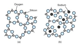
**Figure 8.5:** Schematic illustration of the structure of silica glass. (a) Pure silica glass, in the form of  $(SiO_2)_n$  random structure; (b) partially depolymerized glass. Note that a fourth bond for each silicon is outside the plane shown.
