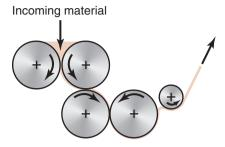
**Figure 19.20:** Schematic illustration of calendering. Sheets produced by this process subsequently are used in thermoforming. The process also is used in the production of various elastomer and rubber products.
