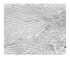
**Figure 4.9:** Microstructure of pearlite in 1080 steel, formed from austenite of eutectoid composition. In this lamellar structure, the lighter regions are ferrite and the darker regions are carbide. Magnification:  $2500 \times$ .
