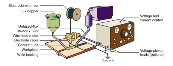
**Figure 30.10:** Schematic illustration of the submerged-arc welding process and equipment. The unfused flux is recovered and reused.
