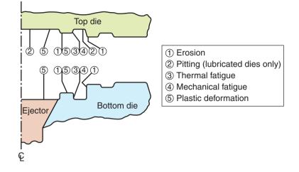
**Figure 33.12:** Types of wear observed in the cavity of a single pair of dies used for hot forging. *Source:* After T.A. Dean.
