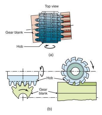
**Figure 24.34:** (a) Hobs, used to machine gear teeth; (b) schematic illustration of gear cutting with a hob. *Source:* (a) Courtesy of Sandvik Coromant.
