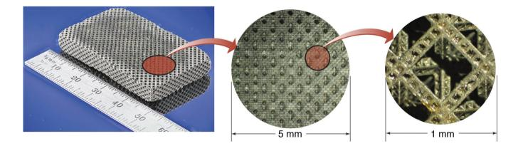
**Figure 6.5:** Nickel alloy hierarchical metamaterial and critical features across two orders of magnitude in length scale. (a) Large-area, high-resolution additive manufacturing of hierarchical metamaterials. (b)–(c) Optical microscope images of bulk hierarchical lattice material with a network of hierarchical stretch-dominated octet unit cells. *Source:* Xiaoyu (Rayne) Zheng, Virginia Tech.
