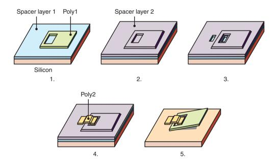
**Figure 29.7:** Schematic illustration of the steps required to manufacture a hinge. 1. Deposition of a phosphosilicate glass (PSG) spacer layer and polysilicon layer (see Fig. 29.3). 2. Deposition of a second spacer layer. 3. Selective etching of the PSG. 4. Deposition of polysilicon to form a staple for the hinge. 5. After selective wet etching of the PSG, the hinge can rotate.
