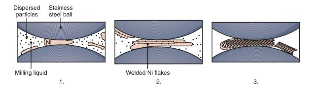
**Figure 17.7:** Mechanical alloying of nickel particles with dispersed smaller particles. As the nickel particles are flattened by the balls, the second, smaller phase is impressed into the nickel surface and eventually is dispersed throughout the particle due to successive flattening, fracture, and welding that occur.
