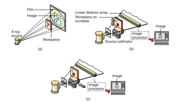
**Figure 36.11:** Three methods of radiographic inspection: (a) conventional radiography, (b) digital radiography, and (c) computed tomography. *Source:* ASM International.
