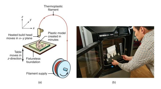
**Figure 20.5:** (a) Schematic illustration of the fused-deposition-modeling process. (b) Removing a part from an F370, a popular fused-deposition-modeling machine. *Source:* Courtesy of Stratasys, Inc.
