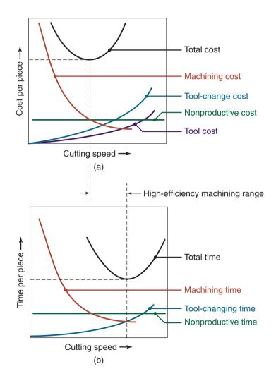
**Figure 25.18:** Graphs showing (a) cost per piece and (b) time per piece in machining. Note the optimum speeds for both cost and time. The range between the two is known as the *high-efficiency machining range*.
