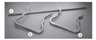
**Figure 16.45:** Sequence of operations in producing a tube-hydroformed component: (1) tube as cut to length; (2) after bending; (3) after hydroforming. *Source:* Courtesy of B. Longhouse, Vari-Form, Inc.
