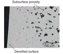
**Figure 17.24:** Micrograph of a PM material surface after roll densification. Note the low porosity near the surface, increasing the material's ability to support contact stresses and resist fatigue. *Source:* Courtesy of Capstan Atlantic Corp.
