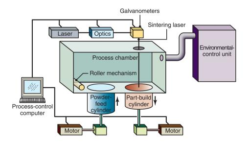
Figure 20.12: Schematic illustration of the selective-laser-sintering process.
