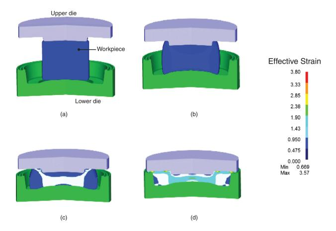
**Figure 14.18:** Deformation of a blank during forging as predicted by the software program DEFORM, based on the finite-element method of analysis. *Source:* Courtesy of Scientific Forming Technologies Corporation.
