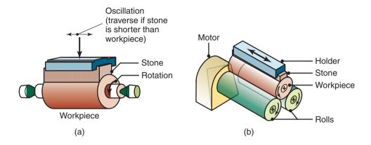
**Figure 26.30:** Schematic illustrations of the superfinishing process for a cylindrical part. (a) Cylindrical microhoning. (b) Centerless microhoning.
