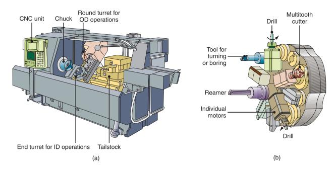
**Figure 23.11:** (a) A computer-numerical-control lathe with two turrets. (b) A typical turret equipped with 10 tools, some of which are powered.
