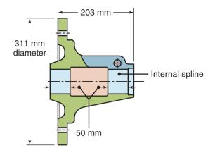
Figure 24.27: Example of a part with internal splines that were produced by broaching.
