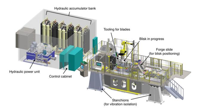
**Figure 31.19:** Illustration of a modern linear friction welding system for production of jet engine bladed disks (blisks). *Source:* After D. Adams, MTI Welding.
