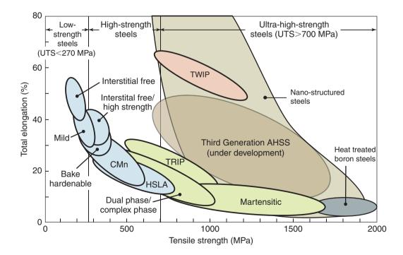
Figure 5.6: Comparison of advanced high-strength steels.
