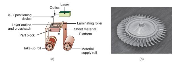
**Figure 20.16:** (a) Schematic illustration of the laminated-object-manufacturing process. (b) Turbine prototype made by LOM. *Source:* Courtesy of M. Feygin, Cubic Technologies, Inc.
