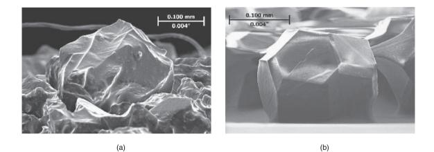
**Figure 26.1:** Typical abrasive grains; note the angular shape with sharp edges. (a) A single, 80-mesh  $Al_2O_3$  grit in a freshly dressed grinding wheel; (b) an 80/100 mesh diamond grit. Diamond and cubic boron nitride grains can be manufactured in various geometries, including the "blocky" shape shown. *Source:* Courtesy of J. Badger.
