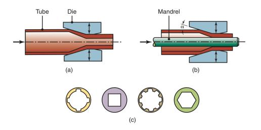
**Figure 14.16:** (a) Swaging of tubes without a mandrel; note the increase in wall thickness in the die gap. (b) Swaging with a mandrel; note that the final wall thickness of the tube depends on the mandrel diameter. (c) Examples of cross sections of tubes produced by swaging on shaped mandrels. Rifling (internal spiral grooves) in small gun barrels can be made by this process.
