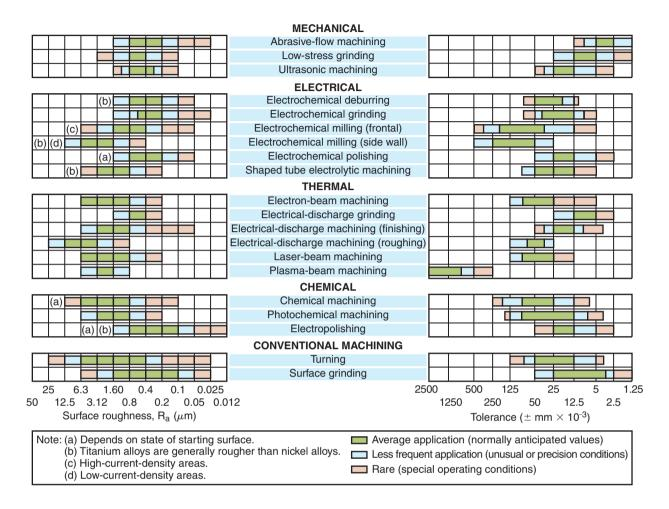
**Figure 33.5:** Surface roughness and tolerances obtained in various machining processes; note the wide range within each process (see also Fig. 23.14). *Source: Machining Data Handbook,* 3rd ed. Copyright 1980. Used by permission of Metcut Research Associates, Inc.
