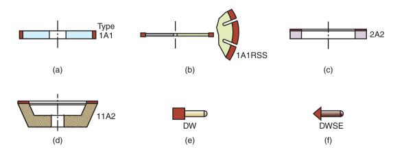
**Figure 26.6:** Examples of superabrasive wheel configurations. The annular regions (rims) are grinding surfaces; the wheel itself (core) generally is made of metal or composites. The bonding materials for superabrasives are (a), (d), and (e) resinoid, metal, or vitrified; (b) metal; (c) vitrified; and (f) resinoid.
