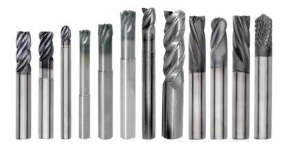
**Figure 24.12:** A selection of end mills. The flute depth and helix angle are selected based on whether it is a roughing or finishing cut. Note the variety of geometries of the end of the mill; with the proper cutter, a radius, chamfer, or flat surface can be machined. *Source:* Courtesy of Kennametal, Inc.
