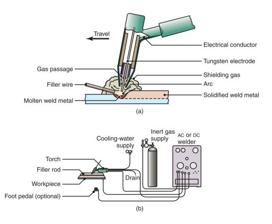
**Figure 30.5:** (a) The gas tungsten-arc welding process, formerly known as TIG (for tungsten–inert gas) welding. (b) Equipment for gas tungsten-arc welding operations.
