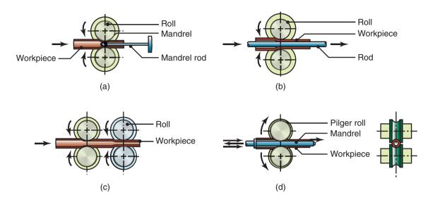
**Figure 13.20:** Schematic illustration of various tube-rolling processes: (a) with a fixed mandrel; (b) with a floating mandrel; (c) without a mandrel; and (d) pilger rolling over a mandrel and a pair of shaped rolls. Tube diameters and thicknesses also can be changed by other processes, such as drawing, extrusion, and spinning.
