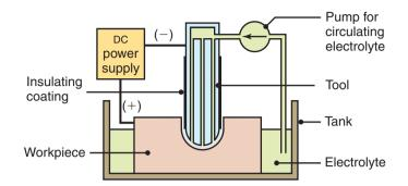
Figure 27.4: Schematic illustration of the electrochemical machining process.
