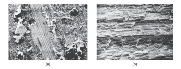
**Figure 21.21:** Machined surfaces produced on steel (highly magnified), as observed with a scanningelectron microscope: (a) turned surface and (b) surface produced by shaping. *Source:* After J T. Black and S. Ramalingam.
