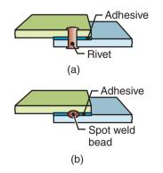
**Figure 32.13:** Two examples of combination joints, for purposes of improved strength, air or liquid tightness, and resistance to crevice corrosion.
