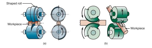
**Figure 13.14:** Two examples of the roll-forging operation, also known as *cross rolling*. Tapered leaf springs and knives can be made by this process. *Source:* After J. Holub.
