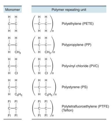
**Figure 7.2:** Molecular structure of various polymers. These are examples of the basic building blocks for plastics.
