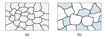
**Figure 4.3:** (a) Schematic illustration of grains, grain boundaries, and particles dispersed throughout the structure of a two-phase system, such as a lead–copper alloy. The grains represent lead in solid solution in copper, and the particles are lead as a second phase. (b) Schematic illustration of a two-phase system consisting of two sets of grains: dark and light. The blue grains and the white grains have separate compositions and properties.
