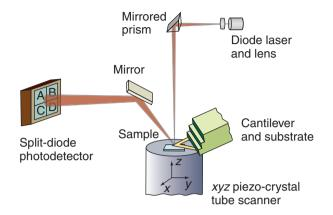
**Figure 29.27:** Schematic illustration of an atomic-force microscope. A probe is mounted on a cylinder containing piezoelectric material; this arrangement allows translation of the probe in three dimensions. A laser reflected from a mirror on the back of the probe onto a set of photosensors allows measurement of the probe's location and monitoring of interactions with a sample surface.
