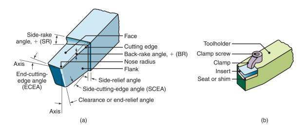
**Figure 21.10:** (a) Schematic illustration of a right-hand cutting tool. The various angles on these tools and their effects on machining are described in Section 23.2. Although these tools traditionally have been produced from solid-tool steel bars, they have been replaced largely with (b) inserts, typically made of carbides and other materials; they are available in a wide variety of shapes and sizes.
