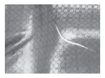
**Figure 16.15:** The deformation of the grid pattern and the tearing of sheet metal during forming. The major and minor axes of the circles are used to determine the coordinates on the forming-limit diagram in Fig. 16.14b. *Source:* After S.P. Keeler.
