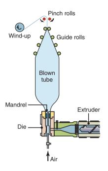
**Figure 19.5:** Schematic illustration of the production of thin film and plastic bags from tube–first produced by an extruder and then blown by air.
