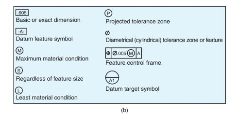
**Figure 35.22:** Geometric characteristic symbols to be indicated on engineering drawings of parts to be manufactured. *Source:* Courtesy of The American Society of Mechanical Engineers.
