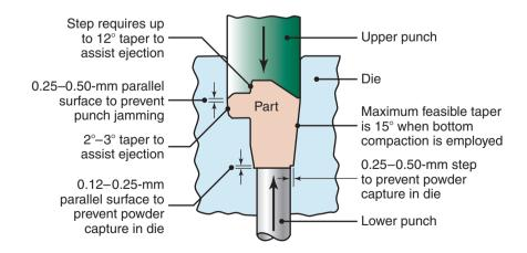
**Figure 17.25:** Die geometry and design features for powder-metal compaction. *Source:* Courtesy of the Metal Powder Industries Federation.
