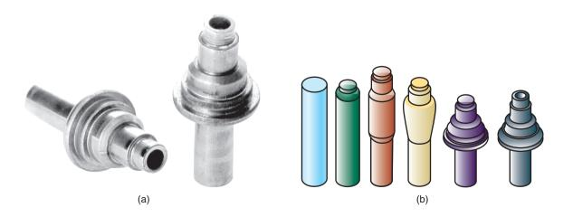
**Figure 14.14:** (a) The stepped pin used in Case Study 14.1. (b) Illustration of the steps used to produce the stepped pin. *Source:* Courtesy of National Machinery, LLC.
