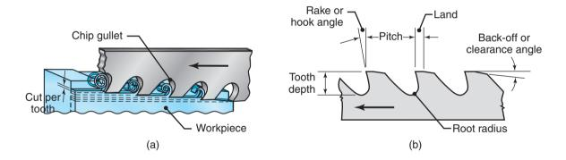
Figure 24.24: (a) Cutting action of a broach, showing various features. (b) Terminology for a broach.
