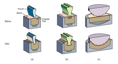
**Figure 16.41:** Examples of the bending and embossing of sheet metal with a metal punch and with a flexible pad serving as the female die.
