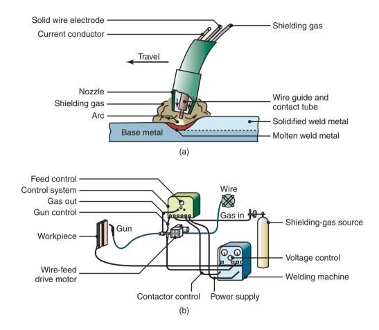
**Figure 30.11:** (a) Schematic illustration of the gas metal-arc welding process, formerly known as MIG (for metal inert-gas) welding. (b) Basic equipment used in gas metal-arc welding operations.
