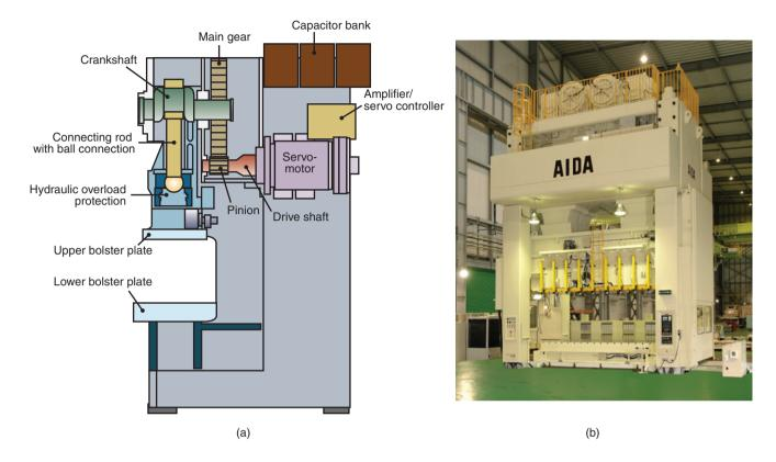
**Figure 14.20:** (a) Schematic illustration of a servo press, with the power source and transmission components highlighted. (b) An example of a servo press, with a 23,000 kN (2250 metric tons) capacity. *Source:* Courtesy of Aida Engineering, Inc.
