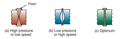
**Figure 31.4:** Shape of the fusion zones in friction welding as a function of the axial force applied and the rotational speed.
