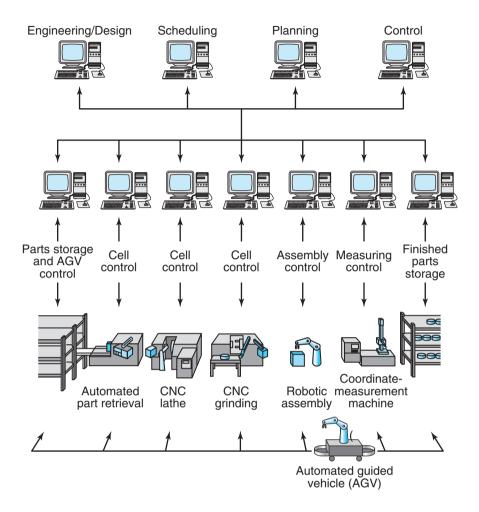
**Figure 38.1:** A schematic illustration of a computer-integrated manufacturing system. The manufacturing cells and their controls shown at the lower left are described in Section 39.2. *Source:* After U. Rembold.
