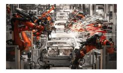
**Figure 37.22:** Example of industrial robot applications. Spot welding automobile bodies with industrial robots. *Source:* Shutterstock/Jensen.
