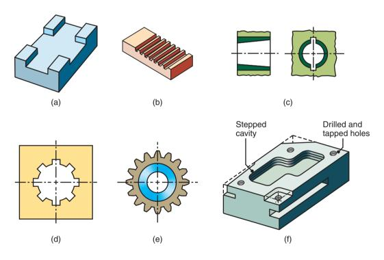
**Figure 24.1:** Typical parts and shapes that can be produced with the machining processes described in this chapter.
