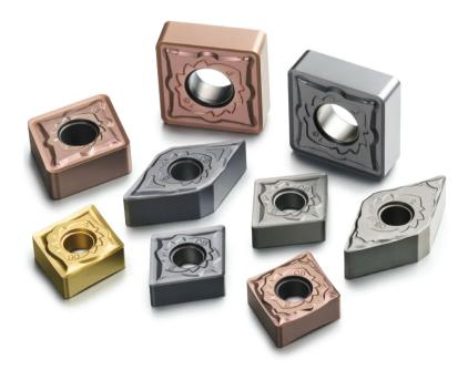
**Figure 22.2:** Typical cutting tool inserts with various shapes and chip-breaker features: Round inserts also are available, as can be seen in Figs. 22.3c and 22.4. The holes in the inserts are standardized for interchangeability in toolholders. *Source:* Courtesy of Kennametal, Inc.
