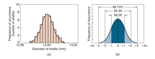
**Figure 36.3:** (a) A histogram of the number of shafts measured and their respective diameters. This type of curve is called a frequency distribution. (b) A normal distribution curve indicating areas within each range of standard deviation. Note that the greater the range, the higher is the percentage of parts that fall within it.
