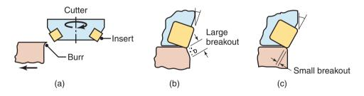
**Figure 24.17:** Edge defects in face milling: (a) burr formation along workpiece edge, (b) breakout along workpiece edge, and (c) how it can be avoided by increasing the lead angle (see also last row in Table 24.3).
