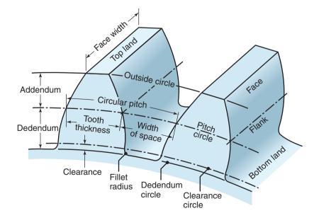
Figure 24.32: Nomenclature for an involute spur gear.
