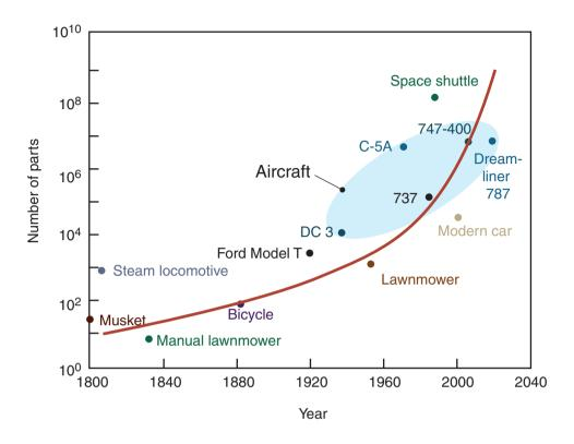
Figure I.1: Increasing complexity of products since the Industrial Revolution. Source: After J. Jeswiet.
