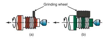
Figure 26.21: Thread grinding by (a) traverse and (b) plunge grinding.
