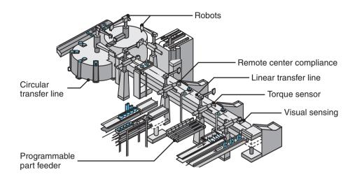
Figure 37.23: Automated assembly operations using industrial robots and circular and linear transfer lines.
