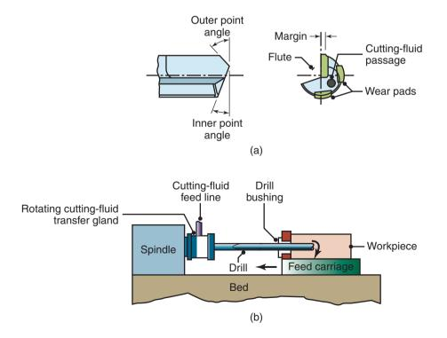
**Figure 23.23:** (a) A gun drill, showing various features. (b) Schematic illustration of the gun-drilling operation.
