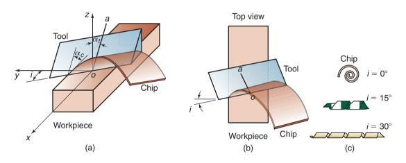
**Figure 21.9:** (a) Schematic illustration of cutting with an oblique tool; note the direction of chip movement. (b) Top view, showing the inclination angle, *i*. (c) Types of chips produced with tools at increasing inclination angles.
