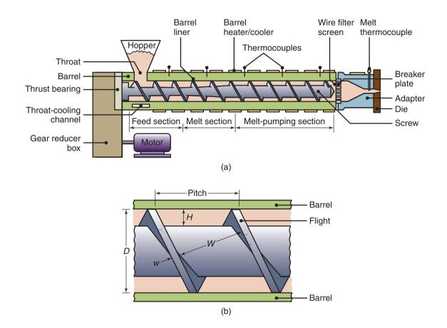
**Figure 19.2:** Common extrusion die geometries: (a) Schematic illustration of a typical screw extruder. (b) Geometry of an extruder screw metering or pumping section. Complex shapes can be extruded with relatively simple and inexpensive dies.
