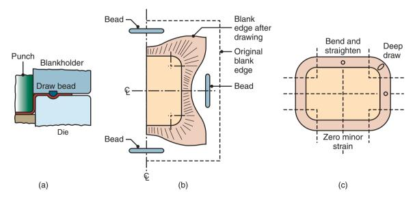
**Figure 16.36:** (a) Schematic illustration of a draw bead. (b) Metal flow during the drawing of a box-shaped part while using beads to control the movement of the material. (c) Deformation of circular grids in the flange in deep drawing.
