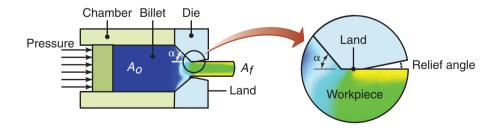
**Figure 15.4:** Process variables in direct extrusion. The die angle, reduction in cross section, extrusion speed, billet temperature, and lubrication all affect the extrusion pressure. The contour plot shows effective strain as obtained from a finite element simulation for the geometry shown.
