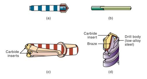
**Figure 23.22:** Various types of drills. (a) Spade drill; (b) straight-flute drill; (c) drill with indexable carbide inserts; (d) drill with brazed-carbide tip.
