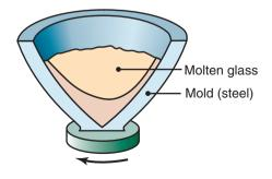
Figure 18.13: Centrifugal casting of glass. Source: Courtesy of Corning Glass Works.
