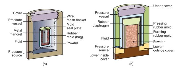
**Figure 17.14:** Schematic diagram of cold isostatic pressing. Pressure is applied isostatically inside a high-pressure chamber. (a) The wet bag process to form a cup-shaped part; the powder is enclosed in a flexible container around a solid-core mandrel. (b) The dry bag process used to form a PM cylinder.
