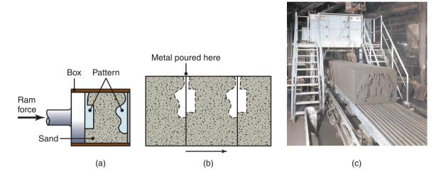
**Figure 11.7:** Vertical flaskless molding. (a) Sand is squeezed between two halves of the pattern. (b) Assembled molds pass along an assembly line for pouring. (c) A photograph of a vertical flaskless molding line. *Source:* Courtesy of American Foundry Society.
