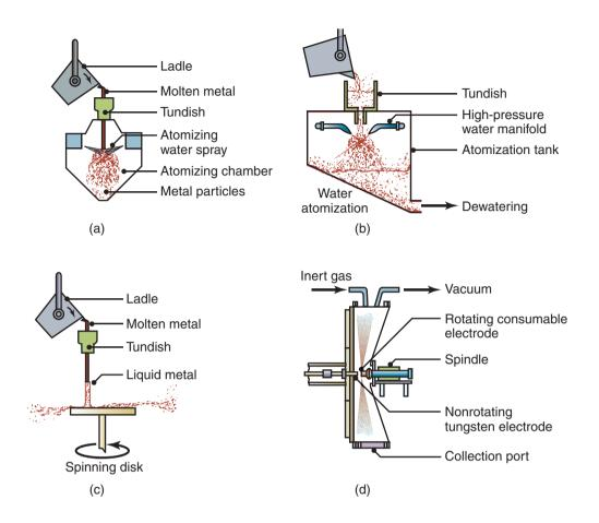
**Figure 17.5:** Methods of metal-powder production by atomization: (a) gas atomization; (b) water atomization; (c) centrifugal atomization with a spinning disk or cup; and (d) atomization with a rotating consumable electrode.
