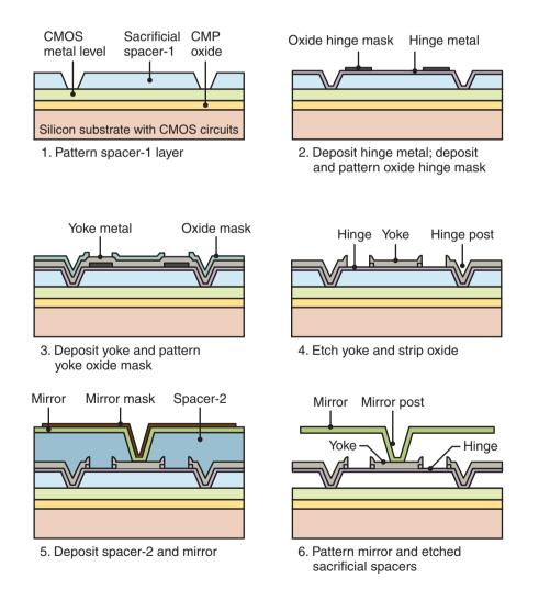
Figure 29.10: Manufacturing sequence for the Texas Instruments DMD device.
