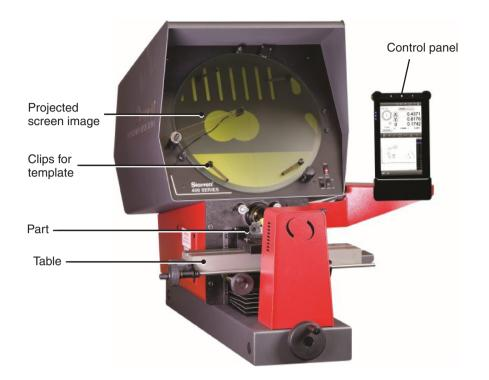
**Figure 35.10:** A horizontal-beam contour projector with a 0.4 m-diameter screen with 150-W tungsten halogen illumination. *Source:* Courtesy of L.S. Starrett Company, Precision Optical Division.
