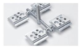
**Figure 17.18:** A single shot of metal injection molded components, with sprue, runners, and gates (see also Fig. 19.10). *Source:* Courtesy HARBEC, Inc.
