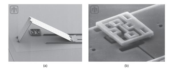
**Figure 29.6:** (a) SEM image of a deployed micromirror, incorporating six hinges. (b) Detail of a micromirror hinge. *Source:* Courtesy of Sandia National Laboratories.
