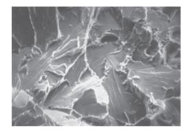
**Figure 2.26:** Fracture surface of steel that has failed in a brittle manner. The fracture path is transgranular (through the grains). Magnification: 200×. *Source:* After B.J. Schulze and S.L. Meiley and Packer Engineering Associates, Inc.
