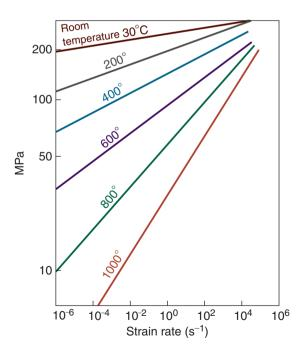
**Figure 2.7:** The effect of strain rate on the ultimate tensile strength for aluminum. Note that, as the temperature increases, the slopes of the curves increase; thus, strength becomes more and more sensitive to strain rate as temperature increases. *Source:* J.H. Hollomon.
