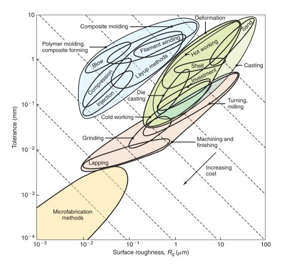
**Figure 40.5**: A plot of achievable tolerance versus surface roughness for assorted manufacturing operations. The dashed lines indicate cost factors, where an increase in precision corresponding to the separation of two neighboring lines gives an increase in cost for a given process (within a factor of two). *Source:* M.F. Ashby, *Materials Selection in Design*, Butterworth-Heinemann, 2010.
