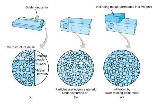
**Figure 20.15:** Three-dimensional printing using (a) part-build, (b) sinter, and (c) infiltration steps to produce metal parts. *Source:* Courtesy of Kennametal Extrude Hone.
