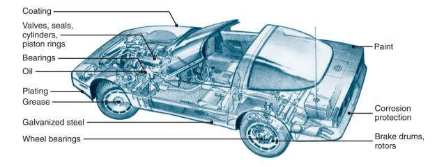
Figure VII.1: Components in a typical automobile that are related to the topics described in Part VII.
