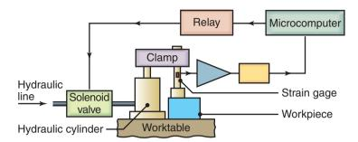
**Figure 37.28:** Schematic illustration of an adjustable-force clamping system; the clamping force is sensed by the strain gage, and the system automatically adjusts this force. *Source:* After P.K. Wright.
