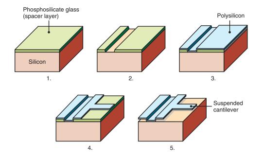
**Figure 29.3:** Schematic illustration of the steps in surface micromachining: 1. Deposition of a phosphosilicate glass (PSG) spacer layer; 2. Lithography and etching of spacer layer; 3. Deposition of polysilicon; 4. Lithography and etching of polysilicon; 5. Selective wet etching of PSG, leaving the silicon substrate and deposited polysilicon unaffected.
