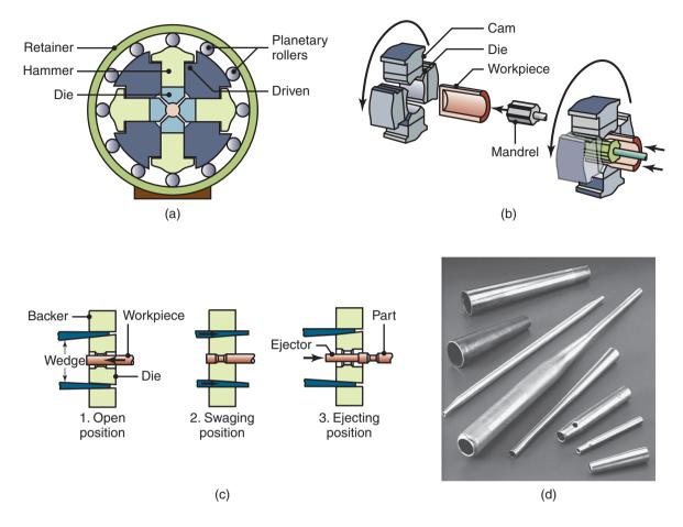
**Figure 14.15:** (a) Schematic illustration of the rotary-swaging process. (b) Forming internal profiles on a tubular workpiece by swaging. (c) A die-closing swaging machine, showing forming of a stepped shaft. (d) Typical parts made by swaging. *Source:* (d) Courtesy of Woodsage Holdings, LLC.
