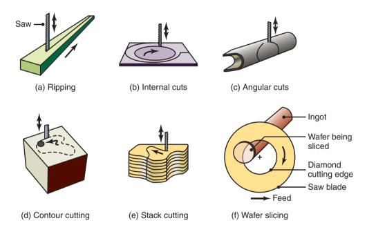
Figure 24.28: Examples of various sawing operations.
