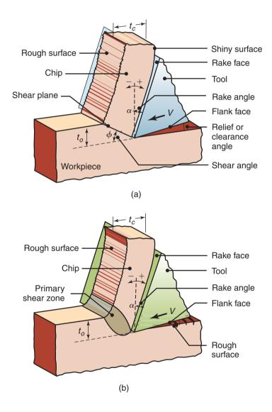
**Figure 21.3:** Schematic illustration of a two-dimensional cutting process, also called orthogonal cutting: (a) Orthogonal cutting with a well-defined shear plane, also known as the M.E. Merchant model. Note that the tool shape, the depth of cut,  $t_o$ , and the cutting speed, V, are all independent variables. (b) Orthogonal cutting without a well-defined shear plane.
