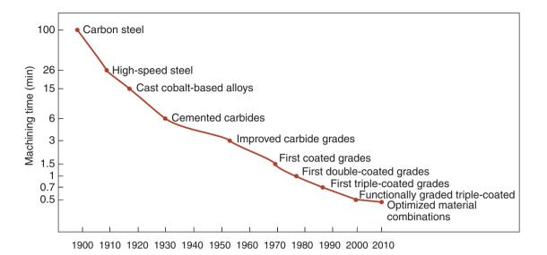
**Figure 22.6:** Relative time required to machine with various cutting-tool materials, indicating the year the tool materials were first introduced. Note that machining time has been reduced by two orders of magnitude within a hundred years. *Source:* Courtesy of Sandvik.
