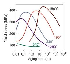
**Figure 4.20:** The effect of aging time and temperature on the yield stress of 2014-T4 aluminum alloy. Note that, for each temperature, there is an optimal aging time for maximum strength.
