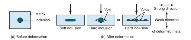
**Figure 2.24:** Schematic illustration of the deformation of soft and hard inclusions and of their effect on void formation in plastic deformation. Note that, because they do not conform to the overall deformation of the ductile matrix, hard inclusions can cause internal voids.
