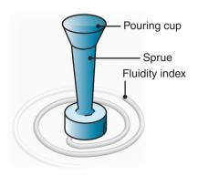
**Figure 10.11:** A test method for fluidity using a spiral mold. The fluidity index is the length of the solidified metal in the spiral passage. The greater the length of the solidified metal, the greater is the metal's fluidity.
