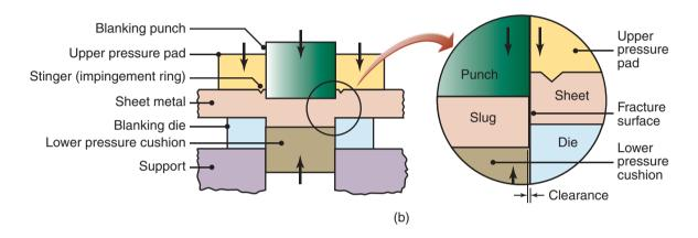
**Figure 16.5:** (a) Comparison of sheared edges produced by conventional (left) and by fine-blanking (right) techniques. (b) Schematic illustration of one setup for fine blanking. *Source:* Courtesy of Feintool U.S. Operations Inc.
