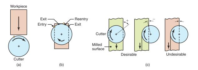
**Figure 24.11:** (a) Relative position of the cutter and insert as they first engage the workpiece in face milling. (b) Insert positions towards the end of cut. (c) Examples of exit angles of the insert, showing desirable (positive or negative angle) and undesirable (zero angle) positions. In all figures, the cutter spindle is perpendicular to the page and rotates clockwise.
