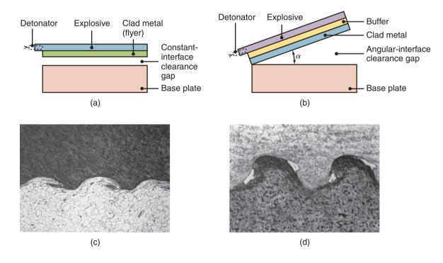
**Figure 31.16:** Schematic illustration of the explosion-welding process: (a) constant-interface clearance gap and (b) angular-interface clearance gap. (c) Cross-section of explosion-welded joint: titanium (top) and low-carbon steel (bottom). (d) Iron–nickel alloy (top) and low-carbon steel (bottom).
