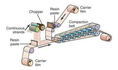
**Figure 19.23:** Schematic illustration of the manufacturing process for producing fiber-reinforced plastic sheets. The sheet still is viscous at this stage and later can be shaped into various products. *Source:* After T.-W. Chou, R.L. McCullough, and R.B. Pipes.
