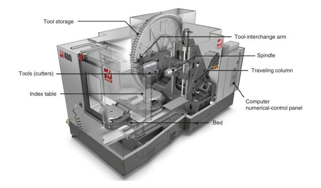
**Figure 25.2:** A horizontal-spindle machining center equipped with an automatic tool changer. Tool magazines can store up to 200 cutting tools of various functions and sizes. *Source:* Courtesy Haas Automation, Inc.
