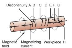
**Figure 36.10:** Schematic illustration of magnetic-particle inspection of a part with a defect in it. Cracks that are in a direction parallel to the magnetic field (such as discontinuity A) would not be detected, whereas the others shown would. Discontinuities F, G, and H are the easiest to detect. *Source:* ASM International.
