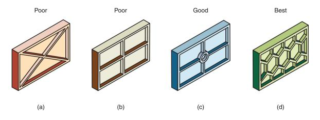
**Figure 12.3:** Rib designs for use on thin sections or flat surfaces to control or eliminate warping. Note the progression of designs: from left to right, the rib designs have improved castability and reliability.
