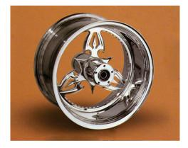
**Figure 25.1:** Examples of parts that can be machined on machining centers, using processes such as turning, facing, milling, drilling, boring, reaming, and threading. Such parts ordinarily would require the use of a variety of machine tools. Forged motorcycle wheel, finish machined to tolerance and subsequently polished and coated. *Source:* Courtesy of R.C. Components.
