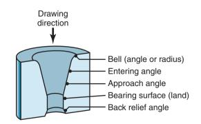
Figure 15.22: Terminology pertaining to a typical die used for drawing a round rod or wire.
