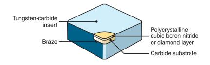
Figure 22.10: An insert of a polycrystalline cubic boron nitride or a diamond layer on tungsten carbide.
