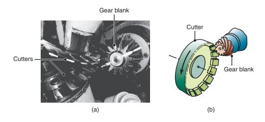
**Figure 24.35:** (a) Cutting a straight bevel-gear blank with two cutters. (b) Cutting a helical bevel gear. *Source:* Courtesy of Steve Schmid, with permission from Schafer Gear Works.
