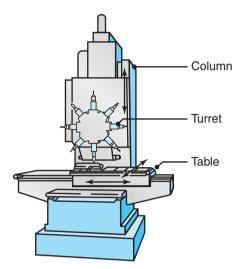
**Figure 23.26:** A three-axis computer-numerical-control drilling machine. The turret holds as many as eight different tools, such as drills, taps, and reamers.
