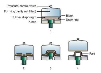
**Figure 16.42:** The hydroform (or fluid-forming) process. Note that, in contrast to the ordinary deep-drawing process, the pressure in the dome forces the cup walls against the punch. The cup travels with the punch; in this way, deep drawability is improved.
