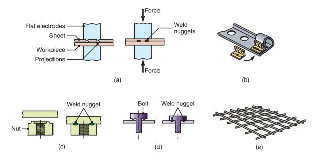
**Figure 31.12:** (a) Schematic illustration of resistance projection welding. (b) A welded bracket. (c) and (d) Projection welding of nuts or threaded bosses and studs. (e) Resistance-projection-welded grills.
