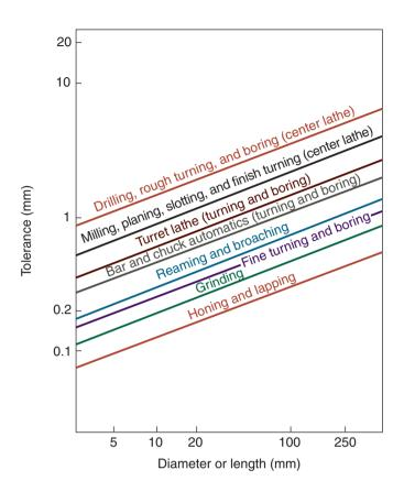
**Figure 23.15:** Range of dimensional tolerances in various machining processes as a function of workpiece size. Note that there is one order of magnitude difference between small and large workpieces.
