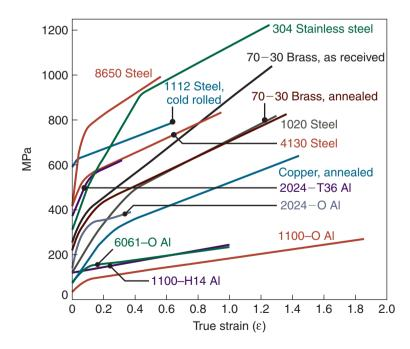
**Figure 2.5:** True stress–true strain curves in tension at room temperature for various metals. The curves start at a finite level of stress: The elastic regions have too steep a slope to be shown in this figure; thus, each curve starts at the yield strength,  $S_y$ , of the material.
