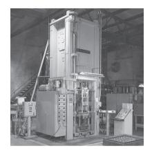
Figure 17.13: A 7.3-MN mechanical press for compacting metal powder. *Source:* Courtesy of Cincinnati Incorporated.
