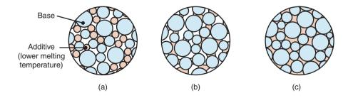
**Figure 17.23:** Schematic illustration of liquid phase sintering using a mixture of two powders. (a) Green compact of a higher melting point base metal and lower temperature additive; (b) liquid melting, wetting and reprecipitation on surfaces; (c) fully sintered solid material.
