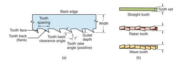
**Figure 24.29:** (a) Terminology for saw teeth. (b) Types of tooth sets on saw teeth staggered to provide clearance for the saw blade to prevent binding during sawing.
