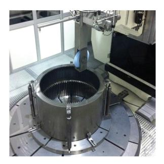
Figure 26.37: Grinding of a 3-m diameter gear.
