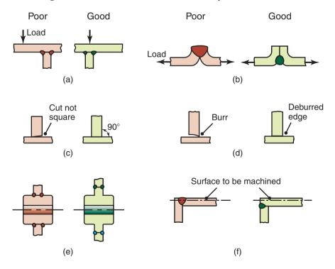
Figure 30.31: Some design guidelines for welds. *Source:* After J.G. Bralla.
