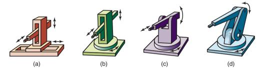
**Figure 37.20:** Four types of industrial robots: (a) Cartesian (rectilinear), (b) cylindrical, (c) spherical (polar), and (d) articulated (revolute, jointed, or anthropomorphic).
