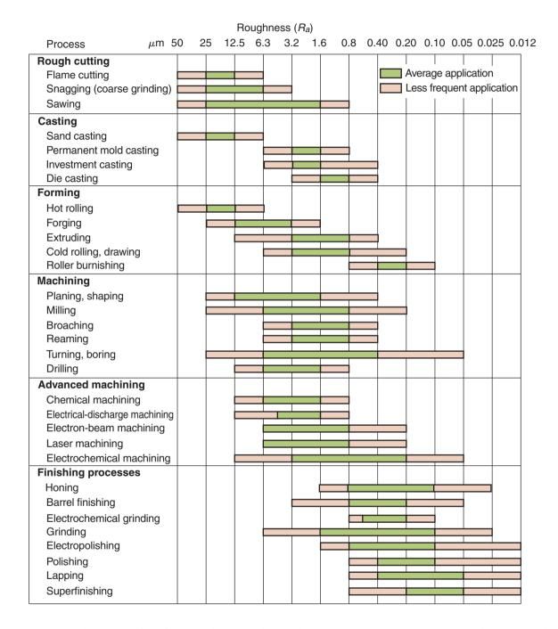
**Figure 23.14:** The range of surface roughnesses obtained in various processes; note the wide range within each group, especially in turning and boring.
