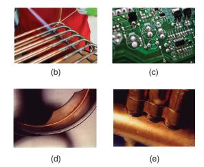
**Figure 32.1:** Examples of brazed and soldered joints. (a) Torch brazing of heat exchanger tubes; (b) a circuit board showing soldered components. *Source:* Courtesy of (a) Shutterstock/Bildagentur Zoonar GmbH; (b) Shutterstock/Chaikom.
