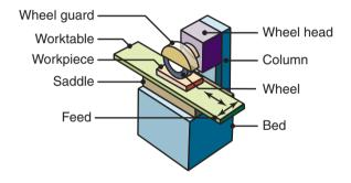
Figure 26.16: Schematic illustration of a horizontal-spindle surface grinder.
