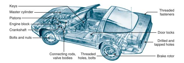
**Figure IV.4:** Typical parts on an automobile that require machining operations to impart desirable shapes, surface characteristics, dimensions, and tolerances.
