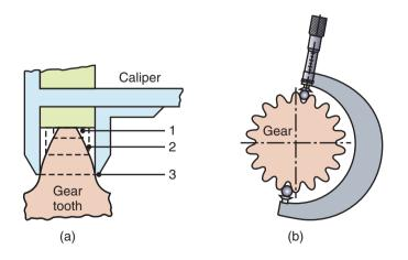
**Figure 35.9:** Measuring gear-tooth thickness and profile with (a) a gear-tooth caliper and (b) pins or balls and a micrometer.
