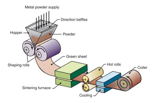
Figure 17.19: An illustration of powder rolling.
