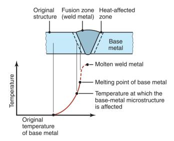
Figure 30.19: Characteristics of a typical fusion-weld zone in oxyfuel–gas and arc welding.
