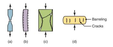
**Figure 2.20:** Schematic illustration of types of failures in materials: (a) necking and fracture of ductile materials; (b) buckling of ductile materials under a compressive load; (c) fracture of brittle materials in compression; (d) cracking on the barreled surface of ductile materials in compression.
