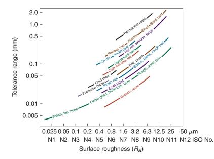
**Figure 35.21:** Dimensional tolerance range and surface roughness obtained in various manufacturing processes; these tolerances apply to a 25-mm workpiece dimension. *Source:* After J.A. Schey.
