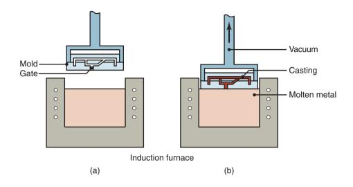
**Figure 11.17:** Schematic illustration of the vacuum-casting process. Note that the mold has a bottom gate. (a) Before and (b) after immersion of the mold into the molten metal. *Source:* After R. Blackburn.
