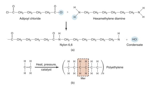
**Figure 7.3:** Examples of polymerization. (a) Condensation polymerization of nylon 6,6 and (b) addition polymerization of polyethylene molecules from ethylene mers.
