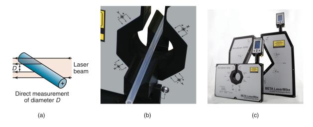
**Figure 35.15:** (a) and (b) Measurement of diameter using a laser scan micrometer; (b) Two types of laser micrometer. Such devices are available in a variety of sizes and can scan in multiple directions if needed. *Source:* (b) and (c) Courtesy of BETA Lasermike.
