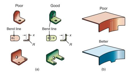
**Figure 16.63:** Stress concentrations near bends. (a) Using a crescent or ear for a hole near a bend. (b) Reducing the severity of tab in a flange. *Source:* Courtesy of Society of Manufacturing Engineers.
