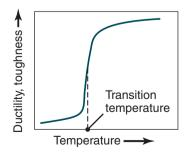
Figure 2.25: Schematic illustration of transition temperature in metals.
