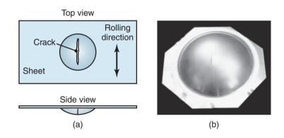
**Figure 1.13:** (a) Schematic illustration of a crack in sheet metal that has been subjected to bulging (caused, for example, by pushing a steel ball against the sheet). Note the orientation of the crack with respect to the rolling direction of the sheet; this sheet is anisotropic. (b) Aluminum sheet with a crack (vertical dark line at the center) developed in a bulge test; the rolling direction of the sheet was vertical. *Source:* After J.S. Kallend, Illinois Institute of Technology.
