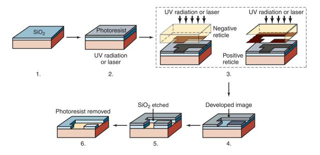
**Figure 28.13:** Pattern transfer by photolithography; note that the mask in Step 3 can be a positive or a negative image of the pattern.
