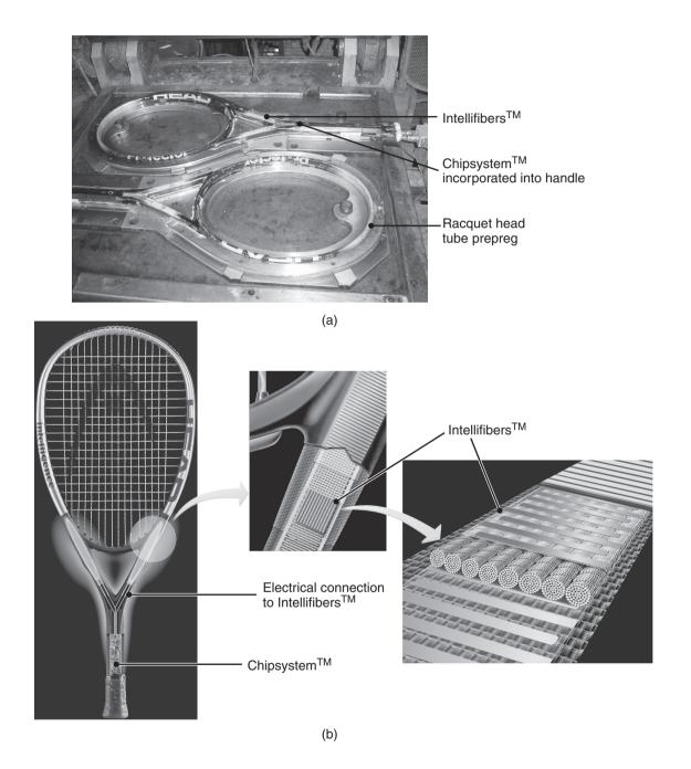
**Figure 19.29:** (a) The composite Head Protector<sup>®</sup> racquet immediately after molding; (b) a completed Head Protector<sup>®</sup> racquet, highlighting the incorporation of piezoelectric Intellifibers<sup>®</sup>. *Source:* Courtesy of Head Sport AG.
