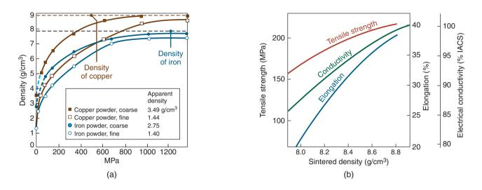
**Figure 17.11:** (a) Density of copper- and iron-powder compacts as a function of compacting pressure. Density greatly influences the mechanical and physical properties of PM parts. (b) Effect of density on tensile strength, elongation, and electrical conductivity of copper powder. *Source:* (a) After F.V. Lenel, (b) After the International Annealed Copper Standard (IACS) for electrical conductivity.
