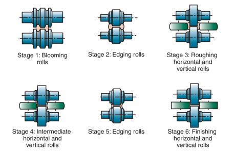
**Figure 13.13:** Steps in the shape rolling of an I-beam. Various other structural sections, such as channels and rails, also are rolled by this kind of process.
