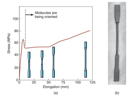
**Figure 7.13:** (a) Stress–elongation curve for polycarbonate, a thermoplastic. *Source:* Courtesy of R.P. Kambour and R.E. Robertson. (b) High-density polyethylene tensile-test specimen, showing uniform elongation (the long, narrow region in the specimen).
