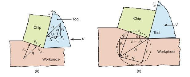
**Figure 21.11:** (a) Forces acting in the cutting zone during two-dimensional cutting. Note that the resultant force, *R*, must be colinear to balance the forces. (b) Force circle to determine various forces acting in the cutting zone.
