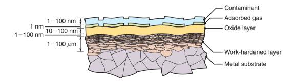
**Figure 33.1:** Schematic illustration of a cross-section of the surface structure of a metal. The thickness of the individual layers depends on both processing conditions and the processing environment. *Source:* After E. Rabinowicz and B. Bhushan.
