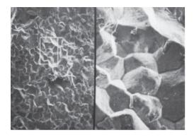
**Figure 2.27:** Intergranular fracture, at two different magnifications. Grains and grain boundaries are clearly visible in this micrograph. The fracture path is along the grain boundaries. Magnification: left,  $100 \times$ ; right,  $500 \times$ . *Source:* After B.J. Schulze and S.L. Meiley and Packer Engineering Associates, Inc.
