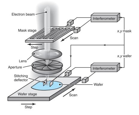
Figure 28.15: Schematic illustration of the SCALPEL process.
