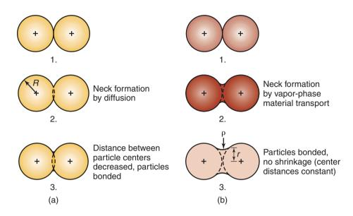
**Figure 17.22:** Schematic illustration of two mechanisms for sintering metal powders: (a) solid-state material transport; and (b) vapor-phase material transport. *R* is the particle radius, *r* is the neck radius, and  $\rho$  is the neck-profile radius.
