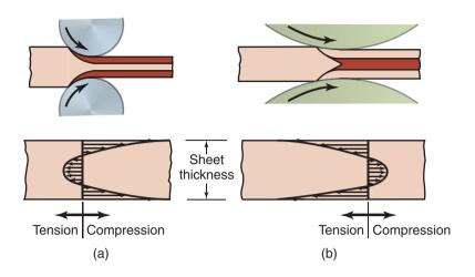
**Figure 13.10:** (a) Residual stresses developed in rolling with small-diameter rolls or at small reductions in thickness per pass. (b) Residual stresses developed in rolling with large-diameter rolls or at high reductions per pass. Note the reversal of the residual stress patterns.
