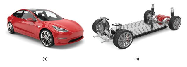
**Figure 6.3:** The Tesla S 60. (a) Image of the Tesla S 60 electric automobile, with an aluminum alloy body; (b) Chasis showing the battery supported and protected by a titanium underbody. *Source:* (a) Shutterstock/Dimitris Leonidas (b) Shutterstock/Alexander Kondratenko.
