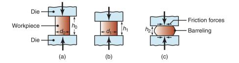
**Figure 14.3:** (a) Solid cylindrical billet upset between two flat dies. (b) Uniform deformation of the billet without friction. (c) Deformation with friction. Note barreling of the billet caused by friction forces at the billet–die interfaces.
