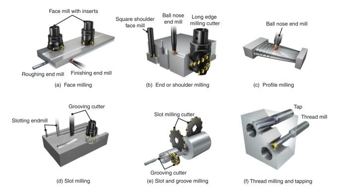
**Figure 24.2:** Some basic types of milling cutters and milling operations. (a) Face milling; (b) end or shoulder milling; (c) profile milling; (d) slot milling; (e) slot and groove milling; (f) thread milling and tapping. *Source:* Courtesy of Sandvik Coromant.
