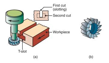
Figure 24.15: (a) T-slot cutting with a milling cutter. (b) A shell mill.
