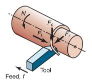
**Figure 23.5:** Forces acting on a cutting tool in turning.  $F_c$  is the cutting force,  $F_t$  is the thrust or feed force (in the direction of feed), and  $F_r$  is the radial force that tends to deflect the tool away from the workpiece being machined.
