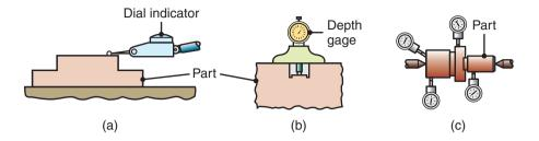
**Figure 35.5:** Three uses of dial indicators to measure (a) roundness and (b) depth, and (c) for multipledimension gaging of a part.
