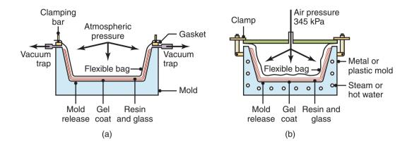
**Figure 19.24:** Schematic illustration of (a) vacuum-bag forming and (b) pressure-bag forming. These processes are used in making discrete reinforced plastic parts. *Source:* After T.H. Meister.
