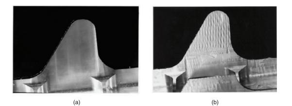
**Figure 25.13:** Chatter marks in machining. (a) smooth surface, created using the stability lobe approach to avoid chatter; (b) milling chatter marks on the surface of an Al 7075 component. Source: Courtesy Scott Smith, University of North Carolina at Charlotte.
