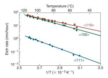
**Figure 28.20:** Etch rates of silicon in different crystallographic orientations, using ethylenediamine/pyrocatechol-in-water as the solution. *Source:* After H. Seidel.
