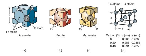
**Figure 4.7:** The unit cells for (a) austenite, (b) ferrite, and (c) martensite. The effect of percentage of carbon (by weight) on lattice dimensions for martensite is shown in (d). Note the interstitial position of the carbon atoms (see Fig. 1.8). Note also the increase in dimension *c* with increasing carbon content; this effect causes the unit cell of martensite to be in the shape of a rectangular prism.
