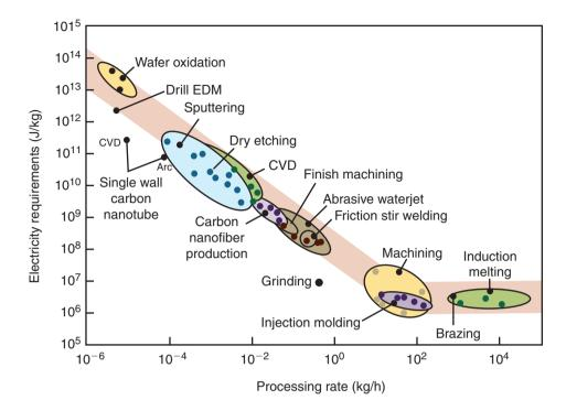
**Figure 40.1:** Specific energy requirements for various manufacturing processes, including ancillary equipment. Note that most manufacturing processes lie within the dark band. Also note the increased energy intensity for slower processes. *Source:* After T. Gutowski.
