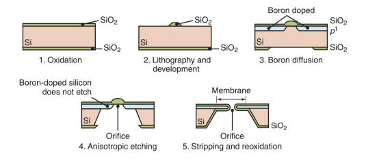
**Figure 28.21:** Application of a boron etch stop and back etching to form a membrane and orifice. *Source:* After I. Brodie and J.J. Murray.
