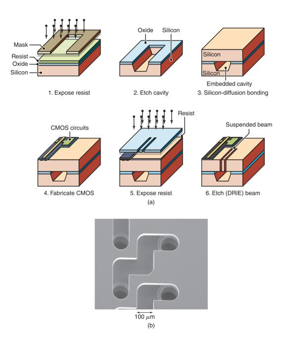
**Figure 29.14:** (a) Schematic illustration of silicon-diffusion bonding combined with deep reactive-ion etching to produce large, suspended cantilevers. (b) A microfluid-flow device manufactured by DRIE etching two separate wafers and then aligning and silicon-fusion bonding them together. Afterward, a Pyrex layer (not shown) is anodically bonded over the top to provide a window to observe fluid flow. *Source:* (a) After N. Maluf. (b) Courtesy of K.R. Williams, Agilent Technologies.
