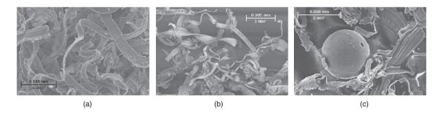
**Figure 26.12:** Typical chips, or swarf, from grinding operations. (a) Swarf from grinding a conventional HSS drill bit; (b) swarf of nickel-alloy workpiece using an  $Al_2O_3$  wheel; (c) swarf of M2 high-speed steel using an  $Al_2O_3$  wheel, showing a melted globule among the chips. *Source:* Courtesy of J. Badger, *The Grinding Doc.*
