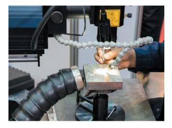
Figure 30.15: Laser beam welding in progress. *Source:* Alamy/Warut Sintapanon.
