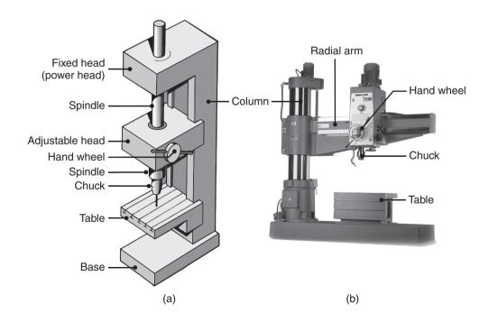
**Figure 23.25:** (a) Schematic illustration of the components of a vertical drill press. (b) A radial drilling machine. *Source:* (b) Courtesy of Willis Machinery and Tools.
