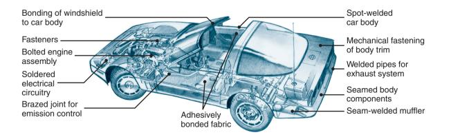
Figure VI.1: Various parts in a typical automobile that are assembled by the processes described in Part VI.
