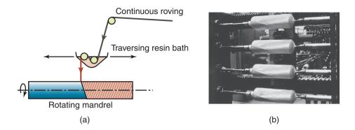
**Figure 19.26:** (a) Schematic illustration of the filament-winding process; (b) fiberglass being wound over aluminum liners for slide-raft inflation vessels for the Boeing 767 aircraft. *Source:* Courtesy of Brunswick Corporation.
