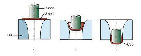
Figure 16.38: Stages in deep drawing without a blankholder, using a *tractrix* die profile.
