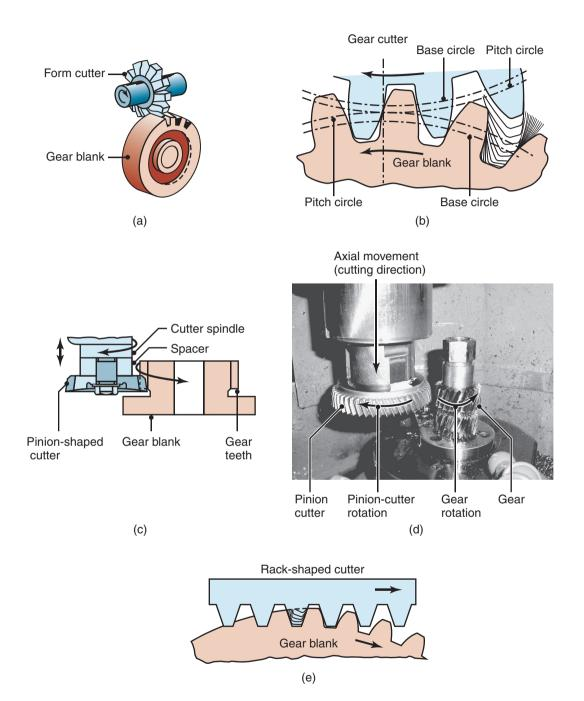
**Figure 24.33:** (a) Producing gear teeth on a blank by form cutting. (b) Schematic illustration of gear generating with a pinion-shaped gear cutter. (c) and (d) Gear generating in a gear shaper using a pinion-shaped cutter. Note that the cutter reciprocates vertically. (e) Gear generating with rack-shaped cutter. *Source:* (d) Courtesy of Steve Schmid, with permission from Schafer Gear Works.
