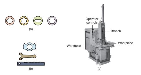
**Figure 24.23:** (a) Typical parts made by internal broaching. (b) Parts made by surface broaching. (c) Vertical broaching machine. *Source:* (a) and (b) Courtesy of General Broach and Engineering Company, (c) Courtesy of Ty Miles, Inc.
