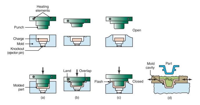
**Figure 19.17:** Types of compression molding–a process similar to forging: (a) *positive;* (b) *semipositive;* and (c) *flash,* in which the flash is later trimmed off. (d) Die design for making a compression-molded part with external undercuts.
