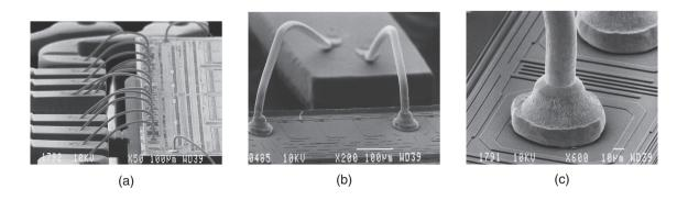
**Figure 28.30:** (a) SEM photograph of wire bonds connecting package leads (left-hand side) to die bonding pads. (b) and (c) Detailed views of (a). *Source:* Courtesy of Micron Technology, Inc.
