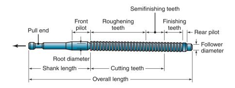
Figure 24.26: Terminology for a pull-type internal broach used for enlarging long holes.
