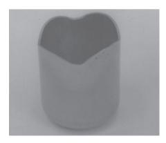
Figure 16.35: Earing in a drawn steel cup, caused by the planar anisotropy of the sheet metal.
