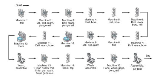
Figure 37.5: A large transfer line for producing engine blocks and cylinder heads.
