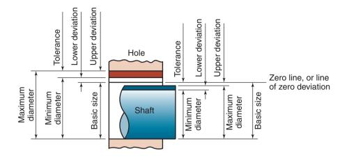
Figure 35.18: Basic size, deviation, and tolerance on a shaft, according to the ISO system.
