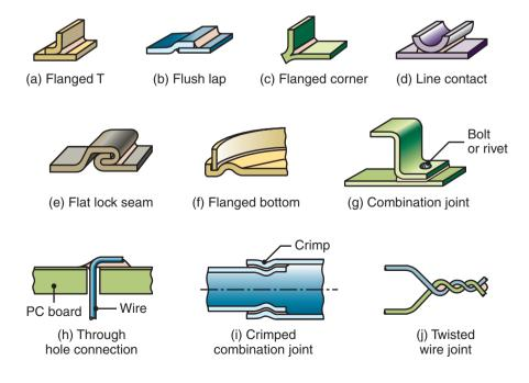
Figure 32.8: Joint designs commonly used for soldering.
