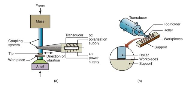
**Figure 31.2:** (a) Components of an ultrasonic-welding machine for making lap welds. The lateral vibrations of the tool tip cause plastic deformation and bonding at the interface of the workpieces. (b) Ultrasonic seam welding using a roller as the *sonotrode*.
