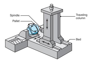
**Figure 25.3:** Schematic illustration of the principle of a five-axis machining center. The pallet, which supports and transfers the workpiece, has three axes of movement and can be swiveled around two axes (thus a total of five axes), allowing the machining of complex shapes, such as those shown in Fig. 25.1. *Source:* Courtesy of Toyoda Machinery.
