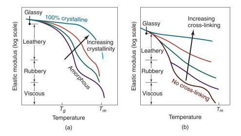
**Figure 7.6:** Behavior of polymers as a function of temperature and (a) degree of crystallinity and (b) crosslinking. The combined elastic and viscous behavior of polymers is known as viscoelasticity.
