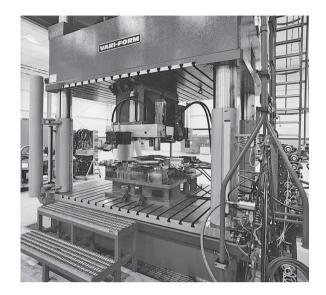
**Figure 16.47:** View of the tube-hydroforming press, with bent tube in place in the forming die. *Source:* Courtesy of B. Longhouse, Vari-Form, Inc.
