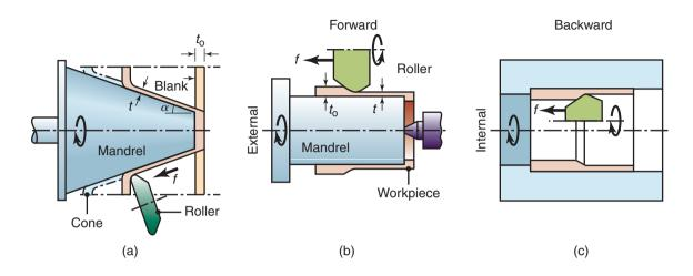
**Figure 16.49:** (a) Schematic illustration of the shear-spinning process for making conical parts. The mandrel can be shaped so that curvilinear parts can be spun. (b) and (c) Schematic illustrations of the tube-spinning process.
