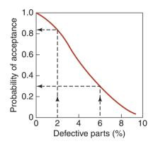
**Figure 36.8:** A typical operating-characteristics curve used in acceptance sampling. The higher the percentage of defective parts, the lower is the probability of acceptance by the consumer.
