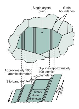
**Figure 1.7:** Schematic illustration of slip lines and slip bands in a single crystal (grain) subjected to a shear stress. A slip band consists of a number of slip planes. The crystal at the center of the upper illustration is an individual grain surrounded by several other grains.
