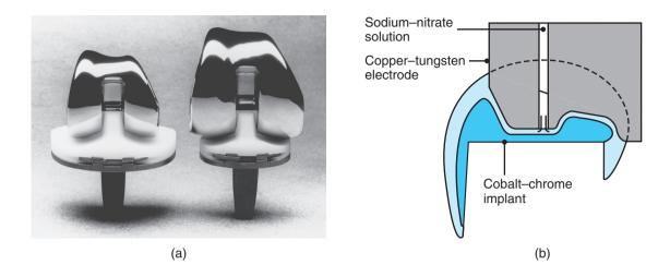
**Figure 27.7:** (a) Two total knee-replacement systems, showing metal implants (top pieces) with an ultrahighmolecular-weight polyethylene insert (bottom pieces). (b) Cross section of the ECM process, as applied to the metal implant. *Source:* Courtesy of Zimmer Biomet, Inc.
