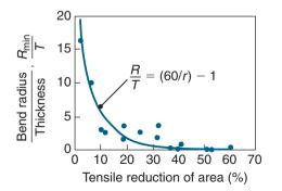
**Figure 16.18:** Relationship between  $R_{\min}/T$  and tensile reduction of area for sheet metals. Note that sheet metal with a 50% tensile reduction of area can be bent over itself in a process like the folding of a piece of paper without cracking. *Source:* After J. Datsko and C.T. Yang.
