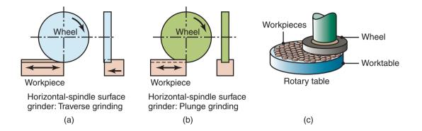
**Figure 26.15:** Schematic illustrations of various surface-grinding operations. (a) Traverse grinding with a horizontal-spindle surface grinder. (b) Plunge grinding with a horizontal-spindle surface grinder, producing a groove in the workpiece. (c) A vertical-spindle rotary-table grinder (also known as the *Blanchard* type).
