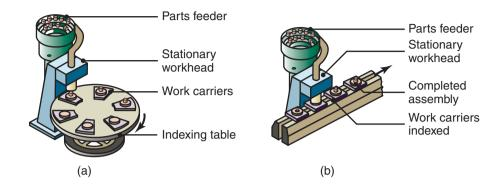
**Figure 37.30:** Transfer systems for automated assembly: (a) rotary indexing machine and (b) in-line indexing machine. *Source:* After G. Boothroyd.
