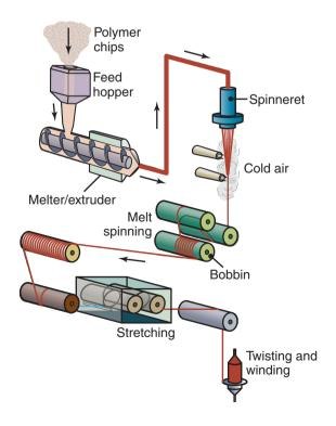
**Figure 19.6:** The melt-spinning process for producing polymer fibers. The fibers are used in a variety of applications, including reinforcements for composite materials and fabrics for clothing. In the stretching box, the right roll rotates faster than the left roll.
