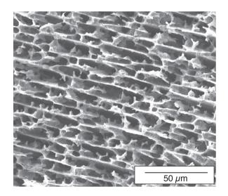
**Figure 10.9:** Microstructure after freeze casting. The specimen shown is titanium oxide (TiO<sub>2</sub>) with pure water as a freezing agent. *Source:* Courtesy S. Naleway and T. Ogden, University of Utah.
