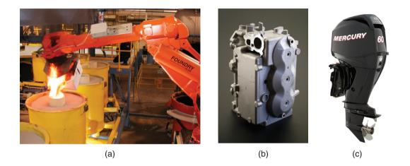
**Figure 11.13:** (a) Metal is poured into a mold for lost-foam casting of a 45-kW, three-cylinder marine engine; (b) finished engine block; (c) completed outboard motor. *Source:* Mercury Marine, a division of Brunswick Corporation.
