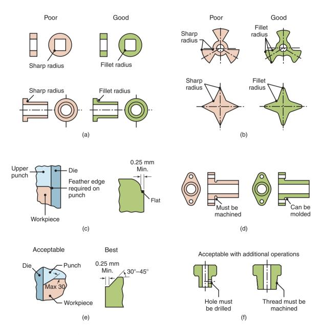
**Figure 17.26:** Examples of PM parts showing poor and good designs. Note that sharp radii and reentry corners should be avoided, and that threads and transverse holes have to be produced separately by additional machining operations. *Source:* Courtesy of the Metal Powder Industries Federation.
