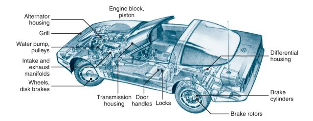
Figure II.2: Cast parts in a typical automobile.
