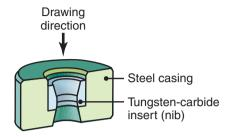
**Figure 15.23:** Tungsten-carbide die insert in a steel casing. Diamond dies used in drawing thin wire are encased in a similar manner.
