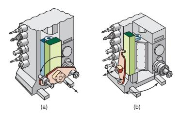
**Figure 25.5:** Swing-around tool changer on a horizontal-spindle machining center. (a) The tool-exchange arm is placing a toolholder, with a cutting tool, into the machine spindle. Note the axial and rotational movements of the arm. (b) The arm is returning to its home position. Note its rotation along a vertical axis after placing the tool, and the two degrees of freedom in its home position.
