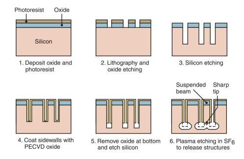
Figure 29.12: The SCREAM process. Source: After N. Maluf.
