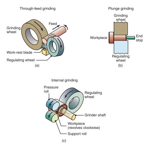
**Figure 26.24:** Schematic illustrations of centerless-grinding operations: (a) through-feed grinding, (b) plunge grinding, (c) and internal grinding.
