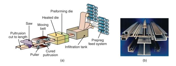
**Figure 19.27:** (a) Schematic illustration of the pultrusion process. (b) Examples of parts made by pultrusion. The major components of fiberglass ladders (used especially by electricians) are made by this process. They are available in different colors, but are heavier because of the presence of glass fibers. *Source:* Courtesy of Strongwell.
