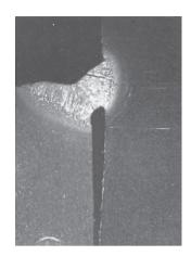
Figure 30.24: Crack in a weld bead. The two welded components were not allowed to contract freely after the weld was completed.
