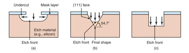
**Figure 28.19:** Etching directionality. (a) Isotropic etching: Etch proceeds vertically and horizontally at approximately the same rate, with significant mask undercut. (b) Orientation-dependent etching (ODE): Etch proceeds vertically, terminating on {111} crystal planes with little mask undercut. (c) Vertical etching: Etch proceeds vertically with little mask undercut. *Source:* After K.R. Williams, Agilent Laboratories.
