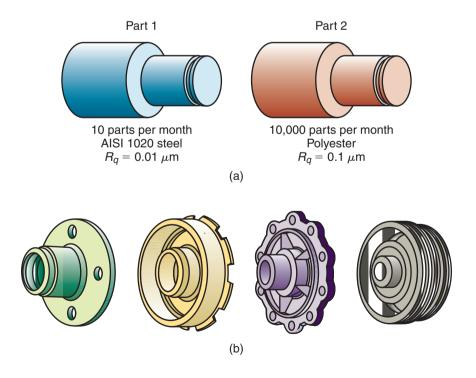
Figure 38.8: Grouping parts according to their (a) geometric similarities and (b) manufacturing attributes.
