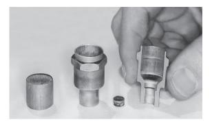
**Figure 15.12:** Production steps for the metal portion of a cold-extruded spark plug. *Source:* Courtesy of National Machinery Company, LLC.
