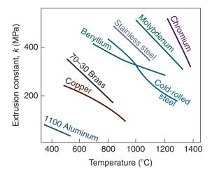
**Figure 15.5:** Extrusion constant *k* for various metals at different temperatures, as determined experimentally. *Source:* After P. Loewenstein.
