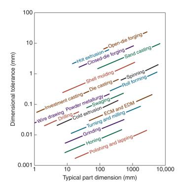
**Figure 35.20:** Dimensional tolerances as a function of part size for various manufacturing processes; note that because many factors are involved, there is a broad range for tolerances.
