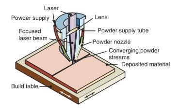
Figure 20.17: Schematic illustration of the laser-engineered net shaping (LENS) process.
