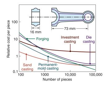
**Figure 14.22:** Relative unit costs of a small connecting rod made by various forging and casting processes. Note that, for large quantities, forging is more economical, and sand casting is the most economical process for fewer than about 20,000 pieces.
