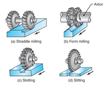
**Figure 24.14:** Cutters for (a) straddle milling, (b) form milling, (c) slotting, and (d) slitting with a milling cutter.
