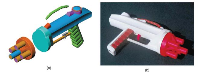
**Figure 20.2:** Additive manufacturing of a Super Soaker<sup>®</sup> squirt gun. (a) original CAD description of a toy; (b) fully functional toy produced through fused-deposition modeling. *Source:* (b) Courtesy of Rapid Models and Prototypes, Inc., and Stratasys, Inc.
