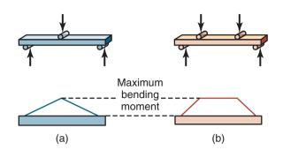
**Figure 2.11:** Two bend-test methods for brittle materials: (a) three-point bending, and (b) four-point bending. The two areas shown above the beams represent the bending-moment diagrams, described in texts on the mechanics of solids. Note the region of constant maximum bending moment in (b); by contrast, the maximum bending moment occurs only at the center of the specimen in (a).
