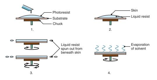
Figure 28.11: Spinning of an organic coating on a wafer.
