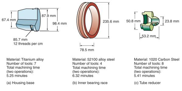
Figure 23.12: Typical parts made on CNC lathes.
