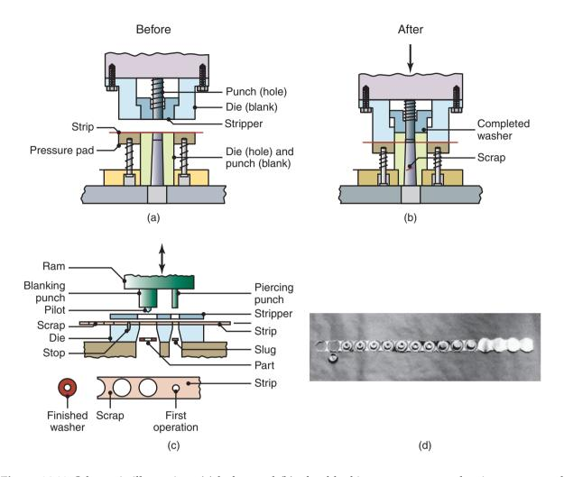
**Figure 16.11:** Schematic illustrations (a) before and (b) after blanking a common washer in a compound die. Note the separate movements of the die (for blanking) and the punch (for punching the hole in the washer). (c) Schematic illustration of making a washer in a progressive die. (d) Forming of the top piece of an aerosol spray can in a progressive die. Note that the part is attached to the strip until the last operation is completed.
