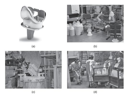
**Figure 11.15:** Manufacture of total knee replacements. (a) The Zimmer NexGen mobile-bearing knee (MBK); the femoral portion (top component) of the total knee replacement is the subject of Case Study 11.2. (b) Assembly of patterns onto a central tree. (c) Dipping of the tree into slurry to develop a mold from investment. (d) Pouring of metal into a mold. *Source:* Courtesy of M. Hawkins, Zimmer, Inc.
