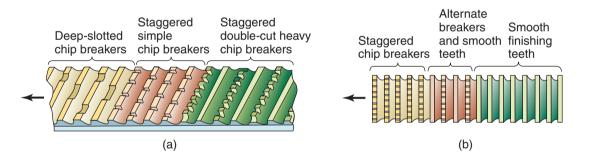
Figure 24.25: Chip breaker features on (a) a flat broach and (b) a round broach.
