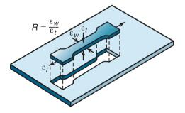
**Figure 16.33:** Strains on a tensile-test specimen removed from a piece of sheet metal. These strains are then used in determining the normal and planar anisotropy of the sheet metal.
