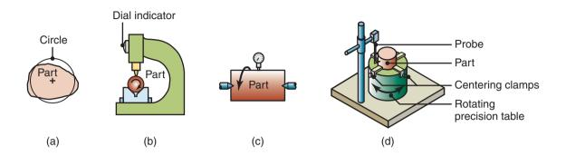
**Figure 35.8:** (a) Schematic illustration of out-of-roundness (exaggerated). Measuring roundness with (b) a V-block and dial indicator, (c) a round part supported on centers and rotated, and (d) circular tracing. *Source:* After F.T. Farago.
