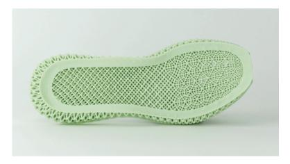
**Figure 20.10:** The use of a metamaterial shoe sole. Note that the pattern in the metamaterial changes with location to obtain a desired mechanical performance. *Source:* Courtesy of Carbon, Inc.
