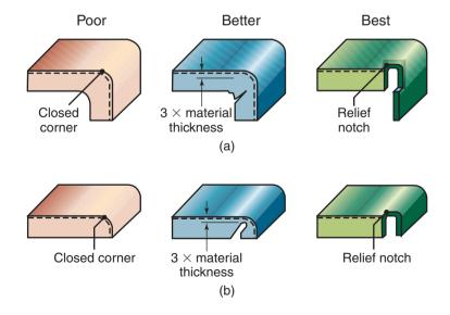
**Figure 16.61:** Control of tearing and buckling of a flange in a right-angle bend. *Source:* Courtesy of Society of Manufacturing Engineers.
