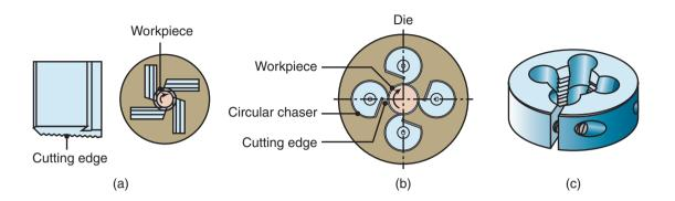
**Figure 23.17:** (a) Straight chasers for cutting threads on a lathe. (b) Circular chasers. (c) A solid threading die; the screw adjusts the gap.
