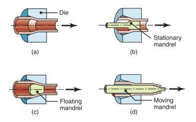
**Figure 15.21:** Examples of tube-drawing operations, with and without an internal mandrel. Note that a range of diameters and wall thicknesses can be produced from the same initial tube stock which has been made by other processes.
