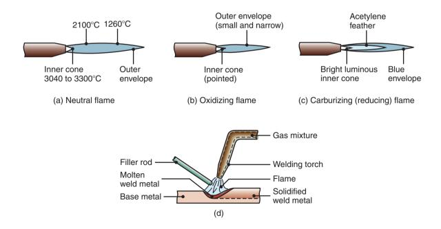
**Figure 30.1:** Three basic types of oxyacetylene flames used in oxyfuel–gas welding and cutting operations: (a) neutral flame; (b) oxidizing flame; (c) carburizing, or reducing, flame. The gas mixture in (a) is basically equal volumes of oxygen and acetylene. (d) The principle of the oxyfuel–gas welding process.
