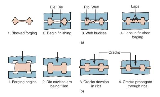
**Figure 14.17:** Examples of defects in forged parts. (a) Laps formed by web buckling during forging; web thickness should be increased to avoid this problem. (b) Internal defects caused by an oversized billet. Die cavities are filled prematurely, and the material at the center flows past the filled regions as the dies close.
