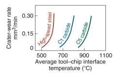
**Figure 21.19:** Relationship between crater-wear rate and average tool–chip interface temperature: (1) high-speed steel, (2) C1 carbide, and (3) C5 carbide (see Table 22.5). Note how rapidly crater-wear rate increases with an incremental increase in temperature. *Source:* After B.T. Chao and K.J. Trigger.
