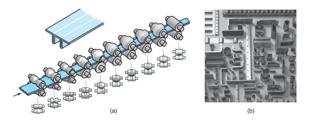
**Figure 16.26:** (a) Schematic illustration of the roll-forming process. (b) Examples of roll-formed cross sections. *Source:* (b) Courtesy of Voestalpine Roll Forming Corporation.
