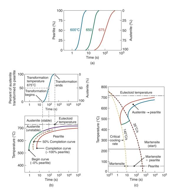
**Figure 4.15:** (a) Austenite-to-pearlite transformation of iron–carbon alloy as a function of time and temperature. (b) Isothermal transformation diagram obtained from (a) for a transformation temperature of 675°C. (c) Microstructures obtained for a eutectoid iron–carbon alloy as a function of cooling rate.
