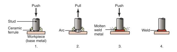
**Figure 31.14:** The sequence of operations in stud welding commonly used for welding bars, threaded rods, and various fasteners onto metal plates.
