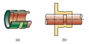
Figure 32.18: Two examples of mechanical joining by crimping.
