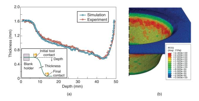
**Figure 16.51:** Finite element model of single point incremental forming. (a) Validation of the thickness profile for a funnel shape; (b) Strain distribution of a 67° cone.
