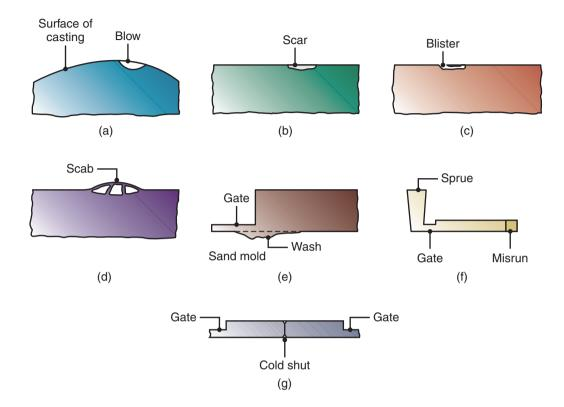
**Figure 10.15:** Examples of common defects in castings. These defects can be minimized or eliminated by proper design and preparation of molds and control of pouring procedures. *Source:* After J. Datsko.
