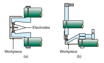
Figure 31.7: Two electrode designs for easy access to the components to be welded.
