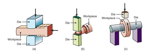
**Figure 14.4:** (a) Schematic illustration of a cogging operation on a rectangular bar. Blacksmiths use this process to reduce the thickness of bars by hammering the part on an anvil. Reduction in thickness is accompanied by barreling, as in Fig. 14.3c. (b) Reducing the diameter of a bar by open-die forging; note the movements of the dies and the workpiece. (c) The thickness of a ring being reduced by open-die forging.
