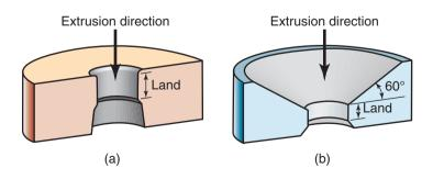
**Figure 15.7:** Typical extrusion–die configurations: (a) die for nonferrous metals; (b) die for ferrous metals; (c) die for a T-shaped extrusion, made of hot-work die steel and used with molten glass as a lubricant.
