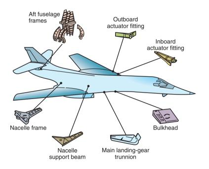
Figure 31.17: Aerospace diffusion bonding applications.
