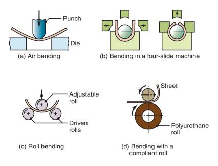
Figure 16.22: Examples of various bending operations.
