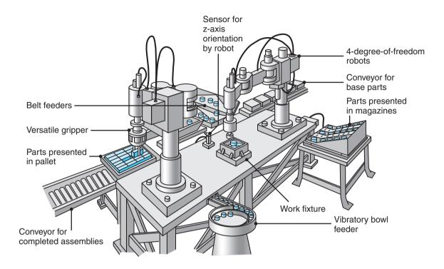
Figure 37.31: A two-arm robot assembly station. Source: After G. Boothroyd and P. Dewhurst.
