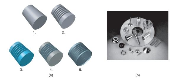
**Figure 34.10:** (a) Typical sequence in electroforming. (1) A mandrel is selected with the correct nominal size. (2) The desired geometry (in this case, that of a bellows) is machined into the mandrel. (3) The desired metal is electroplated onto the mandrel. (4) The plated material is trimmed if necessary. (5) The mandrel is dissolved through chemical machining. (b) A collection of electroformed parts. *Source:* Courtesy of Servometer<sup>(R)</sup>, Cedar Grove, NJ.
