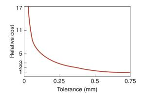
Figure 40.2: Dependence of manufacturing cost on dimensional tolerances.
