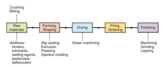
Figure 18.2: Processing steps involved in making ceramic parts.
