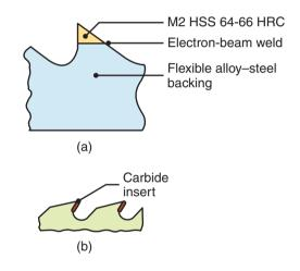
Figure 24.30: (a) High-speed-steel teeth welded onto a steel blade. (b) Carbide inserts brazed to blade teeth.
