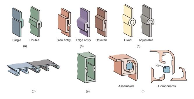
**Figure 15.18:** Examples of part geometries that allow assembly of extruded sections. (a) Lap joints; (b) laplock joints; (c) cylindrical sliding fits; (d) cylindrical sliding lock joints; (e) snap fit; (f) keyed assembly.
