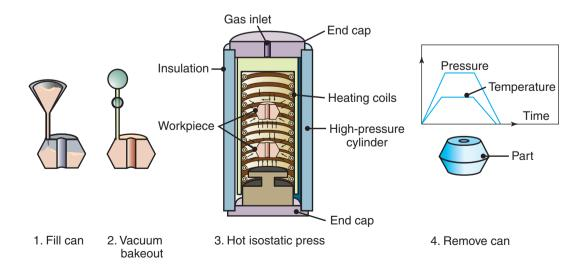
**Figure 17.16:** Schematic illustration of hot isostatic pressing. The pressure and temperature variation versus time are shown in the diagram.
