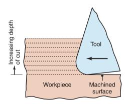
**Figure 21.22:** Schematic illustration of a dull tool with respect to the depth of cut in orthogonal machining (exaggerated). Note that the tool has a positive rake angle, but as the depth of cut decreases, the rake angle effectively can become negative. The tool then simply rides over the workpiece (without cutting) and burnishes its surface; this action raises the workpiece temperature and causes surface residual stresses.
