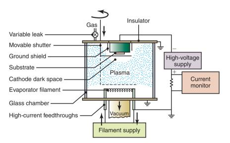
Figure 34.5: Schematic illustration of an ion-plating apparatus.
