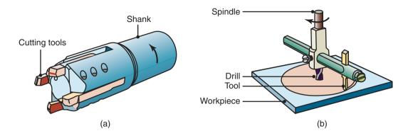
Figure 23.24: (a) Trepanning tool. (b) Trepanning with a drill-mounted single cutter.
