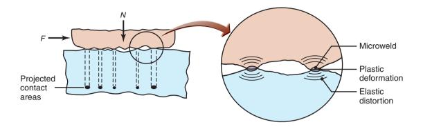
**Figure 33.6:** Schematic illustration of the interface of two bodies in contact showing real areas of contact at the asperities. In engineering surfaces, the ratio of the apparent-to-real areas of contact can be as high as 4 to 5 orders of magnitude.
