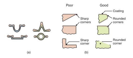
**Figure 34.9:** (a) Schematic illustration of nonuniform coatings (exaggerated) in electroplated parts. (b) Design guidelines for electroplating. Note that sharp external and internal corners should be avoided for uniform plating thickness.
