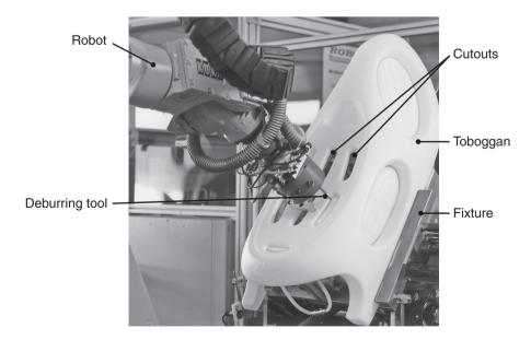
**Figure 37.24:** Robotic Deburring of a Blow-Molded Toboggan. *Source:* Courtesy of Kuka Robotics, Inc., and Roboter Technologie, GmbH. (See also Fig. 26.35.)
