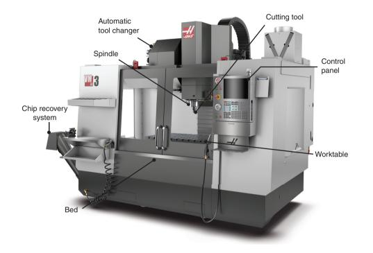
**Figure 25.7:** A vertical-spindle machining center. The tool changer is on the left of the machine, and has a 40 tool magazine. *Source:* Courtesy of Haas Automation, Inc.
