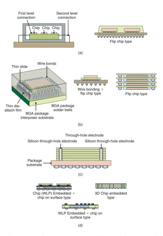
**Figure 28.34:** Major categories of system-in-package designs. (a) Horizontal placement, or multichip modules (MCMs); (b) interposer-type stacked structure; (c) interposerless stacked structure with through-silicon vias; and (d) embedded structure. WLP = wafer level package.
