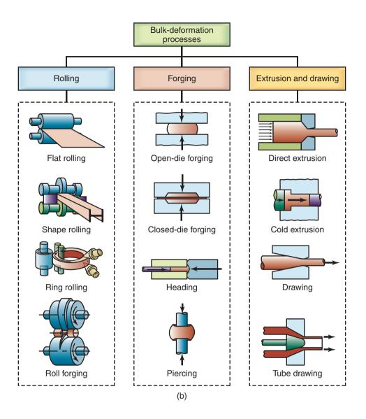
Figure I.7: (b) Schematic illustrations of various bulk-deformation processes.
