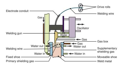
Figure 30.13: Schematic illustration of the electrogas-welding process.
