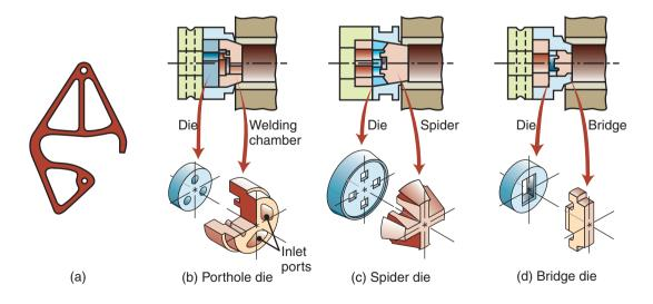
**Figure 15.9:** (a) An extruded 6063-T6 aluminum-ladder lock for aluminum extension ladders. This part is 8 mm thick and is sawed from the extrusion (see Fig. 15.2). (b) through (d) Components of various dies for extruding intricate hollow shapes. *Source:* (b) through (d) after K. Laue and H. Stenger.
