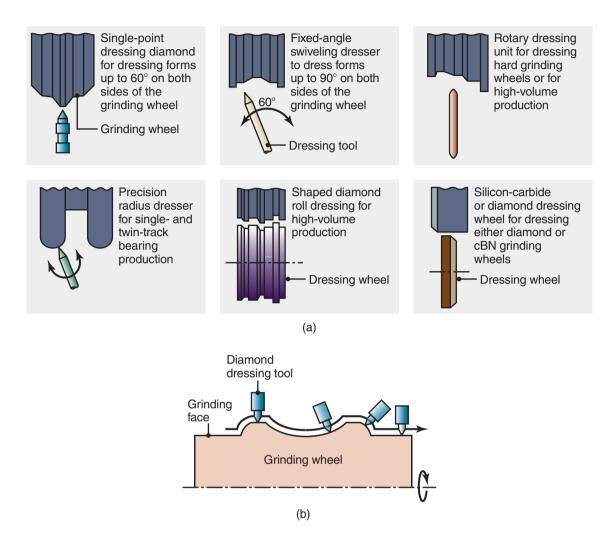
**Figure 26.14:** (a) Types of grinding-wheel dressing. (b) Shaping the grinding face of a wheel by dressing it by computer control. Note that the diamond dressing tool is normal to the surface at the point of contact with the wheel. *Source:* Courtesy of Okuma Machinery Works, Ltd.
