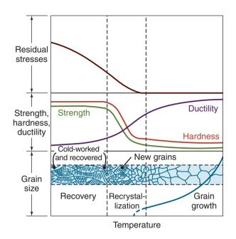
**Figure 1.14:** Schematic illustration of the effects of recovery, recrystallization, and grain growth on mechanical properties and on the shape and size of grains. Note the formation of small new grains during recrystallization. *Source:* After G. Sachs.
