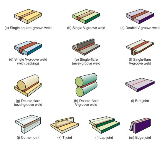
Figure 30.29: Examples of welded joints and their terminology.
