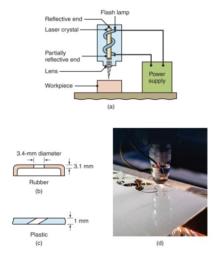
**Figure 27.12:** (a) Schematic illustration of the laser-beam machining process. (b) and (c) Examples of holes produced in nonmetallic parts by LBM. (d) Cutting sheet metal with a laser beam. *Source:* (d) Courtesy of SPI Lasers UK Ltd.
