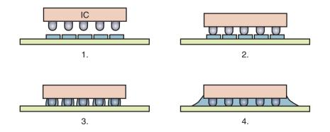
**Figure 28.33:** Illustration of flip-chip technology. Flip-chip package with 1. solder-plated metal balls and pads on the printed circuit board; 2. flux application and placement; 3. reflow soldering; 4. encapsulation.
