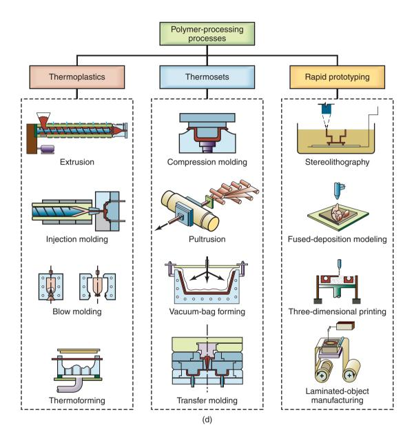
Figure I.7: (d) Schematic illustrations of various polymer-processing methods.
