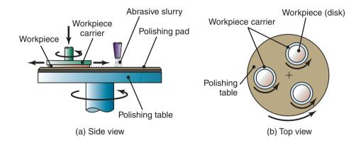
**Figure 26.32:** Schematic illustration of the chemical–mechanical polishing process. This process is used widely in making silicon wafers and integrated circuits and also is known as *chemical–mechanical pla-narization*. For other materials and applications, more carriers and more disks per carrier are possible.
