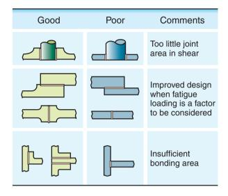
Figure 32.6: Examples of good and poor designs for brazing. Source: American Welding Society.
