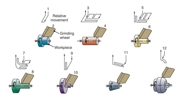
Figure 26.22: Cycle patterns for a CNC precision grinder.
