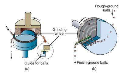
**Figure 26.17:** (a) Rough grinding of steel balls on a vertical-spindle grinder. The balls are guided by a special rotary fixture. (b) Finish grinding of balls in a multiple-groove fixture. The balls are ground to within 0.013 mm of their final size.
