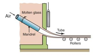
**Figure 18.9:** Manufacturing process for glass tubing. Air is blown through the mandrel to keep the tube from collapsing. Glass tubes for fluorescent bulbs are made by this method.
