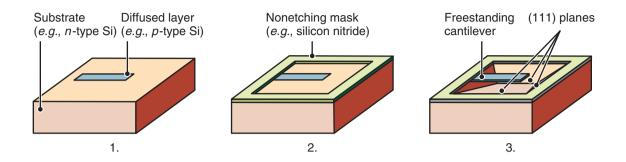
**Figure 29.2:** Schematic illustration of bulk micromachining. 1. Diffuse dopant in desired pattern. 2. Deposit a pattern and masking. 3. Orientation-dependent etching (ODE) leaves behind a freestanding structure. *Source:* Courtesy of K.R. Williams, Agilent Technologies.
