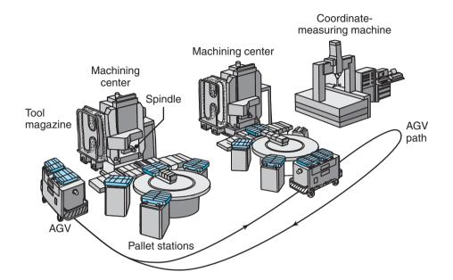
**Figure 39.2:** A schematic illustration of a flexible manufacturing system, showing two machining centers, a measuring and inspection station, and two automated guided vehicles. *Source:* After JT. Black.
