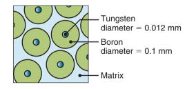
Figure 9.4: Cross section of boron fiber-reinforced composite material.
