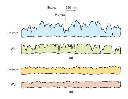
**Figure 33.9:** Changes in original (a) wire-brushed and (b) ground-surface profiles after wear. Note the difference in the vertical and horizontal scales. *Source:* After E. Wild and K.J. Mack.
