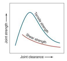
**Figure 32.4:** The effect of joint clearance on the tensile and shear strength of brazed joints. Note that, unlike tensile strength, the shear strength continually decreases as the clearance increases.
