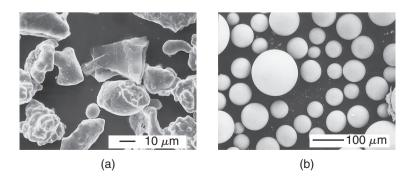
**Figure 17.4:** (a) Scanning-electron microscopy image of iron-powder particles made by atomization. (b) Nickel-based superalloy (Udimet 700) powder particles made by the rotating electrode process; see Fig. 17.5d. *Source:* After P.G. Nash, Illinois Institute of Technology, Chicago.
