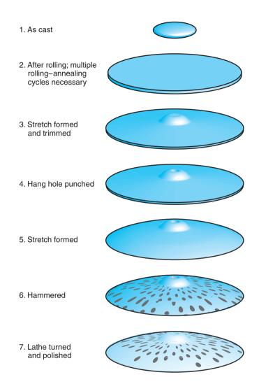
Figure 16.57: Manufacturing sequence for the production of cymbals. *Source:* Courtesy of W. Blanchard, Sabian Ltd.
