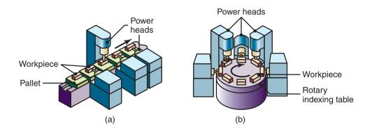
Figure 37.4: Two types of transfer mechanisms: (a) straight rails and (b) circular or rotary.
