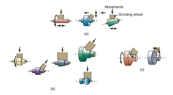
**Figure 26.18:** Examples of various cylindrical-grinding operations: (a) traverse grinding, (b) plunge grinding, and (c) profile grinding. *Source:* Courtesy of Okuma Machinery Works, Ltd.
