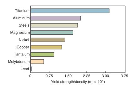
Figure 3.1: Ratio of maximum yield stress to density for selected metals.
