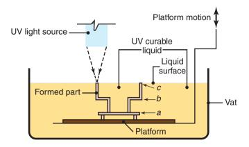
Figure 20.8: Schematic illustration of the stereolithography process.
