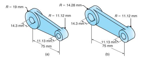
**Figure 38.6:** An example of parametric design; the dimensions of part features can be modified easily to quickly obtain an updated solid model.
