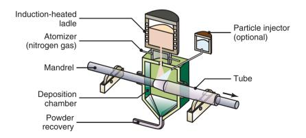
**Figure 17.20:** Spray deposition (*Osprey process*) in which molten metal is sprayed over a rotating mandrel to produce seamless tubing and pipe.
