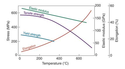
**Figure 2.6:** Effect of temperature on mechanical properties of carbon steel. Most materials display a similar temperature sensitivity for elastic modulus, yield strength, ultimate strength, and ductility.
