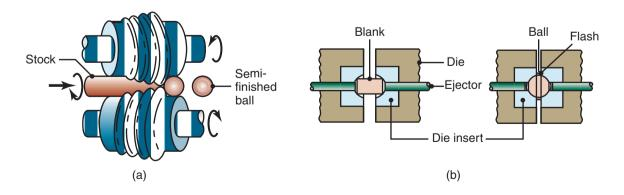
**Figure 13.15:** (a) Producing steel balls by the skew-rolling process. (b) Producing steel balls by upsetting a cylindrical blank. Note the formation of flash. The balls made by these processes are subsequently ground and polished for use in ball bearings.
