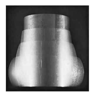
**Figure 2.8:** Barreling in compressing a round solid cylindrical specimen (7075-O aluminum) between flat dies. Barreling is caused by friction at the die–specimen interfaces, which retards the free flow of the material (see also Fig. 14.3).
