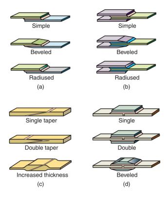
**Figure 32.12:** Desirable configurations for adhesively bonded joints: (a) single lap, (b) double lap, (c) scarf, and (d) strap.
