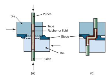
**Figure 16.28:** A method of forming a tube with sharp angles, using an axial compressive force. Note that the tube is supported internally with rubber or fluid to avoid collapsing during forming. *Source:* After J.L. Remmerswaal and A. Verkaik.
