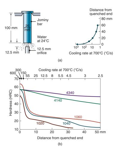
**Figure 4.18:** (a) End-quench test and cooling rate. (b) Hardenability curves for five different steels, as obtained from the end-quench test. Small variations in composition can change the shape of these curves. Each curve is actually a band, and its exact determination is important in the heat treatment of metals, for better control of properties.
