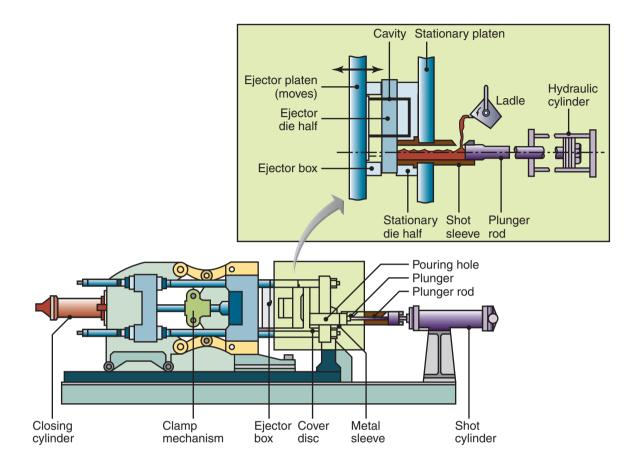
**Figure 11.19:** Schematic illustration of the cold-chamber die-casting process. These machines are large as compared to the size of the casting, because high forces are required to keep the two halves of the dies closed under pressure.
