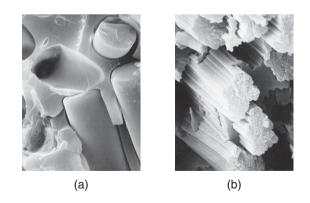
**Figure 9.6:** (a) Fracture surface of a glass fiber-reinforced epoxy composite. The fibers are 10  $\mu$ m in diameter and have random orientation. (b) Fracture surface of a graphite fiber-reinforced epoxy composite. The fibers, 9 to 11  $\mu$ m in diameter, are in bundles and are all aligned in the same direction. *Source:* After L.J. Broutman.
