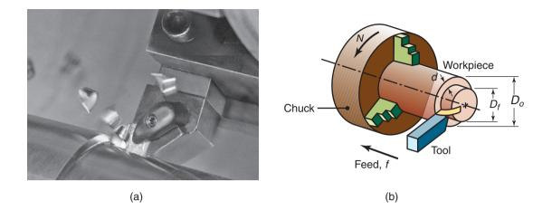
**Figure 23.3:** (a) Photograph of a turning operation, showing insert and discontinuous chips. The cutting tool is traveling from right to left in this photograph. (b) Schematic illustration of the basic turning operation, showing depth of cut, *d*; feed, *f*; and spindle rotational speed, *N*, in rev/min. The cutting speed is the surface speed of the workpiece at the tool tip. *Source:* (a) Courtesy of Kennametal Inc.
