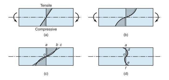
**Figure 2.30:** Residual stresses developed in bending a beam having a rectangular cross section. Note that the horizontal forces and moments caused by residual stresses in the beam must be balanced internally. Because of nonuniform deformation, especially during cold-metalworking operations, most parts develop residual stresses.
