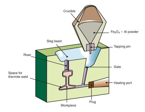
Figure 30.4: Schematic illustration of thermite welding.
