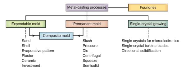
Figure II.3: Outline of metal-casting processes described in Part II.
