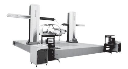
**Figure 35.17:** A large coordinate-measuring machine with two heads measuring various dimensions on a car body.
