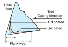
**Figure 22.7:** Schematic illustration of typical wear patterns on uncoated high-speed steel tools and titaniumnitride-coated tools. Note that flank wear is significantly lower for the coated tool.
