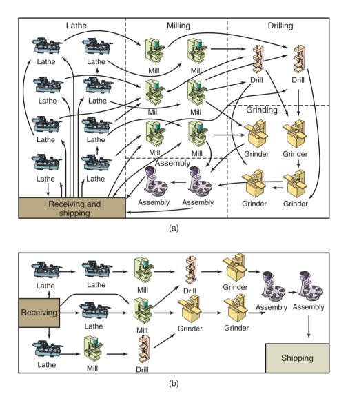
**Figure 38.9:** (a) Functional layout of machine tools in a traditional plant; arrows indicate the flow of materials and parts in various stages of completion. (b) Group-technology (cellular) layout. Legend: L = lathe, M = milling machine, D = drilling machine, G = grinding machine, A = assembly. *Source:* After M.P. Groover.
