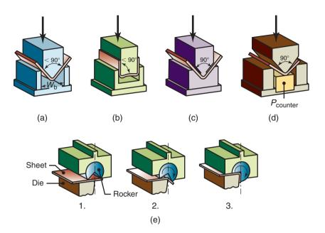
Figure 16.20: Methods of reducing or compensating for springback in bending operations.
