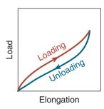
**Figure 7.14:** Typical load–elongation curve for rubbers. The clockwise loop, indicating the loading and the unloading paths, displays the *hysteresis loss*. Hysteresis gives rubbers their capacity to dissipate energy, damp vibration, and absorb shock loading, as is necessary in automobile tires and in vibration dampers placed under machinery.
