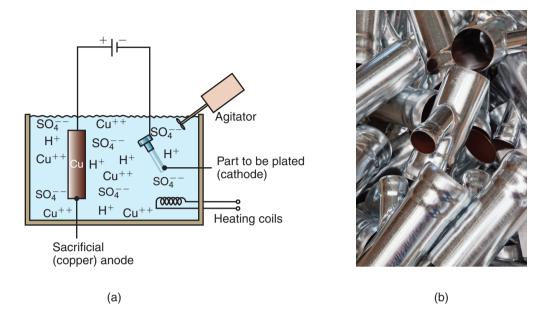
**Figure 34.8:** (a) Schematic illustration of the electroplating process. (b) Examples of electroplated parts. *Source:* Courtesy of Shutterstock/Jarous.
