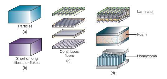
**Figure 9.2:** Schematic illustration of methods of reinforcing plastics (matrix) with (a) particles, (b) short or long fibers or flakes, and (c) continuous fibers. The laminate structures shown in (d) can be produced from layers of continuous fibers or sandwich structures using a foam or honeycomb core (see also Fig. 16.59).
