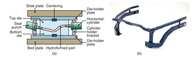
**Figure 16.43:** (a) Schematic illustration of the tube-hydroforming process. (b) A vehicle body assembly module made up of seven hydroformed tubes. *Source:* Courtesy Vari-Form, Inc.
