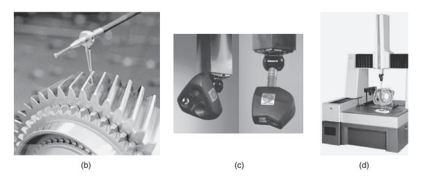
**Figure 35.16:** (a) Schematic illustration of a coordinate-measuring machine. (b) A touch signal probe. (c) Examples of laser probes. (d) A coordinate-measuring machine with a complex part being measured. *Source:* (b) through (d) Courtesy of Mitutoyo America Corp.
