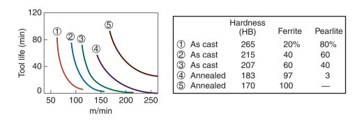
**Figure 21.16:** Effect of workpiece hardness and microstructure on tool life in turning ductile cast iron. Note the rapid decrease in tool life (approaching zero) as the cutting speed increases. Tool materials have been developed that resist high temperatures, such as carbides, ceramics, and cubic boron nitride, as described in Chapter 22.
