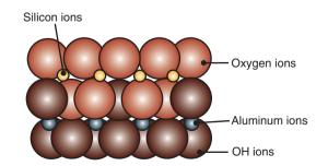
Figure 8.2: The crystal structure of kaolinite, commonly known as clay; compare with Figs. 1.3–1.5 for metals.
