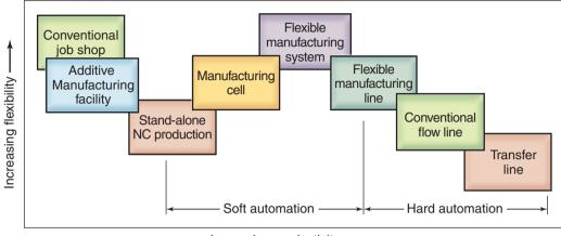
**Figure 37.2:** Flexibility and productivity of various manufacturing systems. Note the overlap between the systems, due to the various levels of automation and computer control that are possible in each group. (See Chapter 39 for details.)
