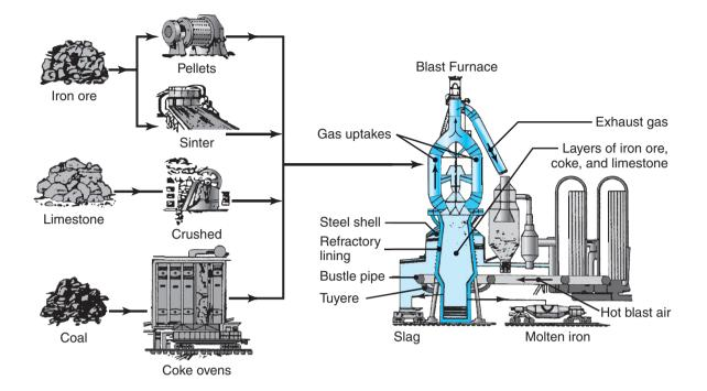
Figure 5.1: Schematic illustration of a blast furnace.
