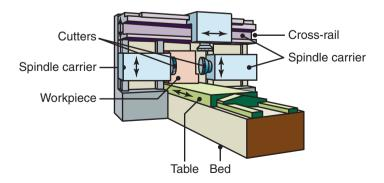
Figure 24.19: Schematic illustration of a bed-type milling machine.
