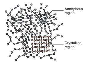
**Figure 7.8:** Amorphous and crystalline regions in a polymer. The crystalline region (crystallite) has an orderly arrangement of molecules. The higher the crystallinity, the harder, stiffer, and less ductile the polymer.
