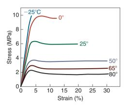
**Figure 7.11:** Effect of temperature on the stress–strain curve for cellulose acetate, a thermoplastic. Note the large drop in strength and the large increase in ductility with a relatively small increase in temperature. *Source:* After T.S. Carswell and H.K. Nason.
