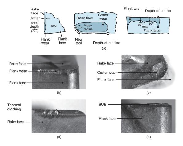
**Figure 21.15:** (a) Features of tool wear in a turning operation. The VB indicates average flank wear. (b)–(e) Examples of wear in cutting tools: (b) flank wear, (c) crater wear, (d) thermal cracking, and (e) flank wear and built-up edge. *Source:* (a) Terms and definitions reproduced with the permission of the International Organization for Standardization, ISO, copyright remains with ISO. (b)–(e) Courtesy of Kennametal Inc.
