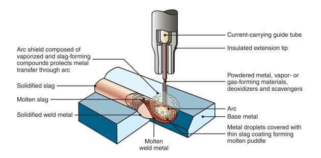
**Figure 30.12:** Schematic illustration of the flux-cored arc-welding process. This operation is similar to gas metal-arc welding, shown in Fig. 30.11.
