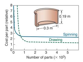
**Figure 16.66:** Cost comparison for manufacturing a round sheet-metal container either by conventional spinning or by deep drawing. Note that for small quantities, spinning is more economical.
