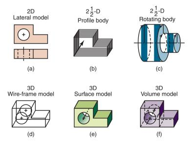
Figure 38.2: Various types of modeling for CAD.
