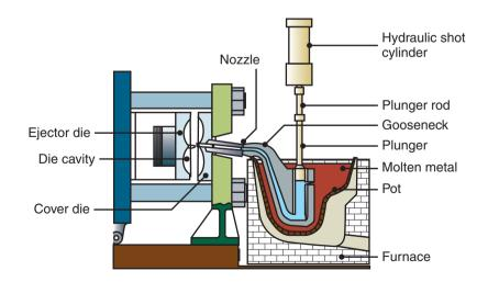
Figure 11.18: Schematic illustration of the hot-chamber die-casting process.
