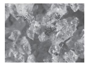
**Figure 26.10:** The surface of a grinding wheel (A46-J8V), showing abrasive grains, wheel porosity, wear flats on grains, and metal chips from the workpiece adhering to the grains. Note the random distribution and shape of the abrasive grains. Magnification:  $50 \times .$  *Source:* S. Kalpakjian.
