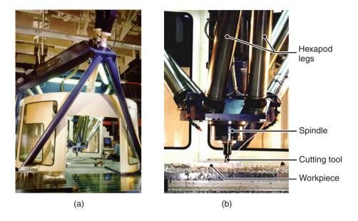
**Figure 25.12:** (a) A hexapod machine tool, showing its major components. (b) A detailed view of the cutting tool in a hexapod machining center. *Source:* National Institute of Standards and Technology.
