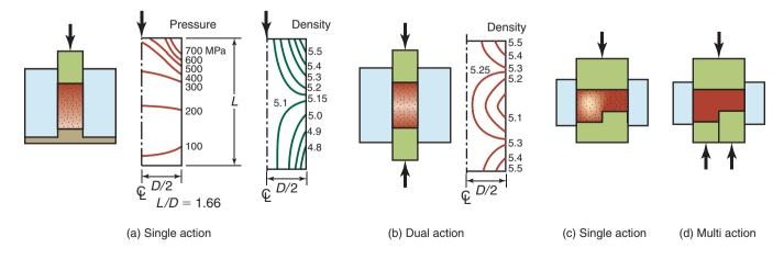
**Figure 17.12:** Density variation in compacting metal powders in various dies. *Source:* After P. Duwez and L. Zwell.
