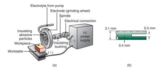
**Figure 27.8:** (a) Schematic illustration of the electrochemical-grinding process. (b) Thin slot produced on a round nickel-alloy (Inconel) tube by this process.
