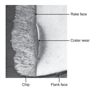
**Figure 21.20:** Interface of a cutting tool (right) and chip (left) in machining plain-carbon steel. The discoloration of the tool indicates the presence of high temperatures. Compare this figure with the temperature profiles shown in Fig. 21.12. *Source:* After P.K. Wright.
