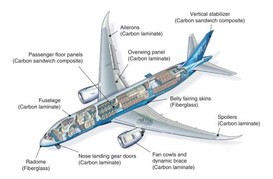
**Figure 9.1:** Application of advanced composite materials in the Boeing 787-D (Dreamliner), which is 50% composite material by weight. The reinforcement type is shown. *Source:* Graphic image Courtesy of FlightGlobal.
