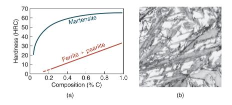
**Figure 4.13:** (a) Hardness of martensite as a function of carbon content. (b) Micrograph of martensite containing 0.8% carbon. The gray platelike regions are martensite; they have the same composition as the original austenite (white regions). Magnification:  $1000 \times$ .
