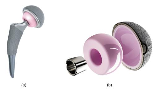
**Figure 8.1:** (a) A ceramic total hip replacement. (b) Detail of the ceramic ball and cup produced from a zirconia-alumina blend. Ceramics perform well in such applications because of their high hardness and wear resistance. *Source:* Courtesy of DePuy, a Johnson & Johnson Company.
