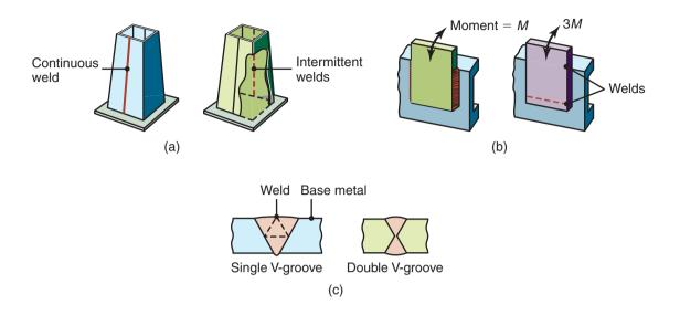
Figure 30.32: Examples of weld designs used in Example 30.3.
