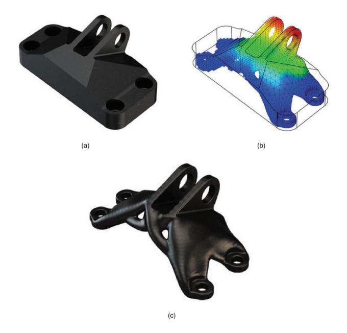
**Figure 20.23:** Topology optimization to reduce the weight of a bracket. (a) Original bracket design; (b) predicted minimum-weight bracket from topology optimization software; and (c) final bracket, representing a 70% weight loss from the original design, as produced through selective laser sintering. *Source:* 3D Systems.
