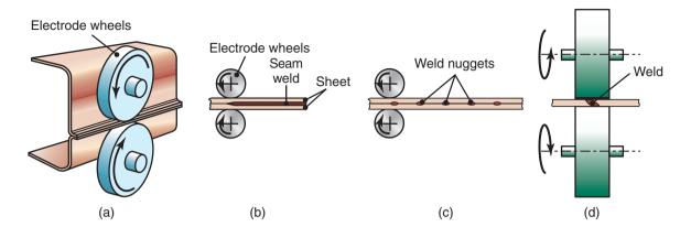
**Figure 31.10:** (a) Seam-welding process in which rotating rolls act as electrodes. (b) Overlapping spots in a seam weld. (c) Roll spot welds and (d) Mash seam welding.
