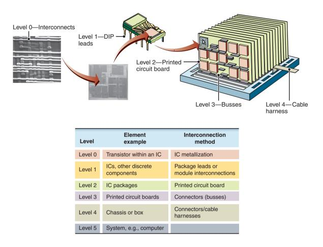
Figure 28.27: Connections between elements in the hierarchy for integrated circuits.
