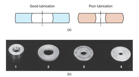
**Figure 33.7:** Ring-compression test between flat dies. (a) Effect of lubrication on type of ring-specimen barreling. (b) Test results: (1) original specimen and (2) to (4) increasing friction. *Source:* After A.T. Male and M.G. Cockcroft.
