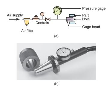
**Figure 35.12:** (a) Schematic illustration of the principle of an air gage. (b) A conical head for air gaging; note the three small airholes on the conical surface. *Source:* (b) Courtesy of Stotz Gaging Co.
