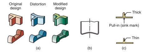
**Figure 19.30:** Examples of design modifications to eliminate or minimize distortion in plastic parts: (a) suggested design changes to minimize distortion, (b) stiffening the bottoms of thin plastic containers by doming (a technique similar to the process used to shape the bottoms of aluminum beverage cans, see Fig. 16.31), and (c) design change in a rib to minimize pull-in (*sink mark*), caused by shrinkage during the cooling of thick sections in molded parts.
