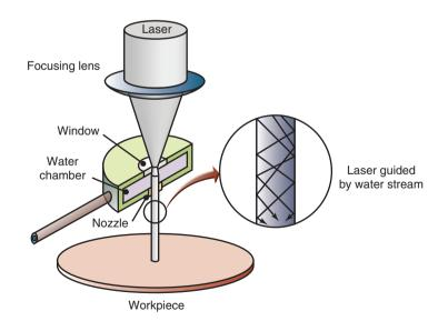
Figure 27.13: Schematic illustration of the laser microjet<sup>®</sup> process.
