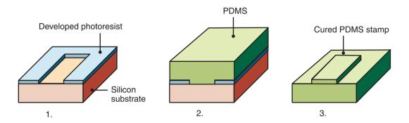
**Figure 28.17:** Production of a polydimethylsiloxane (PDMS) mold for soft lithography. 1. A developed photoresist is produced through standard lithography (Fig. 28.13). 2. A PDMS stamp is cast over the photoresist. 3. The PDMS stamp is peeled off the substrate to produce a stamp. The stamp shown has been rotated to emphasize the replication of surface features; the master pattern can be used several times. *Source:* After Y. Xia and G.M. Whitesides.
