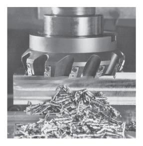
Figure 24.7: A face-milling cutter with indexable inserts. *Source:* Courtesy of Ingersoll Cutting Tool Company.
