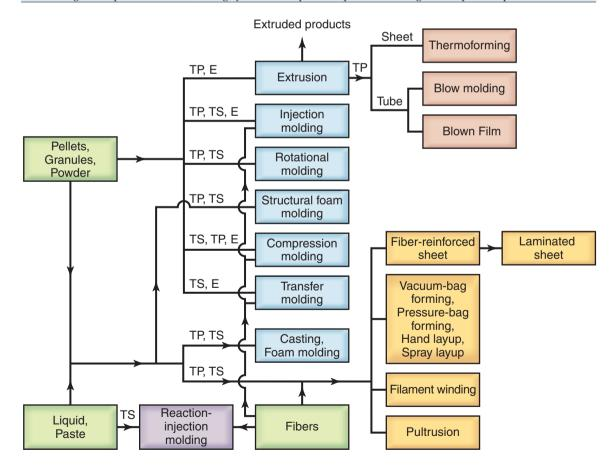
**Figure 19.1:** Outline of forming and shaping processes for plastics, elastomers, and composite materials. (TP = Thermoplastic; TS = Thermoset; E = Elastomer.)
