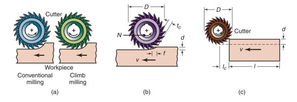
**Figure 24.5:** (a) Schematic illustration of conventional milling and climb milling. (b) Slab-milling operation showing depth of cut, d; feed per tooth, f; chip depth of cut,  $t_c$ , and workpiece speed, v. (c) Schematic illustration of cutter travel distance,  $l_c$ , to reach full depth of cut.
