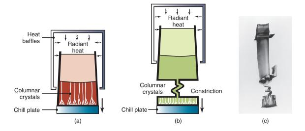
**Figure 11.25:** Methods of casting turbine blades: (a) directional solidification; (b) method to produce a single-crystal blade; (c) a single-crystal blade with the constriction portion still attached (see also Fig. 1.1). *Source:* (a) and (b) After B.H. Kear, (c) Courtesy of ASM International.
