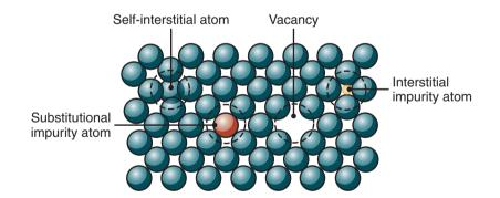
**Figure 1.8:** Schematic illustration of types of defects in a single-crystal lattice: self-interstitial, vacancy, interstitial, and substitutional.
