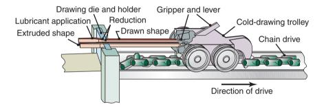
**Figure 15.24:** Cold drawing of an extruded channel on a draw bench to reduce its cross section. Individual lengths of straight rods or of cross sections are drawn by this method.
