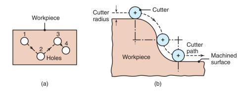
**Figure 37.10:** Movement of tools in numerical-control machining. (a) Point-to-point, in which the drill bit drills a hole at position 1, is retracted and moved to position 2, and so on. (b) Continuous path by a milling cutter. Note that the cutter path is compensated for by the cutter radius; the path also can be compensated for cutter wear.
