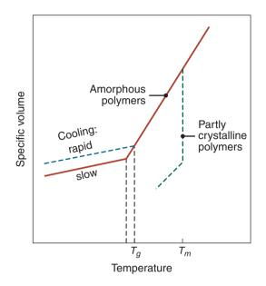
**Figure 7.9:** Specific volume of polymers as a function of temperature. Amorphous polymers, such as acrylic and polycarbonate, have a glass-transition temperature, but do not have a specific melting point. Partly crystalline polymers, such as polyethylene and nylons, contract sharply while passing through their melting temperatures during cooling.
