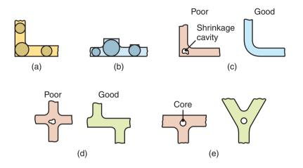
**Figure 12.2:** Examples of designs showing the importance of maintaining uniform cross sections in castings to avoid hot spots and shrinkage cavities. (a) Illustration of the method of inscribing the largest possible circle in a cross section; locations where abrupt changes in circle size occurs are concerns for hot spots and shrinkage pores. (b)–(e) Common geometries and strategies for reducing or eliminating pores.
