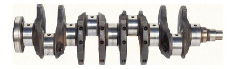
**Figure IV.1:** A forged crankshaft, highlighting the smooth and shiny machined and ground bearing surfaces. The shiny bearing surfaces cannot be made to their final dimensions and surface finish by any of the processes described in previous chapters. *Source:* Shutterstock/AleksandrN
