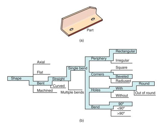
Figure 38.10: Decision-tree classification for a sheet-metal bracket. Source: After G.W. Millar.
