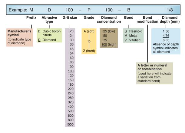
Figure 26.8: Standard marking system for cubic boron nitride and diamond bonded abrasives.
