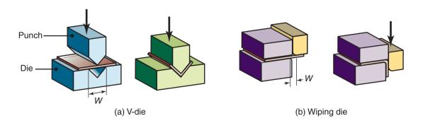
**Figure 16.21:** Common die-bending operations showing the die-opening dimension, *W*, used in calculating bending forces.
