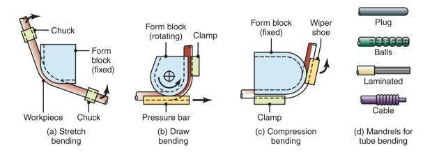
**Figure 16.27:** Methods of bending tubes. Internal mandrels or filling of tubes with particulate materials, such as sand, are often necessary to prevent collapse of the tubes during bending. Tubes also can be bent by a technique in which a stiff, helical tension spring is slipped over the tube. The clearance between the outer diameter of the tube and the inner diameter of the spring is small; thus, the tube cannot kink and the bend is uniform.
