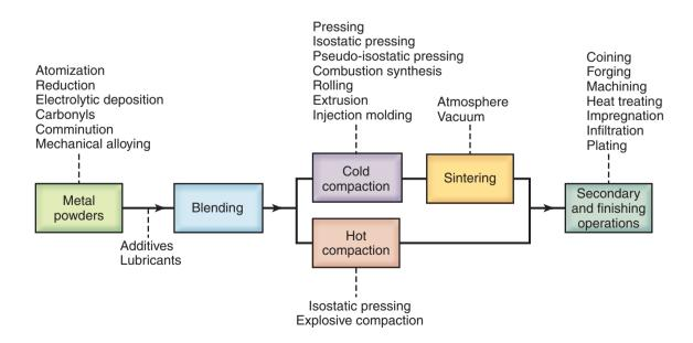
Figure 17.2: Outline of processes and operations involved in producing powder-metallurgy parts.
