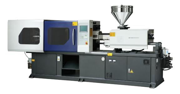
**Figure 19.12:** A 2.2-MN (225-metric ton) injection-molding machine. The tonnage is the force applied to keep the dies closed during the injection of molten plastic into the mold cavities and hold it there until the parts are cool and stiff enough to be removed from the die. *Source:* Shutterstock/Value ho
