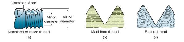
**Figure 13.18:** (a) Features of a machined or rolled thread. Grain flow in (b) machined and (c) rolled threads. Unlike machining, which cuts through the grains of the metal, the rolling of threads imparts improved strength because of cold working and favorable grain flow.
