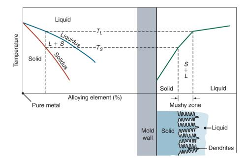
**Figure 10.4:** Schematic illustration of alloy solidification and temperature distribution in the solidifying metal. Note the formation of dendrites in the mushy zone.
