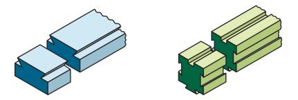
Figure 24.22: Typical parts that can be made on a planer.
