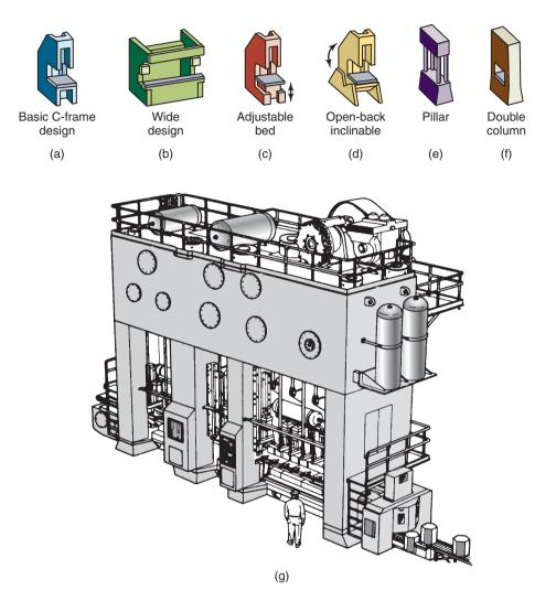
**Figure 16.65:** (a) through (f) Schematic illustrations of types of press frames for sheet-metal forming operations. Each type has its own characteristics of stiffness, capacity, and accessibility. (g) A large stamping press. *Source:* (g) Verson Allsteel Company.
