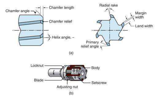
Figure 23.27: (a) Terminology for a helical reamer. (b) Inserted-blade adjustable reamer.
