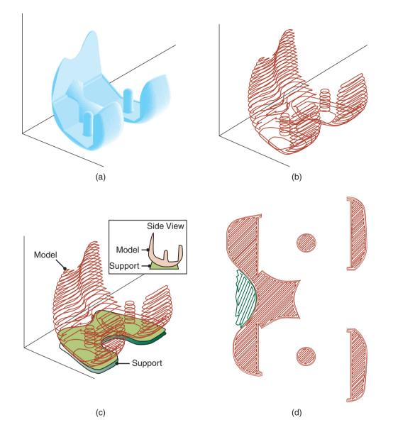
**Figure 20.3:** The computational steps in producing a stereolithography (STL) file. (a) Three-dimensional description of part. (b) The part is divided into slices; only 1 in 10 is shown. (c) Support material is planned. (d) A set of tool directions is determined to manufacture each slice. Also shown is the extruder path at section A–A from (c) for a fused-deposition-modeling operation.
