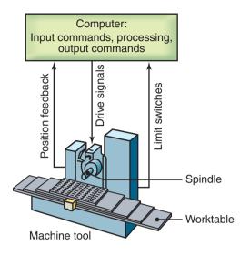
**Figure 37.7:** Schematic illustration of the major components for position control on a numerical-control machine tool.
