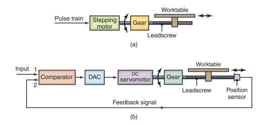
**Figure 37.8:** Schematic illustration of the components of (a) an open-loop and (b) a closed-loop control system for a numerical-control machine. DAC = digital-to-analog converter.
