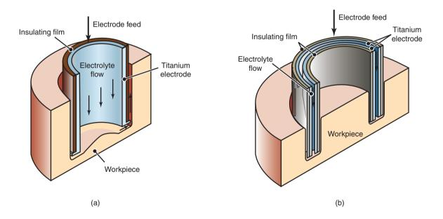
**Figure 27.6:** Shaped electrolytic machining operations. (a) Shaped-tube electrolytic machining, used to make small holes with aspect ratios as large as 300:1; (b) electrolytic trepanning, used for larger diameter holes.
