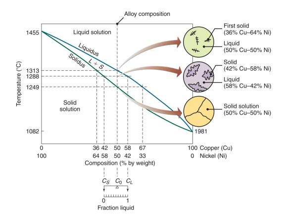
**Figure 4.4:** Phase diagram for nickel–copper alloy system obtained at a slow rate of solidification. Note that pure nickel and pure copper each have a specific freezing or melting temperature. The top circle on the right depicts the nucleation of crystals; the second circle shows the formation of dendrites (see Section 10.2.2). The bottom circle shows the solidified alloy, with grain boundaries.
