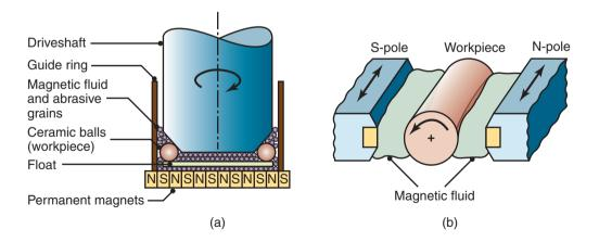
**Figure 26.33:** Schematic illustration of polishing of balls and rollers by magnetic fields. (a) Magnetic-float polishing of ceramic balls. (b) Magnetic-field-assisted polishing of rollers. *Source:* After R. Komanduri, M. Doc, and M. Fox.
