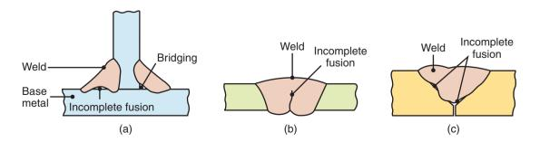
Figure 30.21: Examples of various discontinuities in fusion welds.
