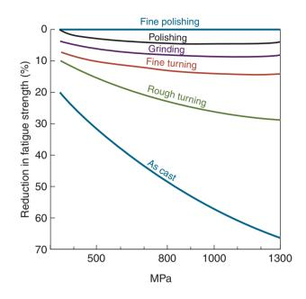
**Figure 2.29:** Reductions in the fatigue strength of cast steels subjected to various surface-finishing operations. Note that the reduction becomes greater as the surface roughness and the strength of the steel increase. *Source:* M.R. Mitchell.
