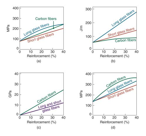
**Figure 9.5:** The effect of the type of fiber on various properties of fiber-reinforced nylon (6,6). *Source:* Courtesy of NASA.
