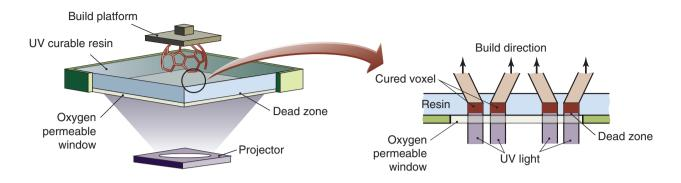
**Figure 20.9**: The CLIP process. An array of micro mirrors directs light to cure a layer, but the photopolymer next to the oxygen-permeable window does not cure because oxygen is a curing inhibitor. The cured polymer can be pulled out of the liquid photopolymer, with liquid photopolymer flowing into the interface to replenish the build layer.
