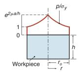
**Figure 14.5:** Distribution of die pressure in upsetting with sliding friction. Note that the pressure at the outer radius is equal to the flow stress,  $\sigma_f$ , of the material. Sliding friction means that the frictional stress is directly proportional to the normal stress.
