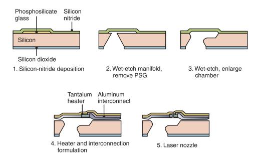
**Figure 29.16:** The manufacturing sequence for producing thermal ink-jet printer heads. *Source:* After F.-G. Tseng
