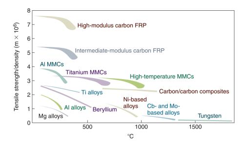
**Figure 3.3:** Specific strength (tensile strength/density) for a variety of materials as a function of temperature. Note the useful temperature range for these materials and the high values for composite materials. MMC = metal-matrix composite; FRP = fiber-reinforced plastic.
