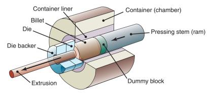
Figure 15.1: Schematic illustration of the direct extrusion process.
