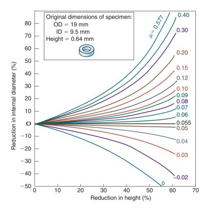
**Figure 33.8:** Chart to determine friction coefficient from a ring-compression test. Reduction in height and change in internal diameter of the ring are measured; then  $\mu$  is read directly from this chart. For example, if the ring specimen is reduced in height by 40% and its internal diameter decreases by 10%, the coefficient of friction is 0.10.
