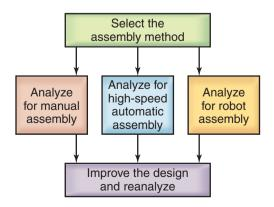
Figure 37.29: Stages in the design for assembly analysis. Source: After G. Boothroyd and P. Dewhurst.
