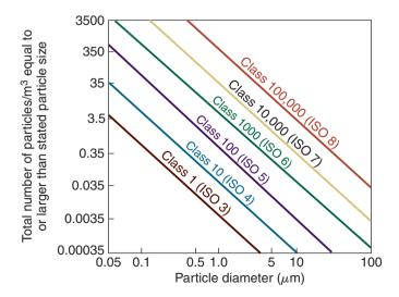
Figure 28.4: Allowable particle size counts for various clean-room classes.
