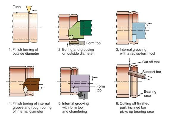
Figure 25.9: Machining of outer bearing races.
