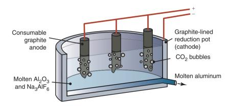
**Figure 6.2:** Schematic illustration of a Hall-Héroult reduction pot, used to produce molten aluminum from aluminum oxide.
