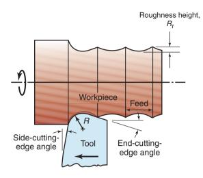
Figure 21.23: Schematic illustration of feed marks on a surface being turned (exaggerated).
