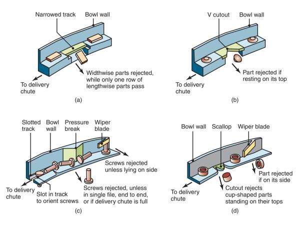
**Figure 37.32:** Examples of guides to ensure that parts are properly oriented for automated assembly. *Source:* After G. Boothroyd.
