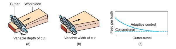
**Figure 37.14:** An example of adaptive control in milling. As the depth of cut (a) or the width of cut (b) increases, the cutting forces and the torque increase. The system senses this increase and automatically reduces the feed (c) to avoid excessive forces or tool breakage in order to maintain cutting efficiency. *Source:* After Y. Koren.
