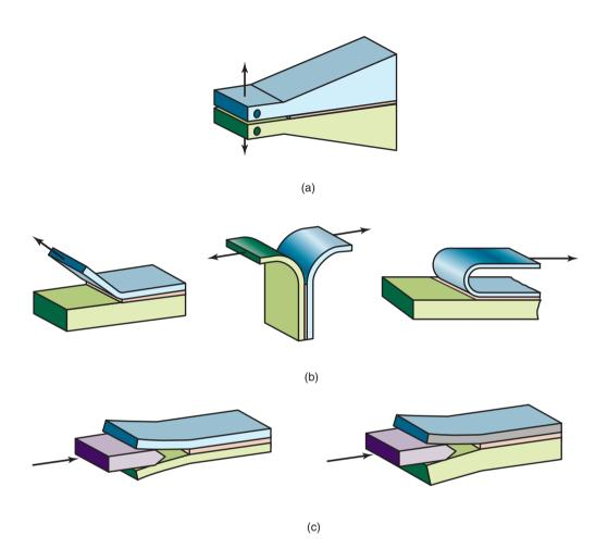
**Figure 32.9:** Common arrangements for evaluating adhesives: (a) tapered double cantilever beam, (b) peel tests and (c) wedge tests.
