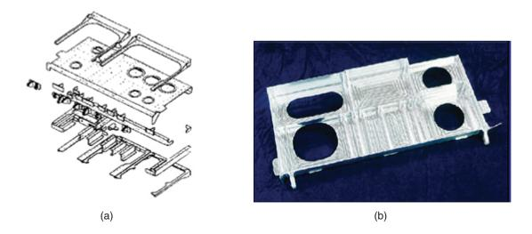
**Figure 24.39:** Production of avionics tray by (a) riveting of multiple stamped parts, and (b) machining from a monolithic block of aluminum.
