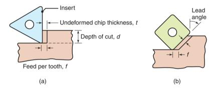
**Figure 24.10:** The effect of the lead angle on the undeformed chip thickness, *t* in face milling. Note that as the lead angle increases, the chip thickness decreases, but the length of contact (i.e., chip width) increases. The edges of the insert must be sufficiently large to accommodate the contact length increase.
