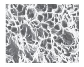
**Figure 2.22:** Surface of ductile fracture in low-carbon steel, showing dimples. Fracture is usually initiated at impurities, inclusions, or preexisting voids (microporosity) in the metal. *Source:* After K.-H. Habig and D. Klaffke.
