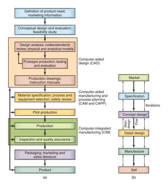
**Figure I.4:** (a) Chart showing various steps involved in *traditional* design and manufacture of a product. Depending on the complexity of the product and the type of materials used, the time span between the original concept and the marketing of the product may range from a few months to several years. (b) Chart showing general product flow in *concurrent engineering*, from market analysis to marketing the product. *Source:* After S. Pugh.
