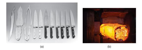
**Figure 14.1:** (a) Illustration of the steps involved in forging a knife. (b) Open die forging of a steel billet. *Source:* (a) Courtesy of Mundial, Inc. (b) Shutterstock/Milos Zvicer.
