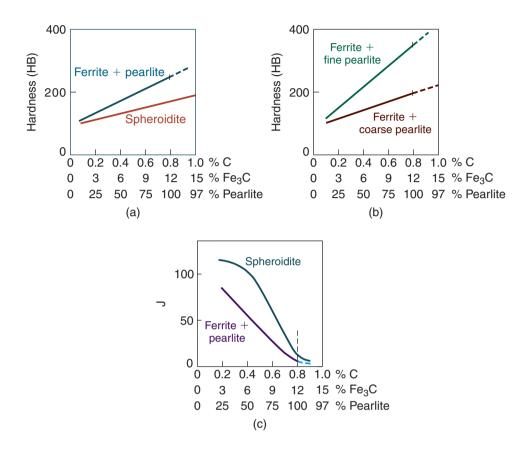
**Figure 4.16:** (a) and (b) Hardness and (c) toughness for annealed plain-carbon steels as a function of carbide shape. Carbides in the pearlite are lamellar. Fine pearlite is obtained by increasing the cooling rate. The spheroidite structure has sphere-like carbide particles.
