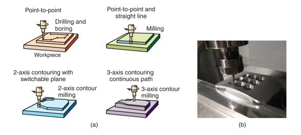
**Figure 37.12:** (a) Schematic illustration of drilling, boring, and milling along various paths. (b) Machining a sculptured surface on a 5-axis numerical-control machine. *Source:* Courtesy of Scott Smith and Geoff Heacock UNC –Charlotte.
