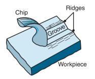
Figure 26.13: Chip formation and plowing of the workpiece surface by an abrasive grain.
