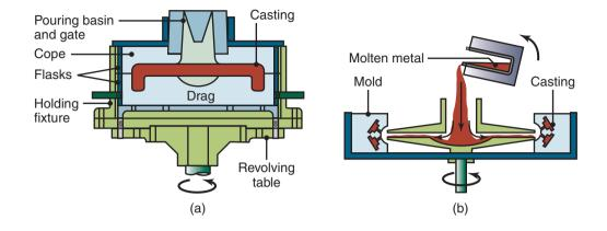
**Figure 11.23:** (a) Schematic illustration of the semicentrifugal casting process. Wheels with spokes can be cast by this process. (b) Schematic illustration of casting by centrifuging. The molds are placed at the periphery of the machine, and the molten metal is forced into the molds by centrifugal force.
