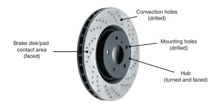
Figure 23.7: Brake disk, used in Case Study 23.1. Source: Courtesy of Kennametal, Inc.
