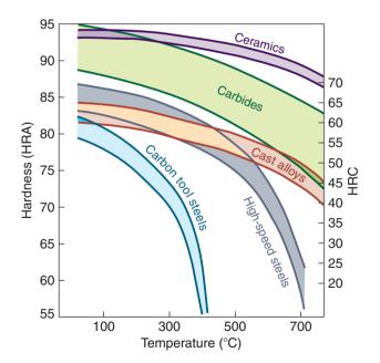
**Figure 22.1:** The hardness of various cutting-tool materials as a function of temperature. The wide range in each group of materials is due to the variety of tool compositions and treatments available for that particular group.
