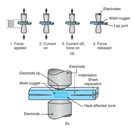
**Figure 31.6:** (a) Sequence of events in resistance spot welding of a lap joint. (b) Cross-section of a spot weld, showing the weld nugget and the indentation of the electrode on sheet surfaces. This is one of the most commonly used processes in sheet-metal fabrication and in automotive metal-body assembly.
