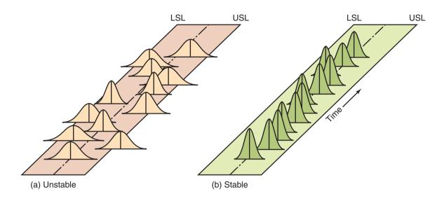
**Figure 36.7:** Illustration of processes that are (a) unstable or out of control and (b) stable or in control. Note in part (b) that all distributions standard deviations that are lower than those of the distributions in part (a) and have means closer to the desired value. *Source:* After K. Crow.
