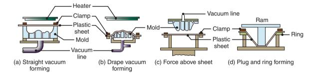
**Figure 19.16:** Various thermoforming processes for a thermoplastic sheet. These processes are commonly used in making advertising signs, cookie and candy trays, panels for shower stalls, and packaging.
