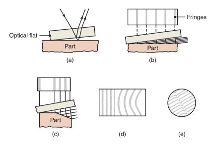
**Figure 35.7:** (a) Interferometry method for measuring flatness with an optical flat. (b) Fringes on a flat, inclined surface. An optical flat resting on a flat workpiece surface will not split the light beam, and no fringes will be present. (c) Fringes on a surface with two inclinations. Note that the greater the incline, the closer together are the fringes. (d) Curved fringe patterns, indicating curvatures on the workpiece surface. (e) Fringe pattern indicating a scratch on the surface.
