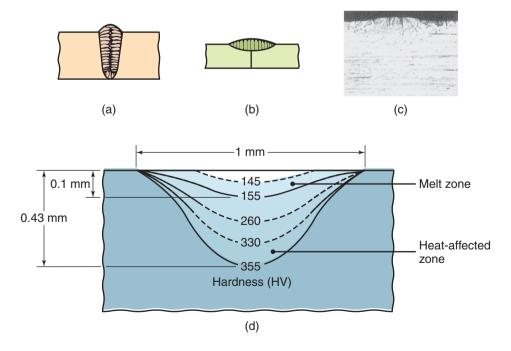
**Figure 30.20:** Grain structure in (a) a deep weld and (b) a shallow weld. Note that the grains in the solidified weld metal are perpendicular to their interface with the base metal. (c) Weld bead on a cold-rolled nickel strip produced by a laser beam. (d) Microhardness (HV) profile across a weld bead.
