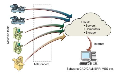
**Figure 39.4:** Schematic illustration of the use of cloud computing to capture manufacturing data and make it available wherever needed. A critical technology for cloud computing remains data security.
