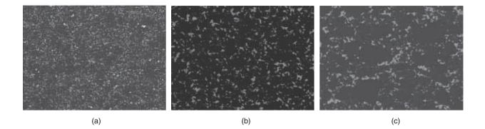
**Figure 22.11:** Microphotographs of diamond compacts: (a) fine-grained diamond, with mean grain size around 2  $\mu$ m; (b) medium grain, with mean grain size around 10  $\mu$ m; (c) coarse grain, with grain size around 25  $\mu$ m. *Source:* Courtesy of Kennametal, Inc.
