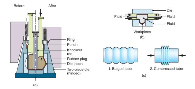
**Figure 16.29:** (a) The bulging of a tubular part with a flexible plug. Water pitchers can be made by this method. (b) Production of fittings for plumbing by expanding tubular blanks under internal pressure. The bottom of the piece is then punched out to produce a T. (c) Steps in manufacturing bellows.
