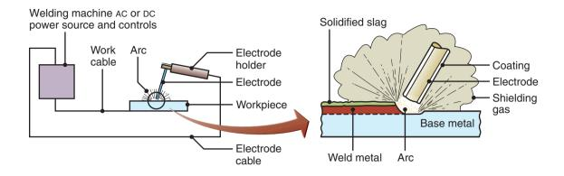
**Figure 30.8:** Schematic illustration of the shielded metal-arc welding process. About 50% of all large-scale industrial-welding operations use this process.
