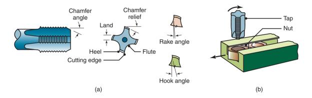
Figure 23.28: (a) Terminology for a tap. (b) Tapping of steel nuts in production.
