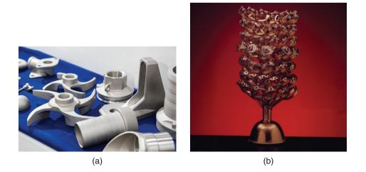
**Figure II.1:** (a) Examples of cast parts. (b) A tree of rings produced through investment casting. *Source:* (a) Shutterstock/Mr.1 (b) Courtesy of Romanoff, Inc.
