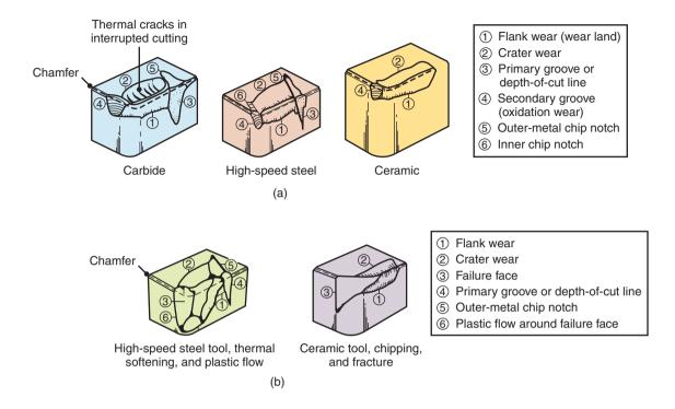
**Figure 21.18:** (a) Schematic illustrations of types of wear observed on various cutting tools. (b) Schematic illustrations of catastrophic tool failures. A wide range of parameters influence these wear and failure patterns. *Source:* Courtesy of V.C. Venkatesh.
