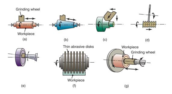
**Figure 26.3:** The types of workpieces and operations typical of grinding: (a) cylindrical surfaces, (b) conical surfaces, (c) fillets on a shaft, (d) helical profiles, (e) concave shape, (f) cutting off or slotting with thin wheels, and (g) internal grinding.
