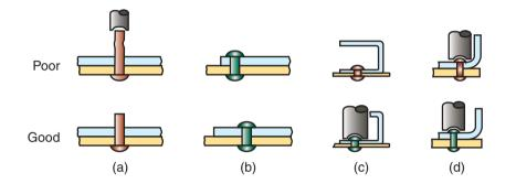
**Figure 32.15:** Design guidelines for riveting. (a) Exposed shank is too long; the result is buckling instead of upsetting. (b) Rivets should be placed sufficiently far from edges of the parts to avoid stress concentrations. (c) Joined sections should allow ample clearance for the riveting tools. (d) Section curvature should not interfere with the riveting process. *Source:* After J.G. Bralla.
