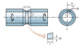
**Figure 2.10:** A typical torsion-test specimen, mounted between the two heads of a testing machine and twisted. Note the shear deformation of an element in the reduced section of the specimen.
