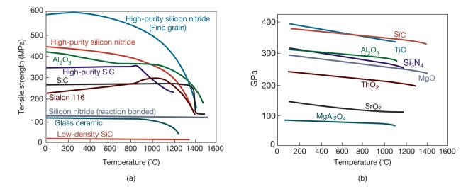
**Figure 8.3:** (a) Effect of temperature on the strength of various engineering ceramics. Note that much of the strength is maintained at high temperatures. (b) Effect of temperature on the modulus of elasticity for various ceramics. These results can be compared with Fig. 2.6.
