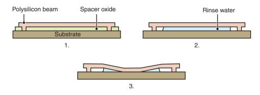
**Figure 29.5:** Stiction after wet etching: 1. Unreleased beam. 2. Released beam before drying. 3. Released beam pulled to the surface by capillary forces during drying. Once contact is made, adhesive forces prevent the beam from returning to its original shape. *Source:* After B. Bhushan.
