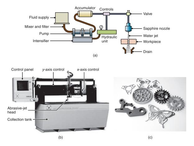
**Figure 27.15:** (a) Schematic illustration of the water-jet machining process. (b) A computer-controlled water-jet cutting machine. (c) Examples of various nonmetallic parts produced by the water-jet cutting process. *Source:* Courtesy of OMAX Corporation.
