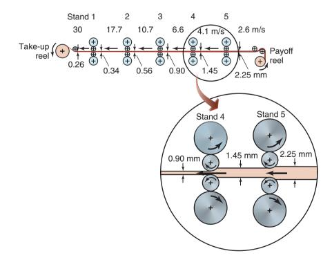
Figure 13.12: An example of a tandem-rolling operation.
