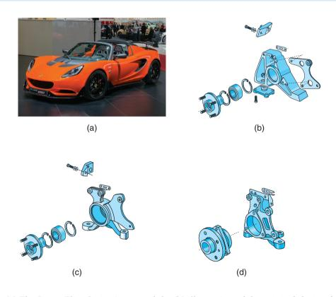
**Figure 14.23:** (a) The Lotus Elise Series 2 automobile, (b) illustration of the original design for the vertical suspension uprights, using an aluminum extrusion, (c) retrofit design, using a steel forging, (d) optimized steel forging design for new car models. *Source:* (a) Shutterstock/VanderWolf Images.
