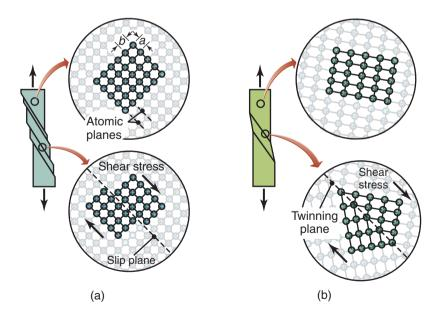
**Figure 1.6:** Permanent deformation of a single crystal under a tensile load. The highlighted grid of atoms emphasizes the motion that occurs within the lattice. (a) Deformation by slip. The b/a ratio influences the magnitude of the shear stress required to cause slip. (b) Deformation by twinning, involving the generation of a "twin" around a line of symmetry subjected to shear. Note that the tensile load results in a shear stress in the plane illustrated.
