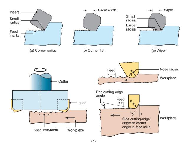
**Figure 24.8:** Schematic illustration of the effect of insert shape on feed marks on a face-milled surface: (a) small corner radius, (b) corner flat on insert, and (c) wiper, consisting of a small radius followed by a large radius, resulting in smoother feed marks. (d) Feed marks due to various insert shapes.
