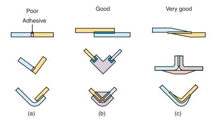
**Figure 32.11:** Various joint designs in adhesive bonding. Note especially that good designs require large contact areas between the members to be joined.
