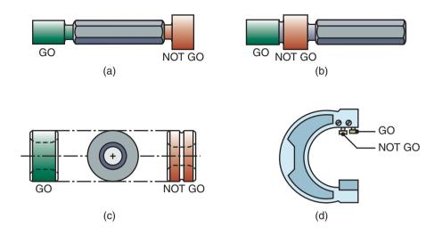
**Figure 35.11:** (a) Plug gage for holes, with *GO* and *NOT GO* on opposite ends of the gage. (b) Plug gage with *GO* and *NOT GO* on one end. (c) Plain ring gages for gaging round rods; note the difference in knurled surfaces to identify the two gages. (d) Snap gage with adjustable anvils.
