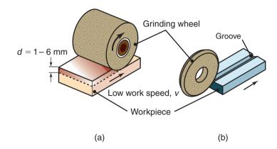
**Figure 26.25:** (a) Schematic illustration of the creep-feed grinding process; note the large wheel depth of cut, *d*. (b) A shaped groove produced on a flat surface by creep-feed grinding in one pass. Groove depth is typically on the order of a few mm. This operation also can be performed by some of the processes described in Chapter 27.
