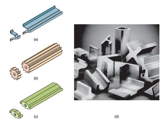
**Figure 15.2:** Extrusions and examples of products made by sectioning off extrusions. *Source:* Courtesy of Plymouth Engineered Shapes.
