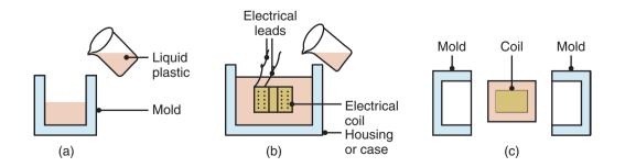
**Figure 19.19:** Schematic illustration of (a) casting, (b) potting, and (c) encapsulation processes for plastics and electrical assemblies, where the surrounding plastic serves as a dielectric.
