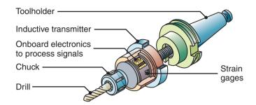
**Figure 37.25:** A toolholder equipped with thrust-force and torque sensors (smart toolholder), capable of continuously monitoring the cutting operation; such toolholders are essential for the adaptive control of manufacturing operations.
