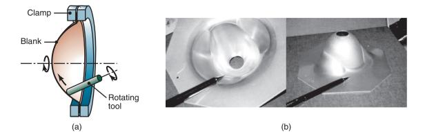
**Figure 16.50:** (a) Illustration of an incremental-forming operation. Note that no mandrel is used and that the final part shape depends on the path of the rotating tool. (b) An automotive headlight reflector produced through CNC incremental forming. Note that the part does not have to be axisymmetric. *Source:* (b) Courtesy of J. Jeswiet, Queen's University, Ontario.
