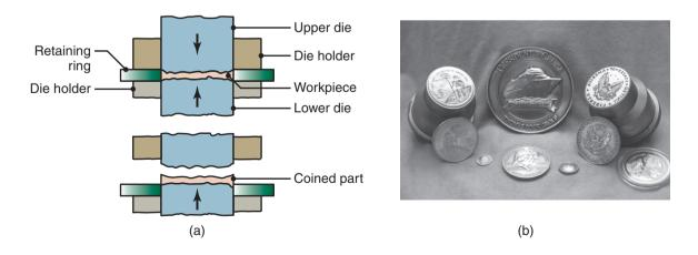
**Figure 14.11:** (a) Schematic illustration of the coining process. (b) An example of a modern coining operation, showing the coins and tooling. Note the detail and superior surface finish that can be achieved in this process. *Source:* Courtesy of C & W Steel Stamp Co., Inc.
