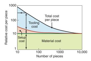
**Figure 14.21:** Typical cost per piece in forging; note how the setup and the tooling costs per piece decrease as the number of pieces forged increases if all pieces use the same die.
