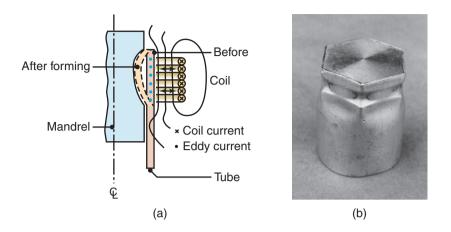
**Figure 16.54:** (a) Schematic illustration of the magnetic-pulse-forming process used to form a tube over a plug. (b) Aluminum tube collapsed over a hexagonal plug by the magnetic-pulse-forming process.
