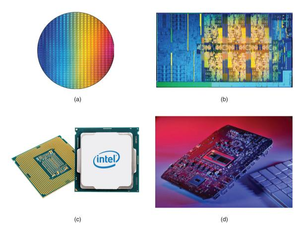
**Figure 28.1:** The 8th generation Intel<sup>®</sup> i7 core processor using 14 nm technology. (a) A 300-mm wafer with a large number of i7 core processor dies fabricated onto its surface; (b) detail view of an Intel i7 core die; (c) image of the Intel i7 die in package; and (d) motherboard of the Intel Hades Canyon Next Unit of Computing (NUC). The large IC package in the middle is an Intel core i7 processor. *Source:* Courtesy of Intel Corporation.
