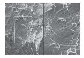
**Figure 2.28:** Typical fatigue-fracture surface on metals, showing beach marks. Magnification: left, 500×; right, 1000×. *Source:* After B.J. Schulze and S.L. Meiley and Packer Engineering Associates, Inc.
