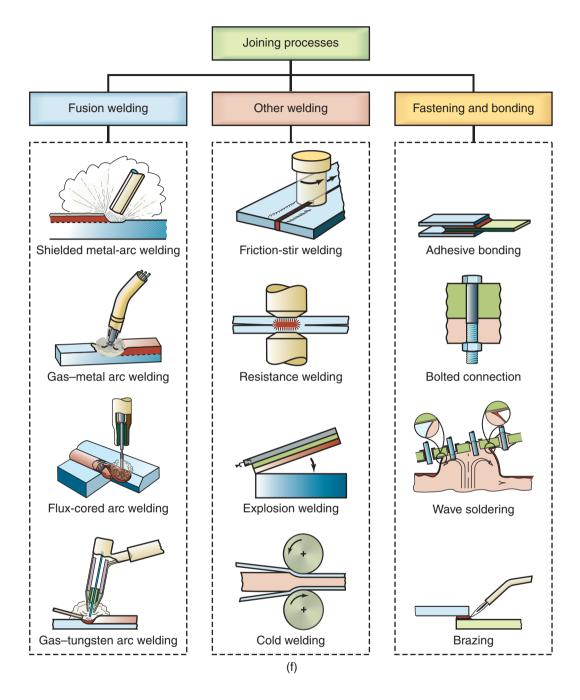
Figure I.7: (f) Schematic illustrations of various joining processes.
