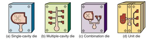
Figure 11.20: Various types of cavities in a die-casting die. *Source:* Courtesy of American Die Casting Institute.
