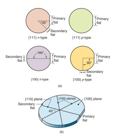
**Figure 28.7:** Identification of single-crystal wafers of silicon. This identification scheme is common for 150-mm diameter wafers, but notches are more common for larger wafers.
