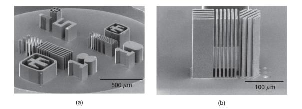
**Figure 29.18:** (a) Electroformed nickel structures, (b) Detail of nickel lines and spaces. *Source:* After T. Christenson, Sandia National Laboratories.
