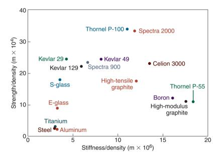
**Figure 9.3:** Specific tensile strength (tensile-strength-to-density ratio) and specific stiffness (modulus-ofelasticity-to-density ratio) for various fibers used in reinforced plastics. Note the wide range of specific strength and stiffness.
