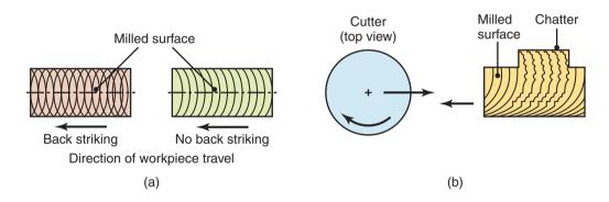
Figure 24.16: Machined surface features in face milling (see also Fig. 24.8).
