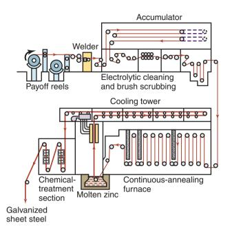
**Figure 34.11:** Flow line for the continuous hot-dipped galvanizing of sheet steel. The welder (upper left) is used to weld the ends of coils to maintain continuous material flow. *Source:* Courtesy of the American Iron and Steel Institute.
