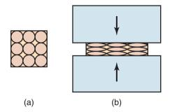
**Figure 1.12:** Plastic deformation of idealized (equiaxed) grains in a specimen subjected to compression (such as occurs in the forging or rolling of metals): (a) before deformation and (b) after deformation. Note the alignment of grain boundaries along a horizontal direction; this effect is known as *preferred orientation*.
