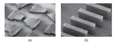
**Figure 29.20:** SEM images of Nd<sub>2</sub>Fe<sub>14</sub>B permanent magnets. The powder particle size ranges from 1 to 5  $\mu$ m, and the binder is a methylene chloride-resistant epoxy. Mild distortion is present in the images due to magnetic perturbation of the imaging electrons. Maximum energy products of 9 MGOe have been obtained with this process. *Source:* Courtesy of T. Christenson, Sandia National Laboratories.
