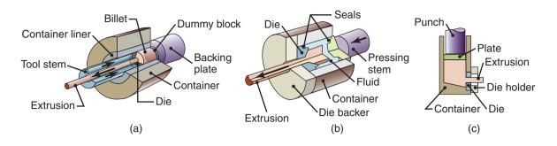
Figure 15.3: Types of extrusion: (a) indirect; (b) hydrostatic; (c) lateral.
