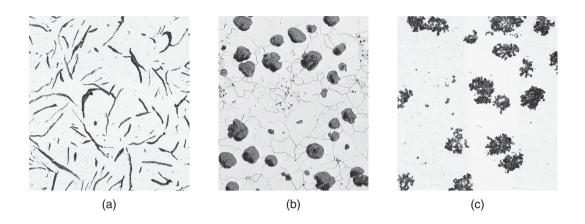
**Figure 4.11:** Microstructure for cast irons. Magnification:  $100 \times$ . (a) Ferritic gray iron with graphite flakes. (b) Ferritic ductile iron (nodular iron), with graphite in nodular form. (c) Ferritic malleable iron; this cast iron solidified as white cast iron, with the carbon present as cementite, and was heat treated to graphitize the carbon.
