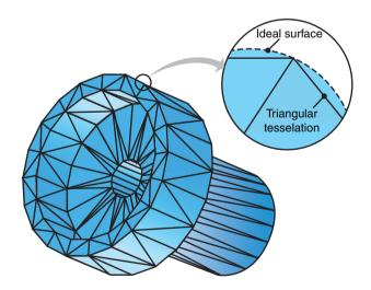
**Figure 38.5:** An example of an STL part description. Note that the surface is defined by a tessellation of triangles, and that there is an inherent error of form that occurs with curved surfaces; however, this can be brought to any desired tolerance by incorporating more triangles in the surface.
