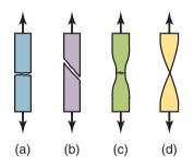
**Figure 2.21:** Schematic illustration of the types of fracture in tension: (a) brittle fracture in polycrystalline metals; (b) shear fracture in ductile single crystals—see also Fig. 1.6a; (c) ductile cup-and-cone fracture in polycrystalline metals; (d) complete ductile fracture in polycrystalline metals, with 100% reduction of area.
