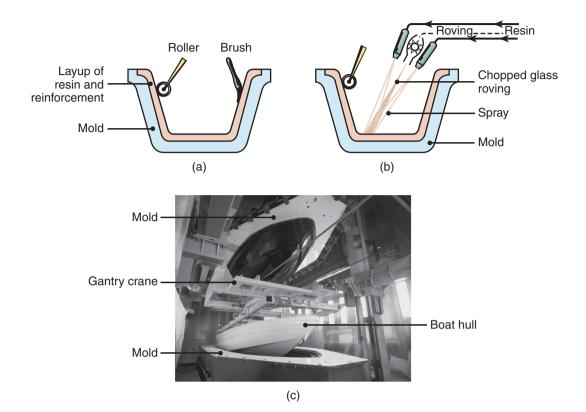
**Figure 19.25:** Manual methods of processing reinforced plastics: (a) hand layup and (b) spray layup. Note that, even though the process is slow, only one mold is required. The figures show a female mold, but male molds are used as well. These methods also are called *open-mold processing*. (c) A boat hull being made by these processes. *Source:* Courtesy of VEC Technology, LLC.
