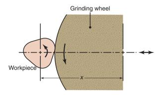
**Figure 26.20:** Schematic illustration of grinding a noncylindrical part on a cylindrical grinder with computer controls to produce the shape. The part rotation and the distance *x* between centers are varied and synchronized to grind the particular workpiece shape.
