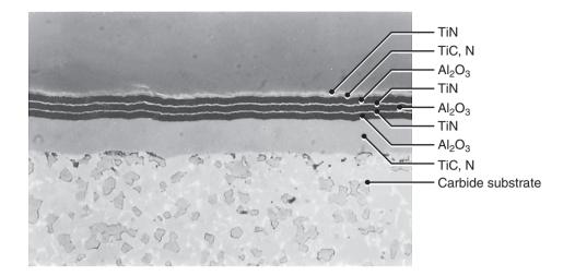
**Figure 22.8:** Multiphase coatings on a tungsten-carbide substrate. Three alternating layers of aluminum oxide are separated by very thin layers of titanium nitride. Inserts with as many as 13 layers of coatings have been made. Coating thicknesses are typically in the range from 2 to 10  $\mu$ m. *Source:* Courtesy of Kennametal Inc.
