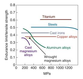
**Figure 2.17:** Ratio of endurance limit to tensile strength for various metals, as a function of tensile strength. Because aluminum does not have an endurance limit, the correlations for aluminum are based on a specific number of cycles, as is seen in Fig. 2.16.
