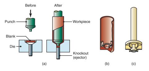
**Figure 15.15:** (a) Impact extrusion of a collapsible tube by the *Hooker process*. (b) and (c) Two examples of products made by impact extrusion. These parts also may be made by casting, forging, or machining. The choice of process depends on the materials involved, part dimensions and wall thickness, and the properties desired. Economic considerations also are important in final process selection.
