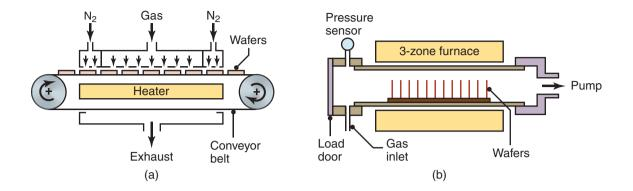
**Figure 28.8:** Schematic diagrams of (a) a continuous, atmospheric-pressure CVD reactor and (b) a low-pressure CVD. *Source:* After S.M. Sze.
