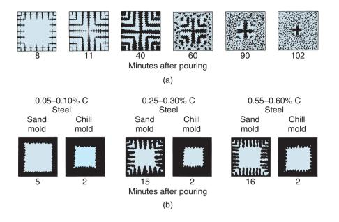
**Figure 10.5:** (a) Solidification patterns for gray cast iron in a 180-mm square casting. Note that after 11 minutes of cooling, dendrites begin to reach each other, but the casting is still mushy throughout. It takes about 2 hours more for this casting to solidify completely. (b) Solidification of carbon steels in sand and chill (metal) molds. Note the difference in solidification patterns as the carbon content of the metal increases. *Source:* After H.F. Bishop and W.S. Pellini.
