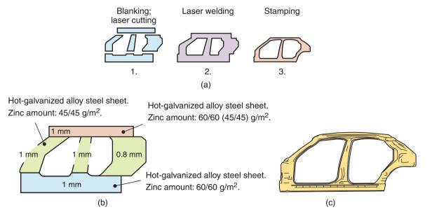
**Figure 16.7:** Production of an outer side panel of a car body by laser butt welding and stamping. The thickness of each section is as indicated. *Source:* After M. Geiger and T. Nakagawa.
