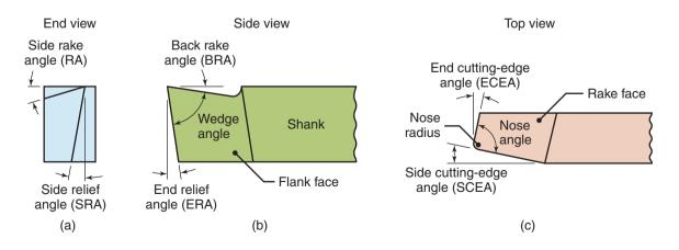
**Figure 23.4:** Designations for a right-hand tool. *Right-hand* means that the tool travels from right to left, as shown in Fig. 23.3b.
