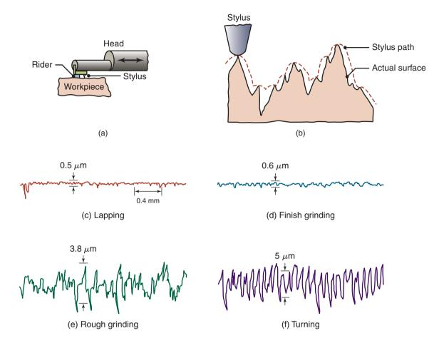
**Figure 33.4:** (a) Measuring surface roughness with a stylus. The rider supports the stylus and guards against damage. (b) Path of the stylus in surface-roughness measurements (broken line), compared with the actual roughness profile. Note that the profile of the stylus path is smoother than that of the actual surface. (c) through (f) Typical surface profiles produced by various machining and surface-finishing processes. Note the difference between the vertical and horizontal scales.
