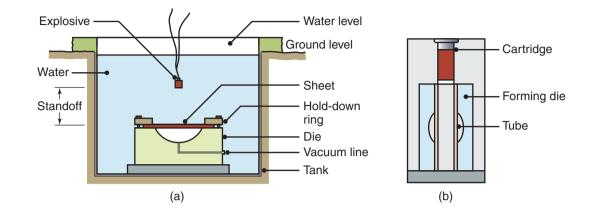
**Figure 16.53:** (a) Schematic illustration of the explosive-forming process. (b) Illustration of the confined method of the explosive bulging of tubes.
