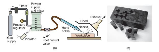
**Figure 27.16:** (a) Schematic illustration of the abrasive-jet machining process. (b) Examples of parts made by abrasive-jet machining, produced in 50-mm thick 304 stainless steel. *Source:* Courtesy of OMAX Corporation.
