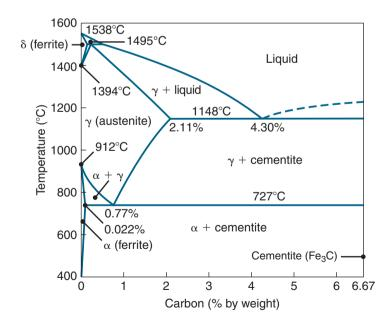
**Figure 4.6:** The iron–iron-carbide phase diagram. Because of the importance of steel as an engineering material, this diagram is one of the most important of all phase diagrams.
