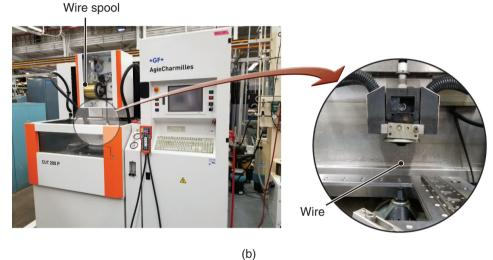
Figure 27.11: (a) Cutting a thick plate with wire EDM. (b) A computer-controlled wire EDM machine. Source: Courtesy of L. Love, Oak Ridge National Laboratory.
