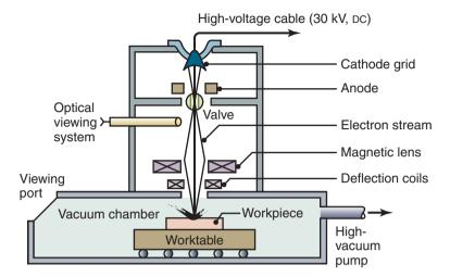
**Figure 27.14:** Schematic illustration of the electron-beam machining process. Unlike LBM, this process requires a vacuum, so the workpiece size is limited to the size of the vacuum chamber.
