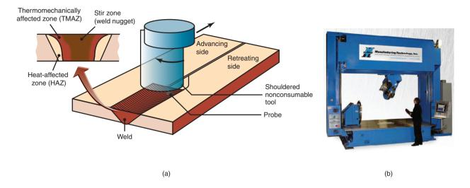
**Figure 31.5:** The friction-stir-welding process. (a) Schematic illustration of friction-stir-welding. Aluminumalloy plates up to 75 mm thick have been welded by this process. (b) Multi-axis friction stir welding machine for large workpieces such as aircraft wing and fuselage structures. This machine can develop 67 kN axial forces and welding speeds up to 1.8 m/s. It is powered by a 15 kW spindle motor. *Source:* (b) Courtesy of Manufacturing Technology, Inc.
