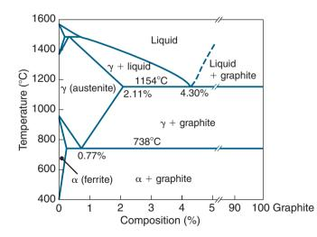
**Figure 4.10:** Phase diagram for the iron–carbon system with graphite (instead of cementite) as the stable phase. Note that this figure is an extended version of Fig. 4.6.
