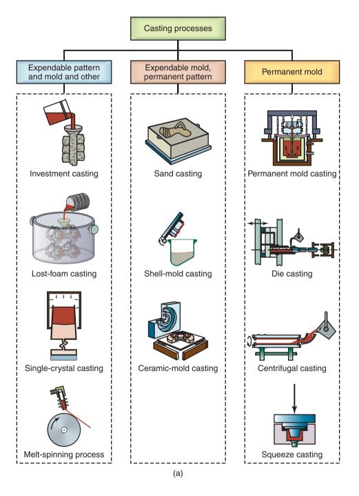
Figure I.7: (a) Schematic illustrations of various casting processes.
