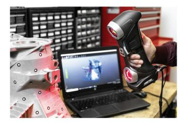
**Figure 37.27:** The use of a 3D scanner to digitize the geometry of a stamped part to create a 3D data file describing the geometry. The data file can then be used for quality control, or it can be additively manufactured or machined to produce a part with the same geometry or a mold for stamping. *Source:* Courtesy of Creaform.
