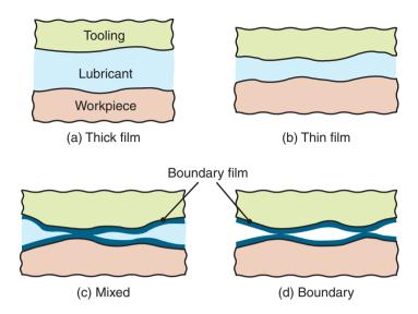
Figure 33.13: Regimes of lubrication generally occurring in metalworking operations. *Source:* After W.R.D. Wilson.
