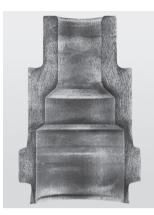
**Figure 15.13:** A cross section of the metal part in Fig. 15.12, showing the grain-flow pattern. *Source:* Courtesy of National Machinery Company, LLC.
