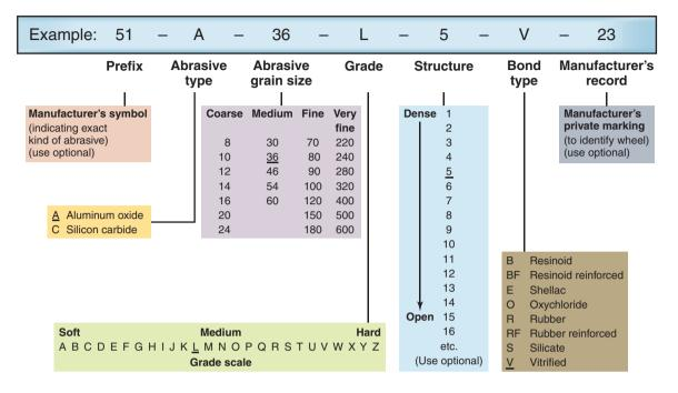
Figure 26.7: Standard marking system for aluminum-oxide and silicon-carbide bonded abrasives.
