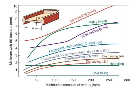
Figure 40.4: Manufacturing process capabilities for minimum part dimensions. Source: After J.A. Schey.
