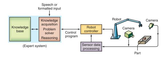
Figure 39.6: Illustration of an expert system as applied to an industrial robot guided by machine vision.
