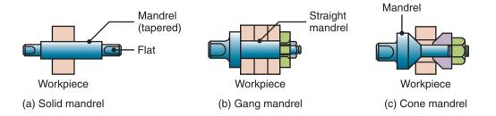
**Figure 23.9:** Various types of mandrels to hold workpieces for turning; they are usually mounted between centers on a lathe. Note that in (a) both the cylindrical and the end faces of the workpiece can be machined, whereas in (b) and (c) only the cylindrical surfaces can be machined.
