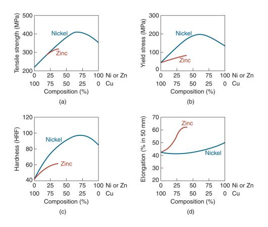
**Figure 4.5:** Mechanical properties of copper–nickel and copper–zinc alloys as a function of their composition. The curves for zinc are short, because zinc has a maximum solid solubility of 40% in copper.
