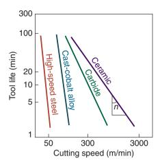
**Figure 21.17:** Tool-life curves for a variety of cutting-tool materials. The negative reciprocal of the slope of these curves is the exponent n in the Taylor tool-life equation [Eq. (21.25)], and C is the cutting speed at T = 1 min, ranging from about 60 to 3000 m/min in this figure.
