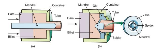
**Figure 15.8:** Extrusion of a seamless tube (a) using an internal mandrel that moves independently of the ram; an alternative arrangement has the mandrel integral with the ram, (b) using a spider die (see Fig. 15.9) to produce seamless tubing.
