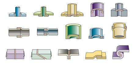
**Figure 32.3:** Joint designs commonly used in brazing operations. The clearance between the two parts being brazed is an important factor in joint strength. If the clearance is too small, the molten braze metal will not fully penetrate the interface; if it is too large, there will be insufficient capillary action for the metal to fill the interface.
