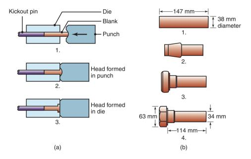
**Figure 14.12:** (a) Heading operation to form heads on fasteners, such as nails and rivets. (b) Sequence of operations used to produce a typical bolt head by heading.
