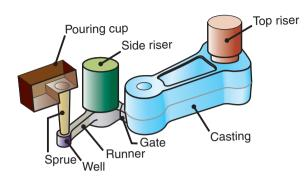
**Figure 10.10:** Schematic illustration of a typical riser-gated casting. Risers serve as reservoirs, supplying molten metal to the casting as it shrinks during solidification.
