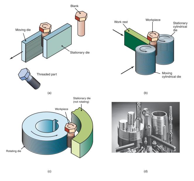
**Figure 13.17:** Thread-rolling processes: (a) reciprocating flat dies used to produce a threaded fastener; (b) two-roll dies; (c) rotary or planetary die set; (d) A collection of thread-rolled parts made economically at high production rates. *Source:* Courtesy of Tesker Manufacturing Corp.
