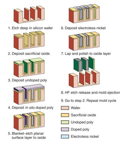
**Figure 29.22:** Illustration of the hexagonal honeycomb structure, silicon micromachining, and thin-film deposition (HEXSIL).
