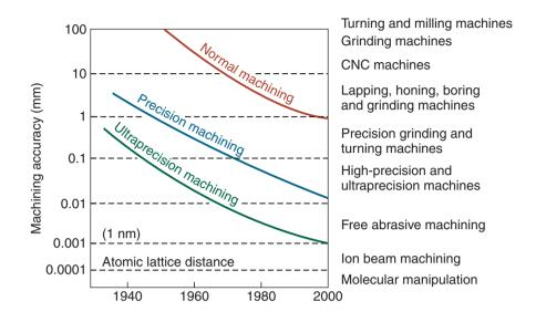
Figure 25.17: Improvements in machining accuracy over the years, using ultraprecision machining technologies. *Source:* After C.J. McKeown, N. Taniguchi, G. Byrne, D. Dornfeld, and B. Denkena.
