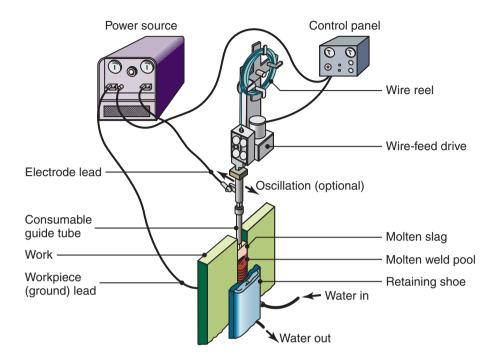
Figure 30.14: Equipment used for electroslag-welding operations.
