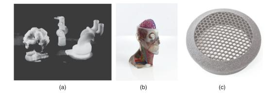
**Figure 20.1:** Examples of parts made by additive manufacturing processes: (a) a selection of parts from fused-deposition modeling; (b) full-color model of an anatomical model; and (c) a speaker cover produced by the CLIP process. *Source:* (a) and (b) Courtesy of Stratasys, Inc., (c) Courtesy of Carbon, Inc.
