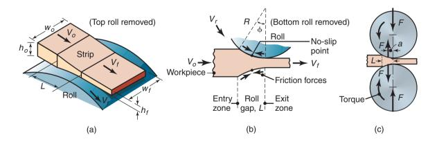
**Figure 13.2:** (a) Schematic illustration of the flat-rolling process. (b) Friction forces acting on strip surfaces. (c) Roll force, *F*, and torque, *T*, acting on the rolls. The width of the strip, *w*, usually increases during rolling, as shown later in Fig. 13.5.
