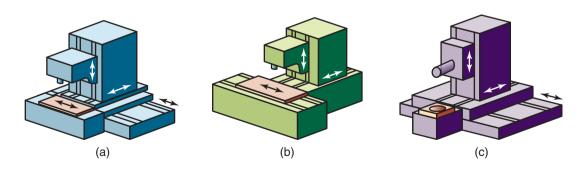
**Figure 25.10:** Schematic illustration of a reconfigurable modular machining center capable of accommodating workpieces of different shapes and sizes and requiring different machining operations on their various surfaces. *Source:* After Y. Koren.
