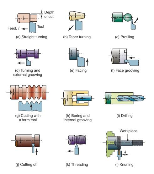
**Figure 23.1:** Miscellaneous cutting operations that can be performed on a lathe. Note that all parts are axisymmetric. The tools used, their shape, and the processing parameters are described in detail throughout this chapter.
