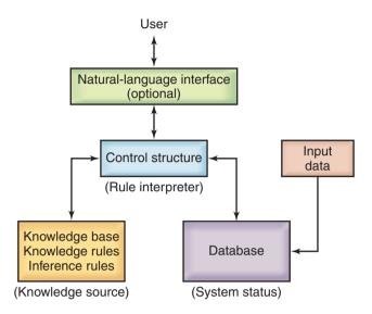
**Figure 39.5:** Basic structure of an expert system. The knowledge base consists of knowledge rules (general information about the problem) and inference rules (the way conclusions are reached). The results may be communicated to the user through the natural-language interface.
