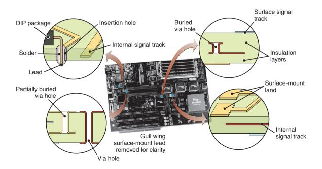
Figure 28.35: Printed circuit board structures and design features.
