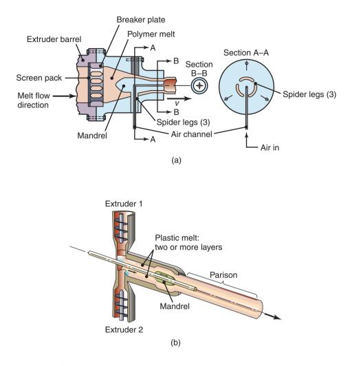
**Figure 19.4:** Extrusion of tubes. (a) Extrusion using a spider die (see also Fig. 15.8) and pressurized air. (b) Coextrusion for producing a parison for a bottle.
