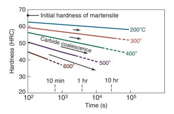
**Figure 4.14:** Hardness of tempered martensite as a function of tempering time for 1080 steel quenched to 65 HRC. Hardness decreases because the carbide particles coalesce and grow in size, thereby increasing the interparticle distance of the softer ferrite.
