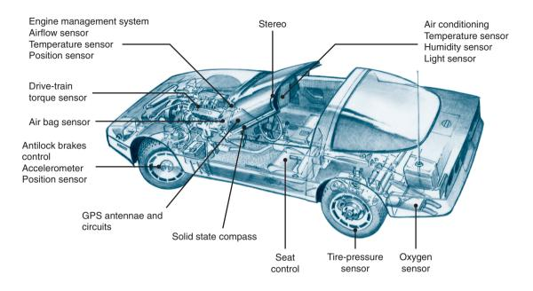
Figure V.2: Microelectronic and microelectromechanical devices and parts used in a typical automobile.
