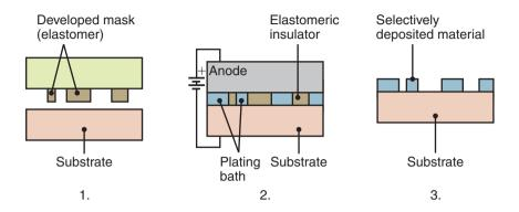
**Figure 29.24:** The instant-masking process: 1. Bare substrate; 2. During deposition, with the substrate and instant mask in contact; 3. The resulting pattern deposited. *Source:* Courtesy of A. Cohen, MEMGen Corporation.
