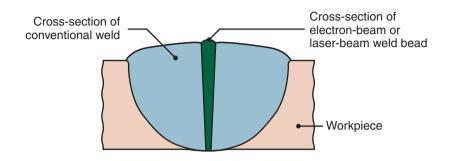
**Figure 31.15:** The relative sizes of the weld beads obtained by tungsten-arc and by electron-beam or laserbeam welding.
