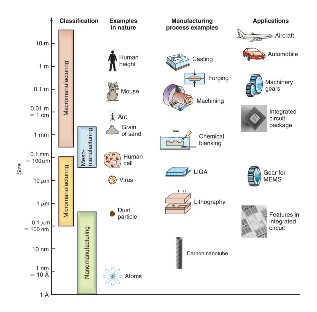
**Figure V.1:** Illustration of the regimes of macro-, meso-, micro-, and nanomanufacturing, the range of common sizes of parts, and the capabilities of manufacturing processes in producing those parts.
