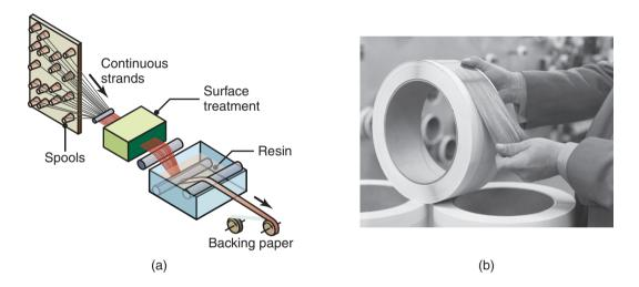
**Figure 19.22:** (a) Manufacturing process for polymer-matrix composite tape. (b) Boron-epoxy prepreg tape. These tapes are then used in making reinforced plastic parts and components with high strength-to-weight and stiffness-to-weight ratios, particularly important for aircraft and aerospace applications and sports equipment. *Source:* (a) After T.W. Chou, R.L. McCullough, and R.B. Pipes. (b) Courtesy of Avco Specialty Materials/Textron.
