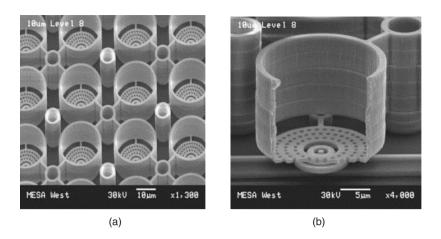
**Figure 29.23:** (a) An array of micro-mass analysis systems consisting of cylindrical ion traps, constructed of 14 layers of molded tungsten, including eight layers for the ring electrode. (b) Detail view of the tungsten structures. *Source:* Courtesy of Sandia National Laboratories.
