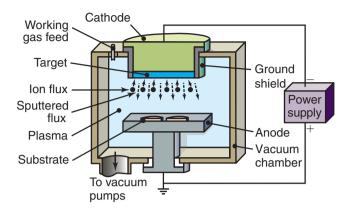
Figure 34.4: Schematic illustration of the sputtering process.
