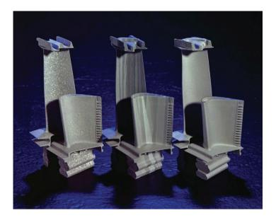
**Figure 1.1:** Turbine blades for jet engines, manufactured by three different methods: left: conventionally cast; center: directionally solidified, with columnar grains as can be seen from the vertical streaks, and right: single crystal. Although more expensive, single-crystal blades have properties at high temperatures that are superior to those of other blades. *Source:* Courtesy of NASA.
