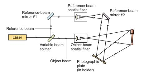
**Figure 36.13:** Schematic illustration of the basic optical system used in holography elements in radiography for detecting flaws. *Source:* ASM International.
