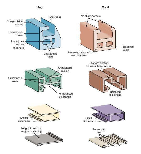
**Figure 15.17:** Examples of poor and good design practices for extrusion. Note the importance of eliminating sharp corners and of keeping section thicknesses uniform.
