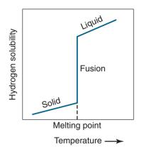
**Figure 10.17:** Solubility of hydrogen in aluminum. Note the sharp decrease in solubility as the molten metal begins to solidify.
