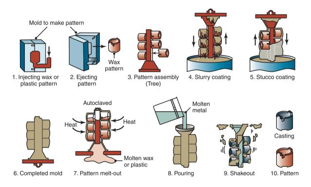
**Figure 11.14:** Schematic illustration of the investment-casting (lost-wax) process. Castings produced by this method can be made with very fine detail and from a variety of metals. *Source:* Courtesy of Steel Founders' Society of America.
