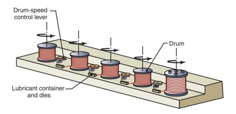
**Figure 15.25:** An illustration of multistage wire drawing typically used to produce copper wire for electrical wiring. Shown is a five bull block configuration; wire drawing machines can incorporate 15 or more drums, depending on the material and wire size. *Source:* After H. Auerswald.
