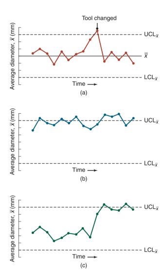
**Figure 36.6:** Control charts. (a) Process begins to become out of control because of such factors as tool wear (*drift*); the tool is changed and the process is then in statistical control. (b) Process parameters are not set properly; thus, all parts are around the upper control limit (*shift in mean*). (c) Process becomes out of control, because of factors such as a change in the properties of the incoming material (*shift in mean*).
