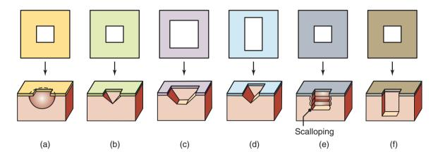
**Figure 28.24:** Various holes generated from a square mask in (a) isotropic (wet) etching; (b) orientationdependent etching (ODE); (c) ODE with a larger hole; (d) ODE of a rectangular hole; (e) deep reactive-ion etching; and (f) vertical etching. *Source:* After M. Madou.
