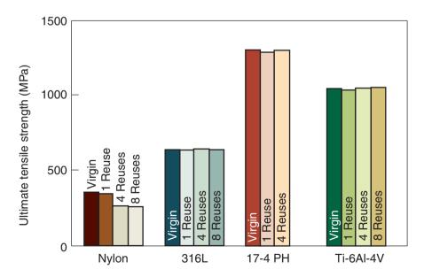
**Figure 20.24:** Effect of powder reuse on mean ultimate tensile strength for nylon, 316L stainless steel, 17-4 precipitation hardening stainless steel and titanium alloy Ti-6Al-4V.
