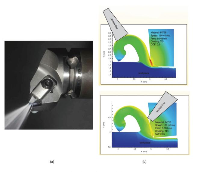
**Figure 22.13:** (a) A turning insert with coolant applied through the tool; (b) comparison of temperature distributions for conventional and through-the-tool application. *Source:* Courtesy of Kennametal, Inc.
