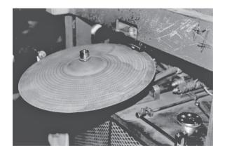
**Figure 16.58:** Automated hammering of a cymbal on a peening machine. *Source:* Courtesy of W. Blanchard, Sabian Ltd.
