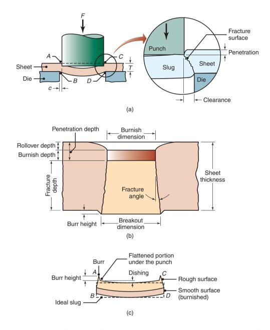
**Figure 16.2:** (a) Schematic illustration of shearing with a punch and die, indicating some of the process variables. Characteristic features of (b) a punched hole and (c) the slug. (Note that the scales of (b) and (c) are different.)
