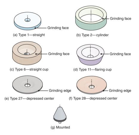
**Figure 26.5:** Common types of grinding wheels made with conventional abrasives. Note that each wheel has a specific *grinding face*; grinding on other surfaces is improper and unsafe.
