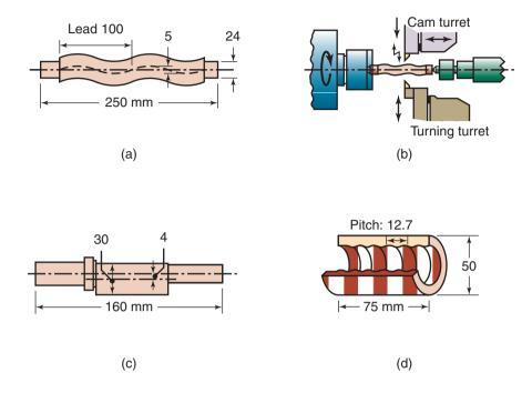
Figure 23.13: Examples of complex shapes that can be produced on a CNC lathe.
