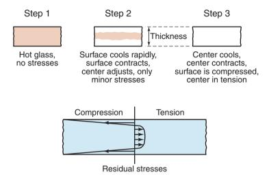
**Figure 18.14:** (a) Stages involved in inducing compressive surface residual stresses for improved strength. (b) Residual stresses in a tempered glass plate. *Source:* Courtesy of Corning Glass Works.
