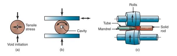
**Figure 13.19:** Cavity formation in a solid, round bar and its utilization in the rotary tube-piercing process for making seamless pipe and tubing (see also Fig. 2.9).
