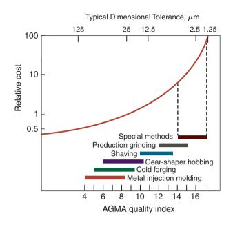
Figure 24.37: Gear manufacturing cost as a function of gear quality.
