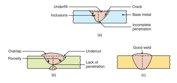
Figure 30.22: Examples of various defects in fusion welds.
