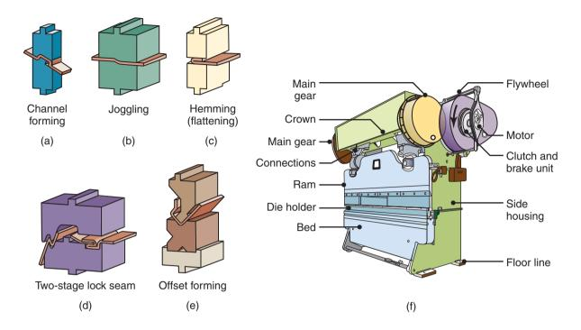
**Figure 16.23:** (a) through (e) Schematic illustrations of various bending operations in a press brake. (f) Schematic illustration of a press brake. *Source:* Courtesy of Verson Allsteel Company.
