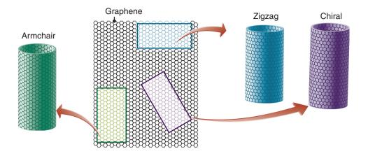
**Figure 8.7:** Forms of carbon nanotubes produced from a section of graphene: armchair, zigzag, and chiral. Armchair nanotubes are noteworthy for their high electrical conductivity, whereas zigzag and chiral nanotubes are semiconductors.
