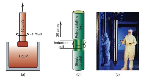
**Figure 11.26:** Two methods of crystal growing: (a) crystal pulling (Czochralski process) and (b) the floating-zone method. (c) A single-crystal ingot produced by the Czochralski process. *Source:* Courtesy of Intel Corp.
