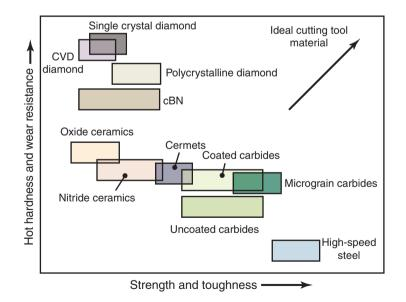
**Figure 22.9:** Ranges of mechanical properties for various groups of tool materials (see also Tables 22.1 through 22.5).
