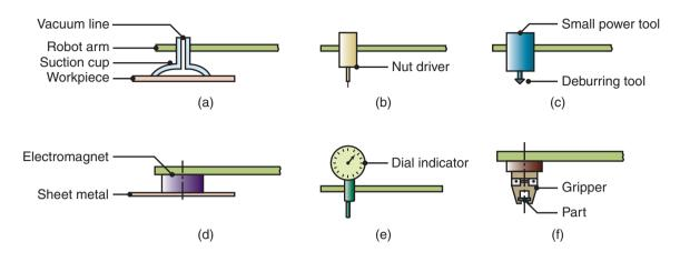
Figure 37.18: Types of tools and devices attached to end effectors to perform a variety of operations.
