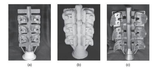
**Figure 11.16:** Progression of the tree. (a) After assembly of blanks onto the tree; (b) after coating with investment; (c) after removal from the mold. *Source:* Courtesy of M. Hawkins, Zimmer Biomet, Inc.
