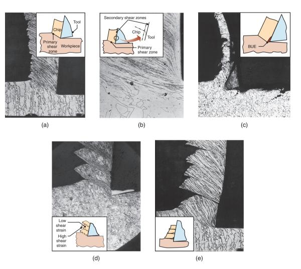
**Figure 21.5:** Basic types of chips produced in orthogonal metal cutting, their schematic representation, and photomicrographs of the cutting zone: (a) continuous chip, with narrow, straight, and primary shear zone; (b) continuous chip, with secondary shear zone at the chip–tool interface; (c) built-up edge; (d) segmented or nonhomogeneous chip; and (e) discontinuous chip. *Source:* After M.C. Shaw, P.K. Wright, and S. Kalpakjian.
