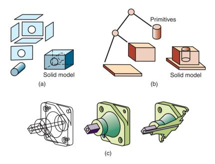
**Figure 38.4:** (a) Boundary representation of solids, showing the enclosing surfaces of the solid model and the generated solid model. (b) A solid model represented as compositions of solid primitives. (c) Three representations of the same part by CAD. *Source:* After P. Ranky.
