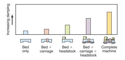
**Figure 25.15:** The damping of vibrations as a function of the number of components on a lathe. Joints dissipate energy; the greater the number of joints, the higher is the damping capacity of the machine. *Source:* After J. Peters.
