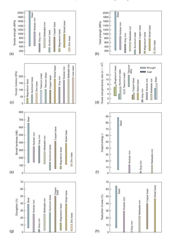
**Figure 12.5:** Mechanical properties for various groups of cast alloys. Note that even within the same group, the properties vary over a wide range, particularly for cast steels. *Source:* Courtesy of Steel Founders' Society of America.
