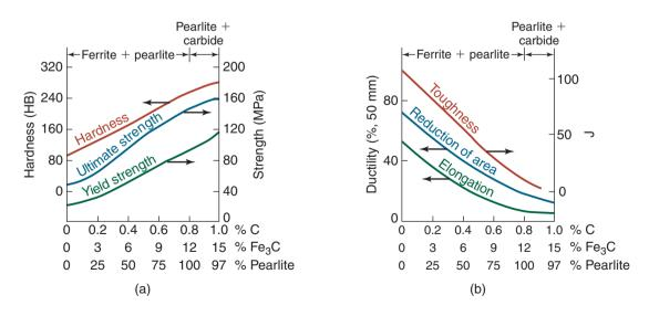
**Figure 4.17:** Mechanical properties of annealed steels as a function of composition and microstructure. Note in (a) the increase in hardness and strength, and in (b), the decrease in ductility and toughness, with increasing amounts of pearlite and iron carbide.
