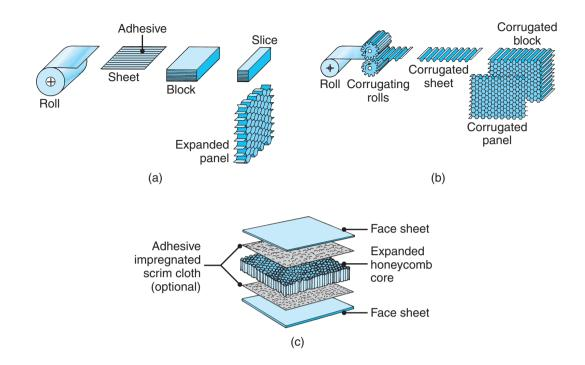
**Figure 16.59:** Methods of manufacturing honeycomb structures: (a) expansion process; (b) corrugation process; and (c) assembling a honeycomb structure into a laminate.
