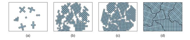
**Figure 1.11:** Schematic illustration of the stages during the solidification of molten metal; each small square represents a unit cell. (a) Nucleation of crystals at random sites in the molten metal; note that the crystallographic orientation of each site is different. (b) and (c) Growth of crystals as solidification continues. (d) Solidified metal, showing individual grains and grain boundaries; note the different angles at which neighboring grains meet each other.
