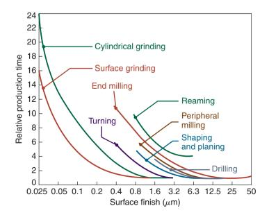
**Figure 40.3:** Relative production time as a function of surface finish produced by various manufacturing processes (see also Fig. 26.35).
