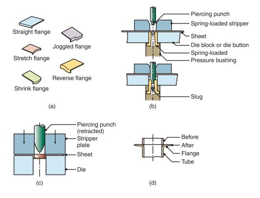
**Figure 16.25:** Various flanging operations. (a) Flanges on flat sheet. (b) Dimpling. (c) The piercing of sheet metal to form a flange. In this operation, a hole does not have to be pre-punched before the punch descends. Note, however, the rough edges along the circumference of the flange. (d) Flanging of a tube; note the thinning of the edges of the flange.
