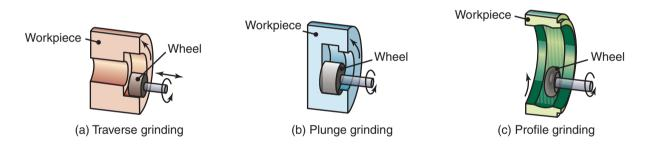
**Figure 26.23:** Schematic illustrations of internal grinding operations: (a) traverse grinding, (b) plunge grinding, and (c) profile grinding.
