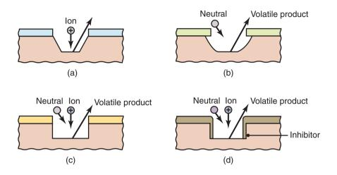
**Figure 28.22:** Machining profiles associated with different dry-etching techniques: (a) sputtering; (b) chemical; (c) ion-enhanced energetic; and (d) ion-enhanced inhibitor. *Source:* After M. Madou.
