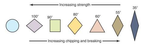
**Figure 22.4:** Relative edge strength and tendency for chipping of inserts with various shapes. Strength refers to the cutting edge indicated by the included angles. *Source:* Courtesy of Kennametal Inc.
