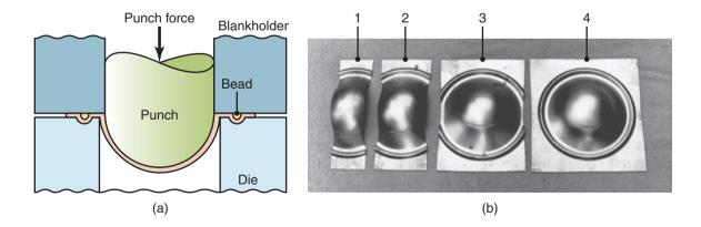
**Figure 16.13:** (a) A cupping test (the Erichsen test) to determine the formability of sheet metals. (b) Bulgetest results on steel sheets of various widths. The specimen farthest left is subjected to, basically, simple tension. The specimen that is farthest right is subjected to equal biaxial stretching. *Source:* (b) Courtesy of ArcelorMittal.
