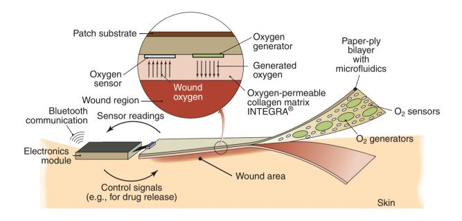
**Figure I.3:** A flexible hybrid electronic wound care system (see Section 28.15). The device integrates communication ability (in this case a Bluetooth ability), sensors to detect the oxygen levels at the wound, and oxygen generating devices to increase oxygen level to optimize healing. These devices use combinations of printed electronic devices and silicon-based integrated circuits. *Source:* Courtesy of NextFlex.
