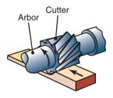
Figure 24.4: Schematic illustration of peripheral milling.
