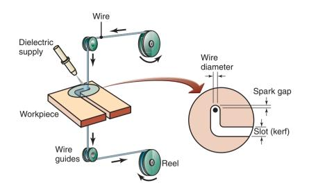
**Figure 27.10:** Schematic illustration of the wire EDM process. As many as 50 hours of machining can be performed with one reel of wire, which is then discarded.
