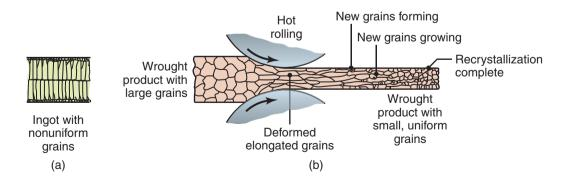
**Figure 13.6:** Changes in the grain structure of cast or of large-grain wrought metals during hot rolling. Hot rolling is an effective way of reducing grain size in metals for improved strength and ductility. The cast structures of ingots or of continuous castings are converted to a wrought structure by hot working.
