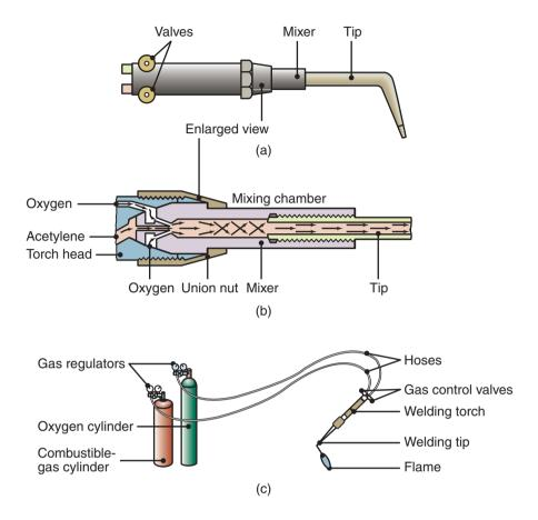
**Figure 30.2:** (a) General view of, and (b) cross section of, a torch used in oxyacetylene welding. The acetylene valve is opened first. The gas is lit with a spark lighter or a pilot light. Then the oxygen valve is opened and the flame is adjusted. (c) Basic equipment used in oxyfuel–gas welding. To ensure correct connections, all threads on acetylene fittings are left handed, whereas those for oxygen are right handed. Oxygen regulators usually are painted green and acetylene regulators red.
