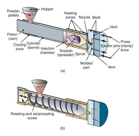
**Figure 19.7:** Schematic illustration of injection molding with (a) a plunger and (b) a reciprocating rotating screw.
