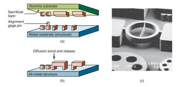
**Figure 29.21:** Multilevel MEMS fabrication through wafer-scale diffusion bonding. (a) Two wafers are aligned and assembled. (b) Resultant structure after diffusion bonding and removal of alumina substrate. (c) A suspended ring structure for measurement of tensile strain, formed by two-layer wafer-scale diffusion bonding. *Source:* (c) Courtesy of T. Christenson, Sandia National Laboratories.
