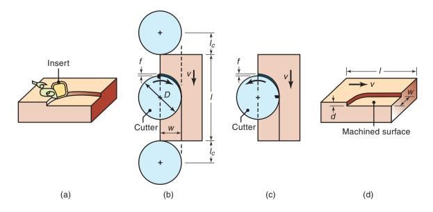
**Figure 24.6:** (a) Face-milling operation with cutter removed, showing the action of a single insert; (b) climb milling; (c) conventional milling; and (d) dimensions in face milling. The width of cut, *w*, is not necessarily the same as the cutter radius.
