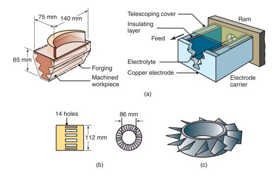
**Figure 27.5:** Typical parts made by electrochemical machining. (a) Turbine blade made of a nickel alloy of 360 HB; note the shape of the electrode on the right. (b) Thin slots on a 4340-steel roller-bearing cage. (c) Integral airfoils on a compressor disk.
