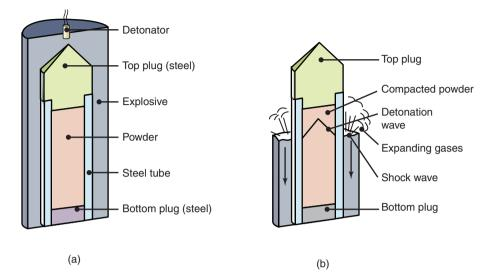
**Figure 17.21:** Schematic illustration of explosive compaction. (a) A tube filled with powder is surrounded by explosive media inside a container typically made of cardboard or wood. (b) After detonation, a compression wave follows the detonation wave, resulting in a compacted powder material.
