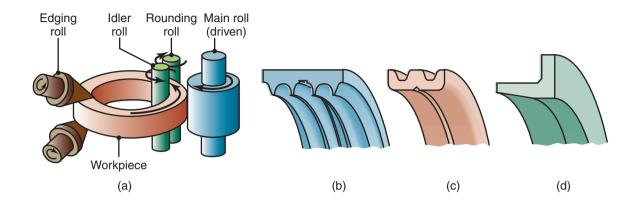
**Figure 13.16:** (a) Schematic illustration of a ring-rolling operation. Thickness reduction results in an increase in the part diameter. (b) through (d) Examples of cross sections that can be formed by ring rolling.
