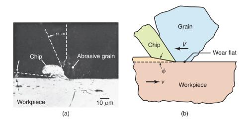
**Figure 26.9:** (a) Grinding chip being produced by a single abrasive grain; note the large negative rake angle of the grain. (b) Schematic illustration of chip formation by an abrasive grain with a wear flat; note the negative rake angle of the grain and the small shear angle. *Source:* (a) After M.E. Merchant.
