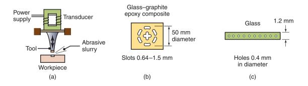
**Figure 26.26:** (a) Schematic illustration of the ultrasonic machining process. (b) and (c) Types of parts made by this process. Note the small size of the holes produced.
