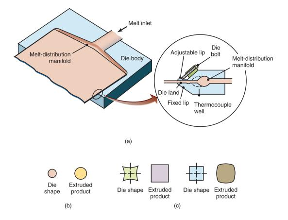
**Figure 19.3:** Common extrusion die geometries: (a) coat-hanger die for extruding sheet; (b) round die for producing rods; and (c) nonuniform recovery of the part after it exits the die.
