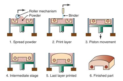
Figure 20.13: Schematic illustration of the binder-jet printing process.
