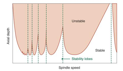
**Figure 25.16:** The milling stability lobe diagram, or stability map, showing the spindle speed against the limiting axial depth of cut to avoid chatter. Stable and unstable combinations are identified by the white and shaded regions. *Source:* After T. Schmitz, University of North Carolina at Charlotte.
