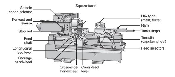
**Figure 23.10:** Schematic illustration of the components of a turret lathe; note the two turrets: square and hexagonal (main).
