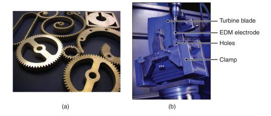
**Figure 27.1:** Examples of parts made by advanced machining processes. (a) Samples of parts produced by water-jet cutting. (b) Turbine blade, produced by plunge electrical-discharge machining, in a fixture to produce forced air cooling channels also by electrical-discharge machining. *Source:* (a) Courtesy of OMAX Corporation; (b) Courtesy of HI-TEK Mfg., Inc.
