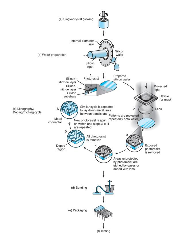
Figure 28.2: Outline of the general fabrication sequence for integrated circuits.
