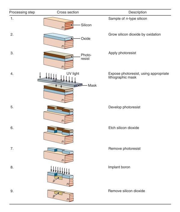
Figure 28.26: Fabrication sequence for a *pn*-junction diode.
