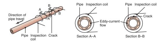
Figure 36.12: Changes in eddy-current flow caused by a defect in a part. Source: ASM International.
