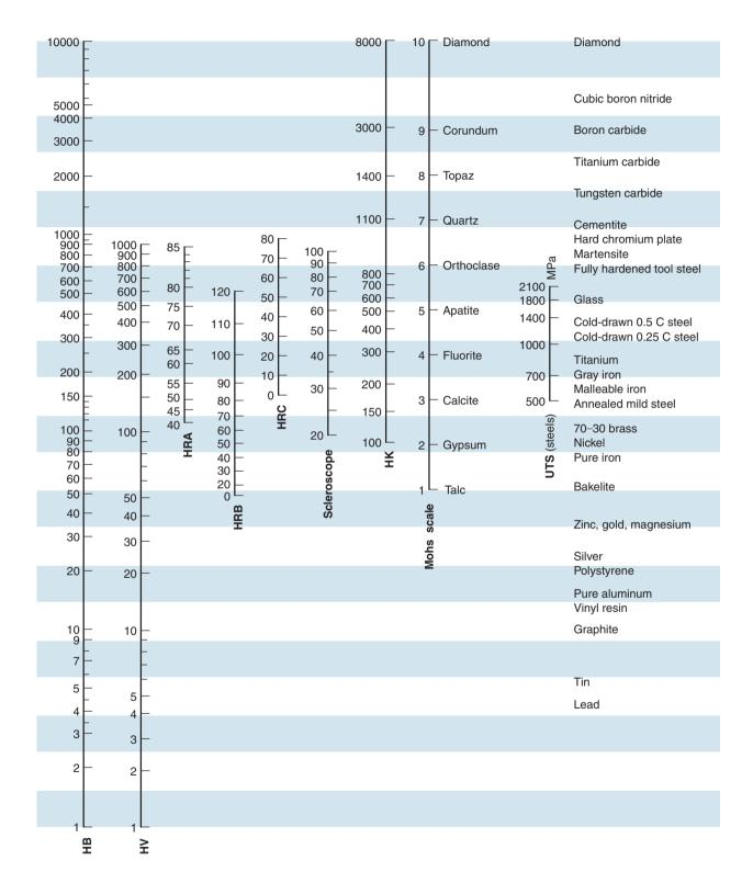
**Figure 2.15:** Chart for converting various hardness scales; note the limited range of most of the scales. Because of the many factors involved, these conversions are approximate.
