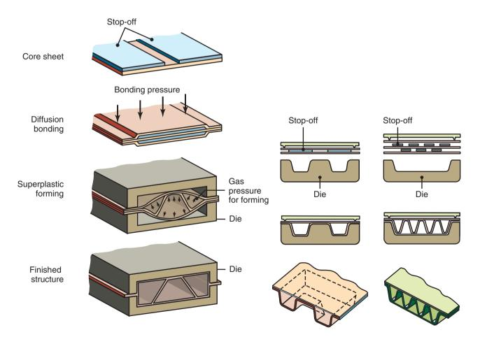
**Figure 31.18:** The sequence of operations in the fabrication of a structure by the diffusion bonding and superplastic forming of three originally flat sheets (see also Fig. 16.52).
