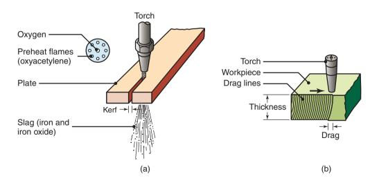
**Figure 30.18:** (a) Flame cutting of a steel plate with an oxyacetylene torch, and a cross-section of the torch nozzle. (b) Cross-section of a flame-cut plate, showing drag lines.
