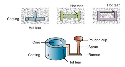
**Figure 10.14:** Examples of hot tears in castings. These defects occur because the casting cannot shrink freely during cooling, owing to constraints in various portions of the molds and cores. Exothermic (heat producing) compounds may be used as *exothermic padding* to control cooling at critical regions to avoid hot tearing.
