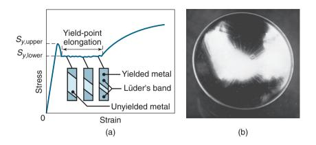
**Figure 16.12:** (a) Yield-point elongation in a sheet-metal specimen. (b) Stretcher strains at the bottom of a steel can for household products.
