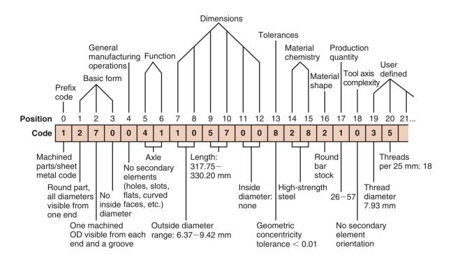
**Figure 38.12:** Typical multiClass code for a machined part. The routing sheet travels with the part from operation to operation. Source: Courtesy of Organization for Industrial Research.
