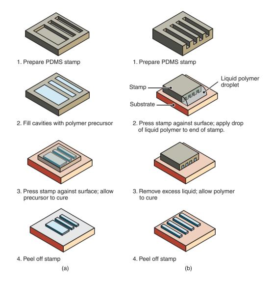
**Figure 28.18:** Soft lithography techniques. (a) Microtransfer molding (TM), and (b) micromolding in capillaries (MIMIC). *Source:* After Y. Xia and G.M. Whitesides.
