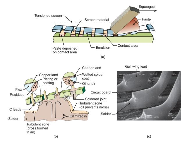
**Figure 32.7:** (a) Screening solder paste onto a printed circuit board in reflow soldering. (b) Schematic illustration of the wave-soldering process. (c) SEM image of a wave-soldered joint on surface-mount device. *Source:* (a) After V. Solberg.
