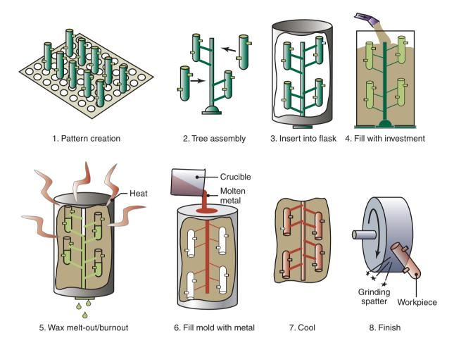
**Figure 20.19:** Manufacturing steps for investment casting with rapid-prototyped wax parts as blanks. This method uses a flask for the investment, but a shell method also can be used. *Source:* Courtesy of 3D Systems, Inc.
