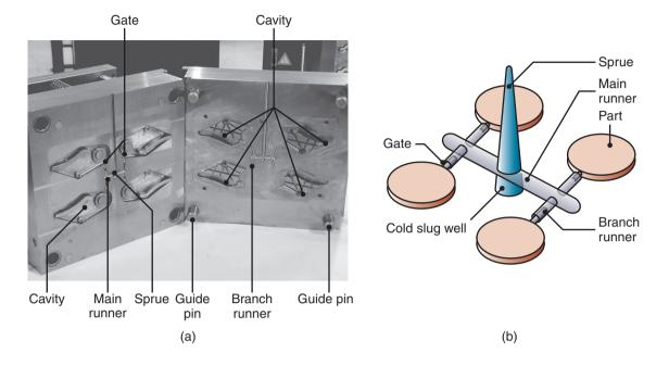
**Figure 19.10:** Illustration of mold features for injection molding. (a) Two-plate mold with important features identified. (b) Schematic illustration of the features in a mold. *Source:* Courtesy of Tooling Molds West, Inc.
