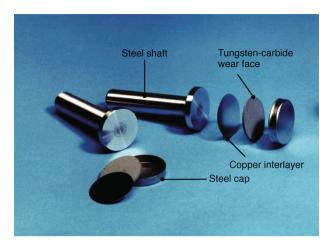
**Figure 17.17:** A valve lifter for heavy-duty diesel engines produced from a hot-isostatic-pressed carbide cap on a steel shaft. *Source:* Courtesy of the Metal Powder Industries Federation.
