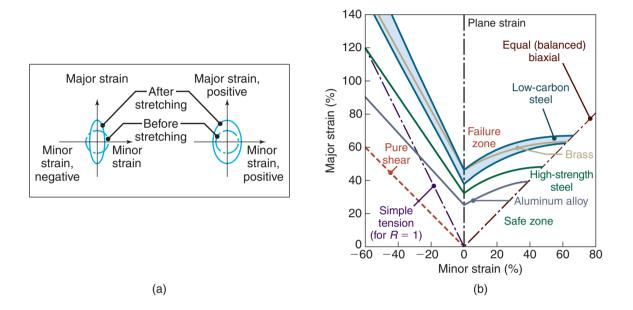
**Figure 16.14:** (a) Strains in deformed circular grid patterns. (b) Forming-limit diagrams (FLD) for various sheet metals. Although the major strain is always positive (stretching), the minor strain may be either positive or negative. R is the normal anisotropy of the sheet, as described in Section 16.3. *Source:* After S.S. Hecker and A.K. Ghosh.
