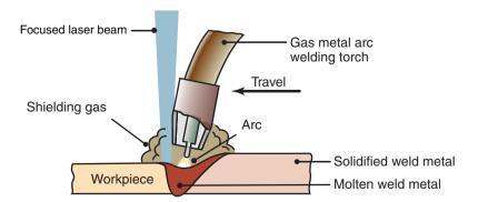
Figure 30.17: Schematic illustration of the Laser GMAW hybrid welding process. *Source:* Courtesy of Lincoln Electric.
