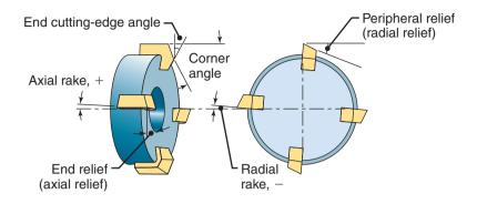
Figure 24.9: Terminology for a face-milling cutter.
