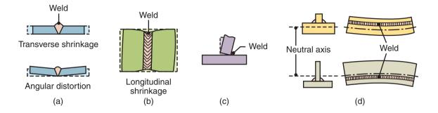
**Figure 30.25:** Distortion of parts after welding. Distortion is caused by differential thermal expansion and contraction of different regions of the welded assembly.
