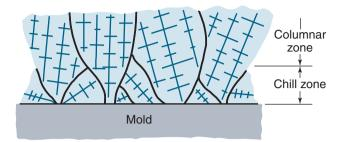
**Figure 10.3:** Development of a preferred texture at a cool mold wall; note that only favorably oriented grains grow away from the surface of the mold.
