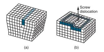
Figure 1.9: Types of dislocations in a single crystal: (a) edge dislocation and (b) screw dislocation.
