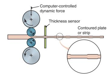
**Figure 13.7:** Production of tailor rolled blanks, with varying thickness in the rolling direction. A desired contour can be rolled into the workpiece, allowing for optimum placement of material.
