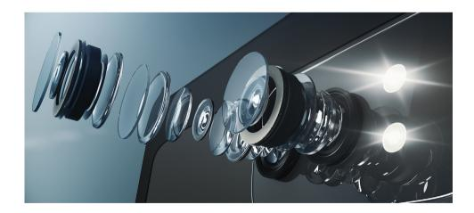
**Figure 29.1:** Exploded view of the camera in a smart phone. Perhaps the most widespread use of MEMS devices is in cameras and sensors of all kinds. *Source:* Shutterstock/Who is Danny.
