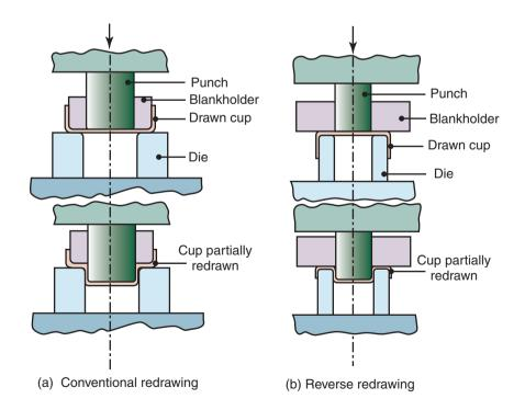
**Figure 16.37:** Reducing the diameter of drawn cups by redrawing operations: (a) conventional redrawing and (b) reverse redrawing. Small-diameter deep containers may undergo several redrawing operations.
