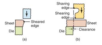
**Figure 16.9:** Schematic illustrations of the shaving process. (a) Shaving a sheared edge. (b) Shearing and shaving combined in one stroke.
