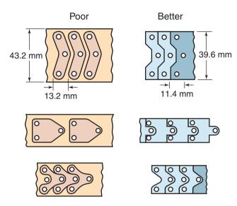
**Figure 16.60:** Efficient nesting of parts for optimum material utilization in blanking. *Source:* Courtesy of Society of Manufacturing Engineers.
