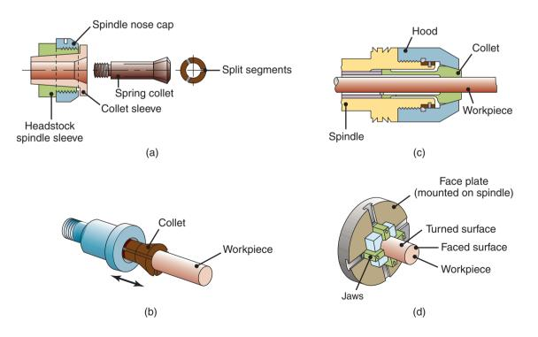
**Figure 23.8:** (a) and (b) Schematic illustrations of a draw-in type of collet. The workpiece is placed in the collet hole, and the conical surfaces of the collet are forced inward by pulling it with a draw bar into the sleeve. (c) A push-out type of collet. (d) Workholding of a workpiece on a face plate.
