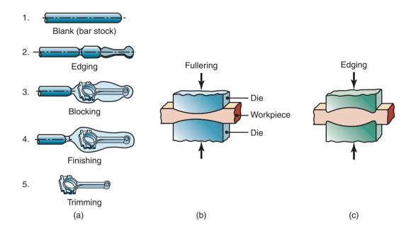
**Figure 14.8:** (a) Stages in forging a connecting rod for an internal combustion engine. Note the amount of flash required to ensure proper filling of the die cavities. (b) Fullering and (c) edging operations to distribute the material properly when preshaping the blank for forging.
