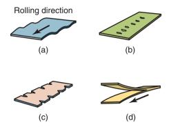
**Figure 13.9:** Schematic illustration of typical defects in flat rolling: (a) wavy edges; (b) zipper cracks in the center of the strip; (c) edge cracks; and (d) alligatoring.
