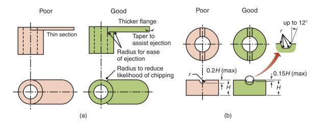
**Figure 17.27:** (a) Design features to use with unsupported flanges. (b) Design features for use with grooves. *Source:* Courtesy of Metal Powder Industries Federation.
