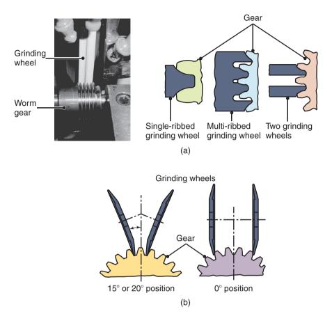
**Figure 24.36:** Finishing gears by grinding: (a) form grinding with shaped grinding wheels; (b) grinding by generating, using two wheels.
