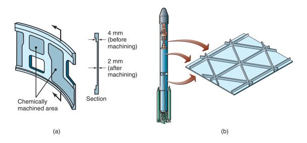
**Figure 27.2:** (a) Missile skin-panel section contoured by chemical milling to improve the stiffness-to-weight ratio of the part. (b) Weight reduction of space-launch vehicles by the chemical milling of aluminum-alloy plates. The plates are chemically milled after they have been formed into shape by a process such as roll forming or stretch forming. The design of the chemically machined rib patterns can readily be modified at minimal cost.
