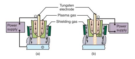
**Figure 30.7:** Two types of plasma-arc welding processes: (a) transferred and (b) nontransferred. Deep and narrow welds can be made by these processes at high welding speeds.
