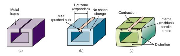
Figure 30.27: Distortion of a welded structure. Source: After J.A. Schey.
