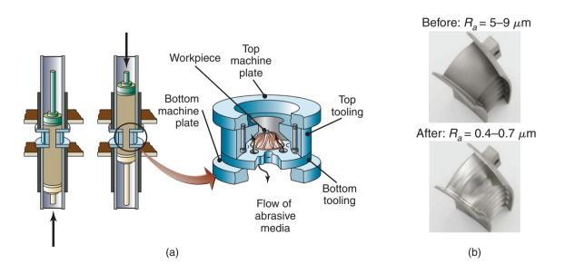
**Figure 26.34:** (a) Schematic illustration of abrasive-flow machining to deburr a turbine impeller. The arrows indicate movement of the abrasive media. Note the special fixture, which is usually different for each part design. (b) Valve fittings subjected to abrasive-flow machining to eliminate burrs and improve surface quality. *Source:* Courtesy of Kennametal Extrude Hone.
