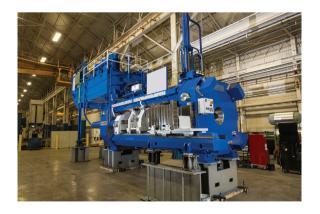
**Figure 15.19:** A 27-MN (2721-metric ton) Sutton aluminum extrusion press. This is the first of the Sutton MK-V extrusion press series built in the United States to SMS group Engineering specifications. Photo courtesy of SMS Group, Inc., Pittsburgh, PA.
