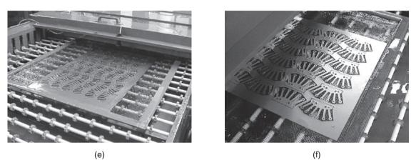
**Figure 27.19:** Processing sequence for photochemical etching of microsatellite components: (a) clean the raw material, (b) coat with photosensitive material, (c) expose with photographic tool, (d) develop a resist image, (e) etch, and (f) remove the resist. *Source:* Courtesy of R. Hoppe, VACCO Industries, Inc.
