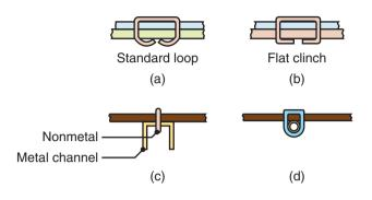
Figure 32.16: Typical examples of metal stitching.
