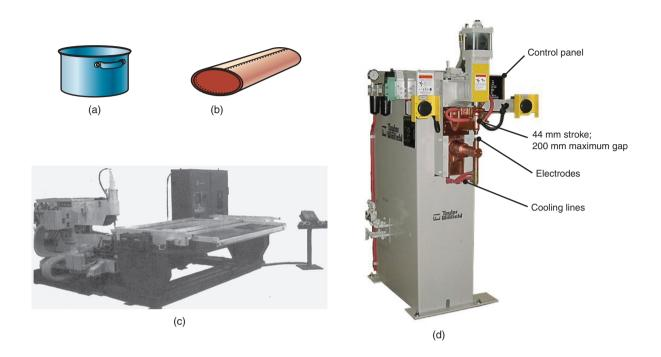
**Figure 31.8:** Spot-welded (a) cookware and (b) muffler. (c) An automated spot-welding machine. The welding tip can move in three principal directions. Sheets as large as  $2.2 \times 0.55$  m can be accommodated in this machine with proper workpiece supports. (d) A typical spot welding machine. *Source:* (c) and (d) Courtesy of Taylor-Winfield Technologies, Inc.
