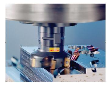
**Figure 24.3:** Photograph of the cutting action of a milling cutter that uses a number of inserts to remove metal in the form of chips. *Source:* Courtesy of Sandvik Coromant.
