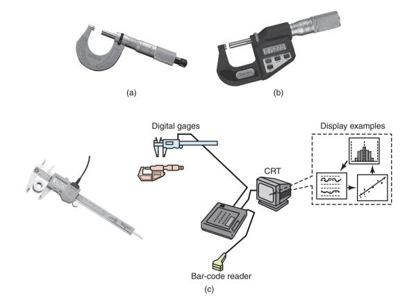
**Figure 35.2:** (a) A vernier (analog) micrometer. (b) A digital micrometer with a range of 0 to 25 mm and a resolution of 1.25  $\mu$ m; note that it is much easier to read dimensions on this instrument than on analog micrometers. (c) Schematic illustration showing the integration of digital gages with microprocessors for real-time data acquisition for statistical process control. *Source:* (a) Courtesy of L.C. Starrett Co. (b) Courtesy of Mitutoyo America Corp.
