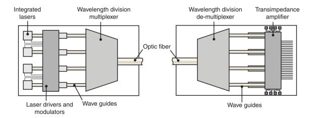
**Figure 29.26:** Schematic illustration of a photonic integrated circuit for data transmission. Numerous lasers, each producing a different wavelength of light, have their output signal modulated and combined into one fiber-optic cable by the wavelength division multiplexer (WDM Mux). The cable can extend thousands of kilometers to the receiving circuit, where the signal is separated into its components by a demultiplexer (WDM Demux), and then detected and amplified.
