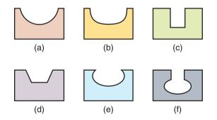
28.28. Referring to Fig. 28.24, sketch the shape of the holes generated from a circular mask.
