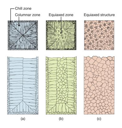
**Figure 10.2:** Schematic illustration of three cast structures of metals solidified in a square mold: (a) pure metals; (b) solid–solution alloys; and (c) structure obtained by using nucleating agents. *Source:* After G.W. Form, J.F. Wallace, J.L. Walker, and A. Cibula.
