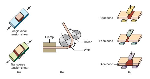
**Figure 30.28:** (a) Specimens for longitudinal tension-shear testing and for transfer tension-shear testing. (b) Wraparound bend-test method. (c) Three-point transverse bending of welded specimens.
