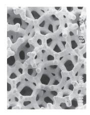
**Figure 6.4:** Structure of a metal foam used in orthopedic implants to encourage bone ingrowth. *Source:* Courtesy of Zimmer, Inc.
