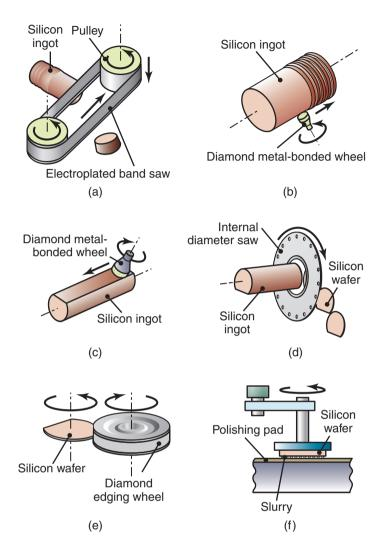
**Figure 28.6:** Finishing operations on a silicon ingot to produce wafers: (a) sawing the ends off the ingot; (b) grinding of the end and cylindrical surfaces of a silicon ingot; (c) machining of a notch or flat; (d) slicing of wafers; (e) end grinding of wafers; (f) chemical–mechanical polishing of wafers.
