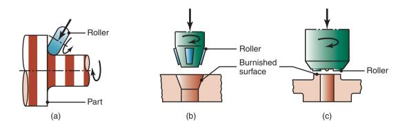
**Figure 34.1:** Burnishing tools and roller burnishing of (a) the fillet of a stepped shaft to induce compressive surface residual stresses for improved fatigue life; (b) a conical surface; and (c) a flat surface.
