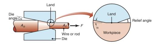
**Figure 15.20:** Process variables in wire drawing. The major processing variables in drawing are similar to those in extrusion, that is, reduction in cross-sectional area, die angle, frictional conditions along the die–workpiece interfaces, and drawing speed.
