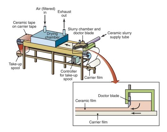
Figure 18.4: Production of ceramic sheets through the doctor-blade process.
