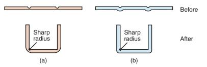
**Figure 16.64:** Application of (a) scoring or (b) embossing to obtain a sharp inner radius in bending. Unless properly designed, these features can lead to fracture. *Source:* Courtesy of Society of Manufacturing Engineers.
