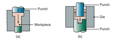
Figure 15.11: Two examples of cold extrusion; arrows indicate the direction of metal flow during extrusion.
