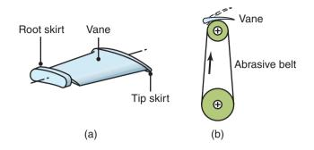
Figure 26.28: Turbine nozzle vane considered in Example 26.5.
