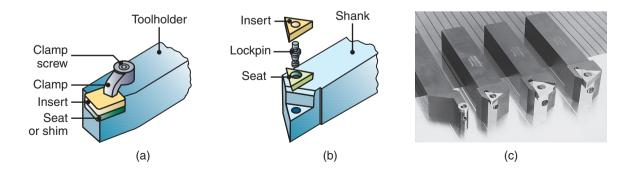
**Figure 22.3:** Methods of mounting inserts on toolholders: (a) clamping and (b) wing lockpins. (c) Examples of inserts mounted with threadless lockpins, which are secured with side screws. *Source:* Courtesy of Sandvik.
