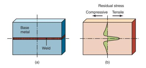
**Figure 30.26:** Residual stresses developed in (a) a straight-butt joint; note that the residual stresses shown in (b) must be balanced internally (see also Fig. 2.30.)
