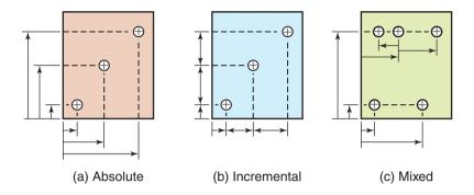
**Figure 37.6:** Positions of drilled holes in a workpiece. Three methods of measurements are shown: (a) Absolute dimensioning, referenced from one point at the lower left of the part; (b) Incremental dimensioning, made sequentially from one hole to another; and (c) Mixed dimensioning, a combination of both methods.
