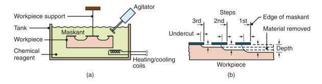
**Figure 27.3:** (a) Schematic illustration of the chemical-machining process; note that no forces or machine tools are involved in this process. (b) Stages in producing a profiled cavity by chemical machining; note the undercut.
