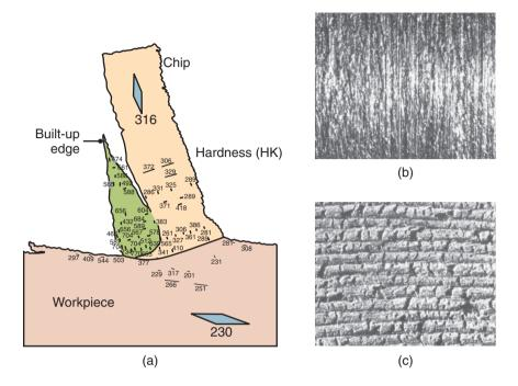
**Figure 21.6:** (a) Hardness distribution in a built-up edge in 3115 steel. Note that some regions within the built-up edge are as much as three times harder than the bulk metal being machined. (b) Surface finish produced in turning 5130 steel with a built-up edge. (c) Surface finish on 1018 steel in face milling. Magnifications:  $15 \times$ . *Source:* (b) and (c) Courtesy of TechSolve, Inc.
