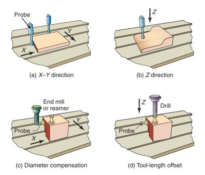
**Figure 25.6:** Touch probes used in machining centers for determining workpiece and tool positions and surfaces relative to the machine table or column. Touch probe (a) determining the x-y (horizontal) position of a workpiece, (b) determining the height of a horizontal surface, (c) determining the planar position of the surface of a cutter (*e.g.*, for cutter–diameter compensation), and (d) determining the length of a tool for tool-length offset.
