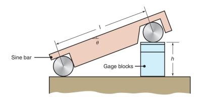
Figure 35.4: Schematic illustration of a sine bar.
