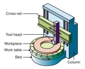
**Figure 23.19:** Schematic illustration of a vertical boring mill. Such a machine can accommodate workpiece sizes as large as 2.5 m in diameter.
