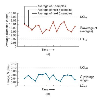
**Figure 36.5:** Control charts used in statistical quality control. The process shown is in good statistical control because all points fall within the lower and upper control limits. In this illustration, the sample size is 5 and the number of samples is 15.
