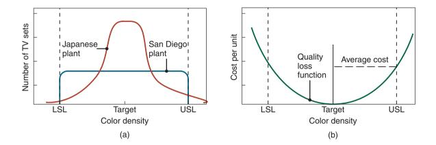
**Figure 36.2:** (a) Objective-function value distribution of color density for television sets. (b) Taguchi loss function, showing the average replacement cost per unit to correct quality problems.
