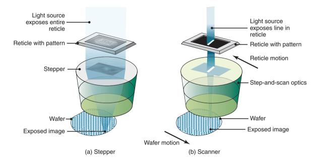
**Figure 28.12:** Schematic illustration of (a) wafer stepper technique for pattern transfer, and (b) wafer stepand-scan technique.
