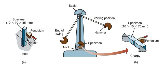
Figure 2.19: Impact test specimens. (a) Izod; (b) Charpy.
