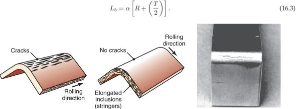
**Figure 16.17:** (a) and (b) The effect of elongated inclusions (stringers) on cracking as a function of the direction of bending with respect to the original rolling direction of the sheet. (c) Cracks on the outer surface of an aluminum strip bent to an angle of 90°. Note also the narrowing of the top surface in the bend area due to the Poisson effect.
