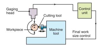
**Figure 37.15:** In-process inspection of a workpiece diameter in a turning operation. The system automatically adjusts the radial position of the cutting tool in order to produce the correct diameter.
