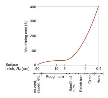
**Figure 26.35:** Increase in the cost of machining and finishing a part as a function of the surface finish required. This is the main reason that the surface finish specified on parts should not be any finer than is necessary for the part to function properly.
