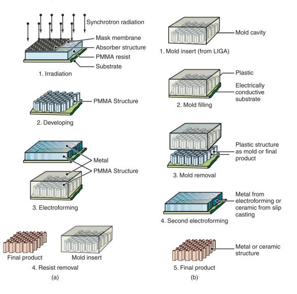
**Figure 29.17:** The LIGA (lithography, electrodeposition and molding) technique. (a) Primary production of a metal final product or mold insert. (b) Use of the primary part for secondary operations or replication. *Source:* Courtesy of IMM Institut für Mikrotechnik, Mainz, Germany.
