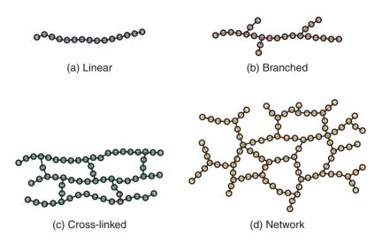
**Figure 7.5:** Schematic illustration of polymer chains. (a) Linear structure-thermoplastics such as acrylics, nylons, polyethylene, and polyvinyl chloride have linear structures. (b) Branched structure, such as in polyethylene. (c) Cross-linked structure—many rubbers, or elastomers, have this structure, and the vulcanization of rubber produces this structure. (d) Network structure, which is basically highly cross-linked. Examples are thermosetting plastics, such as epoxies and phenolics.
