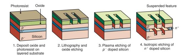
Figure 29.13: Schematic illustration of silicon micromachining by single-step plasma etching (SIMPLE) process.
