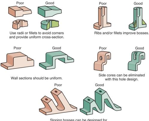
Sloping bosses can be designed for straight die parting to simplify die design.
