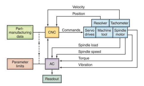
**Figure 37.13:** Schematic illustration of the application of adaptive control (AC) for a turning operation. The system monitors such parameters as cutting force, torque, and vibrations; if these parameters are excessive, it modifies process variables (such as feed and depth of cut) to bring the parameters back to acceptable levels.
