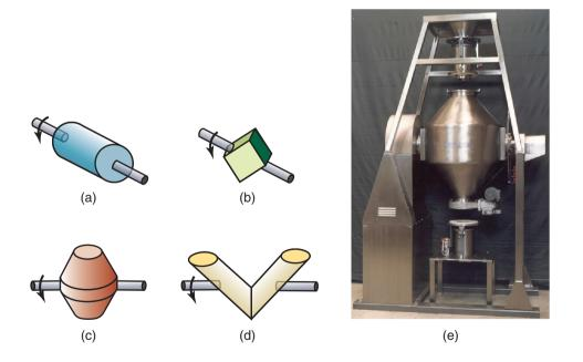
**Figure 17.8:** Powder mixing and blending. (a) through (d) Some common bowl geometries for mixing or blending powders. (e) A mixer suitable for blending metal powders. Since metal powders are abrasive, mixers rely on the rotation or tumbling of enclosed geometries, as opposed to using aggressive agitators. *Source:* Courtesy of Kemutec Group, Inc.
