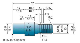
**Figure IV.3:** A machined and threaded part, showing various dimensions and tolerances; all dimensions are in mm. Note that some tolerances are only a few tenths of an mm.
