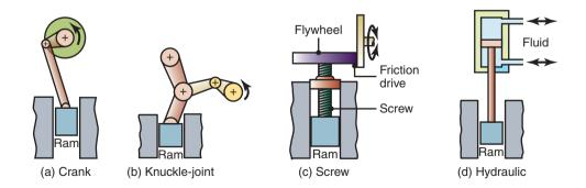
**Figure 14.19:** Schematic illustration of the principles of various forging machines. (a) Mechanical press with an eccentric drive; the eccentric shaft can be replaced by a crankshaft to give up-and-down motion to the ram. (b) Knuckle-joint press. (c) Screw press. (d) Hydraulic press.
