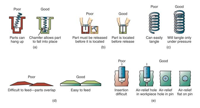
Figure I.6: Redesign of parts to facilitate assembly. Source: After G. Boothroyd and P. Dewhurst.
