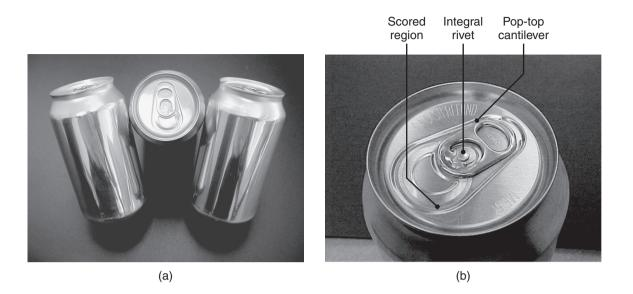
**Figure 16.40:** (a) Aluminum beverage cans; note the smooth surface. (b) Detail of the can lid, showing the integral rivet and scored periphery for the pop-top.
