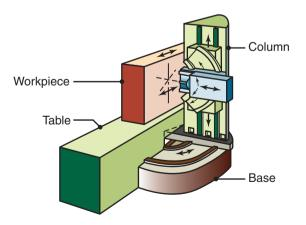
**Figure 24.21:** Schematic illustration of a five-axis profile milling machine. Note that there are three principal linear and two angular movements of machine components.
