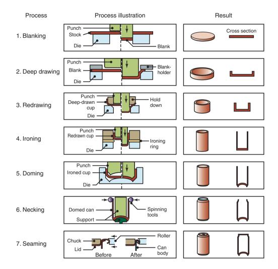
Figure 16.31: The metal-forming processes involved in manufacturing two-piece aluminum beverage cans.
