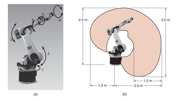
**Figure 37.17:** (a) Schematic illustration of a 6-axis KR-30 KUKA robot; the payload at the wrist is 30 kg and repeatability is  $\pm$  0.15 mm. The robot has mechanical brakes on all of its axes, which are directly coupled to one another. (b) The work envelope of the robot, as viewed from the side. *Source:* Courtesy of KUKA Robotics Corp.
