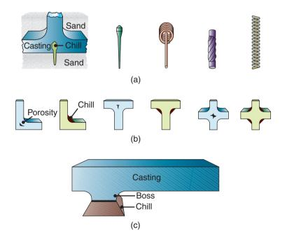
**Figure 10.16:** Various types of (a) internal and (b) external chills (dark areas at corners) used in castings to eliminate porosity caused by shrinkage. Chills are placed in regions where there is a larger volume of metal, as shown in (c).
