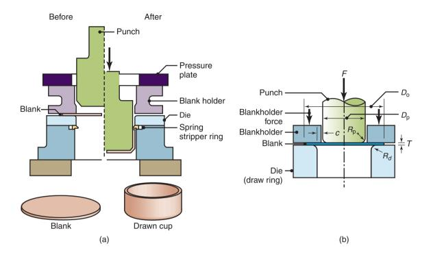
**Figure 16.32:** (a) Schematic illustration of the deep-drawing process on a circular sheet-metal blank. The stripper ring facilitates the removal of the formed cup from the punch. (b) Process variables in deep drawing. Except for the punch force, *F*, all the parameters indicated in the figure are independent variables.
