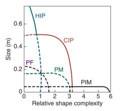
**Figure 17.15:** Capabilities, with respect to part size and shape complexity, available in various PM operations. PF = powder forging. *Source:* Courtesy of the Metal Powder Industries Federation.
