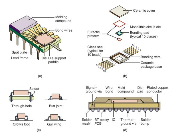
**Figure 28.32:** Schematic illustrations of various IC packages: (a) dual-in-line package (DIP); (b) flat ceramic package; (c) common surface-mount configurations; (d) ball-grid arrays.
