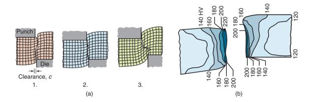
**Figure 16.3:** (a) Effect of the clearance, *c*, between punch and die on the deformation zone in shearing. As the clearance increases, the material tends to be pulled into the die rather than be sheared. In practice, clearances usually range between 2% and 10% of the thickness of the sheet. (b) Microhardness (HV) contours for a 6.4-mm thick AISI 1020 hot-rolled steel in the sheared region.
