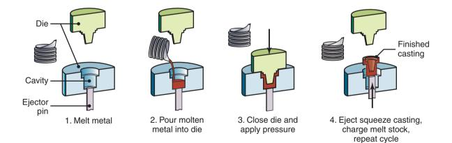
**Figure 11.24:** Sequence of operations in the squeeze-casting process. This process combines the advantages of casting and forging.
