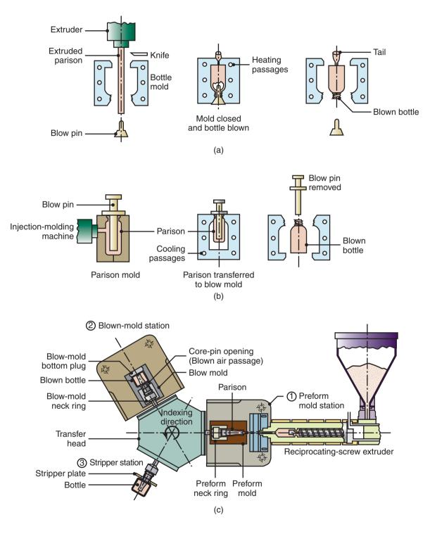
**Figure 19.14:** Schematic illustrations of (a) the extrusion blow-molding process for making plastic beverage bottles; (b) the injection blow-molding process; and (c) a three-station injection blow-molding machine for making plastic bottles.
