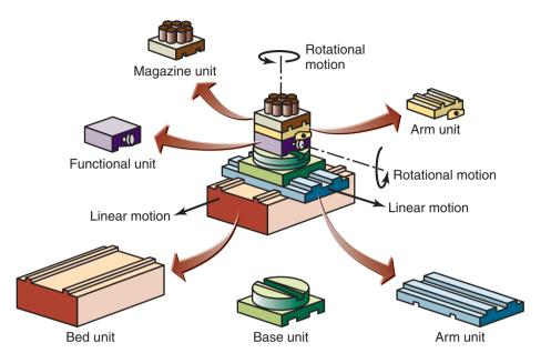
**Figure 25.11:** Schematic illustration of the assembly of different components of a reconfigurable machining center. *Source:* After Y. Koren.
