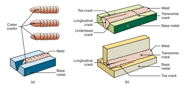
**Figure 30.23:** Types of cracks developed in welded joints. The cracks are caused by thermal stresses, similar to the development of hot tears in castings, as shown in Fig. 10.14.
