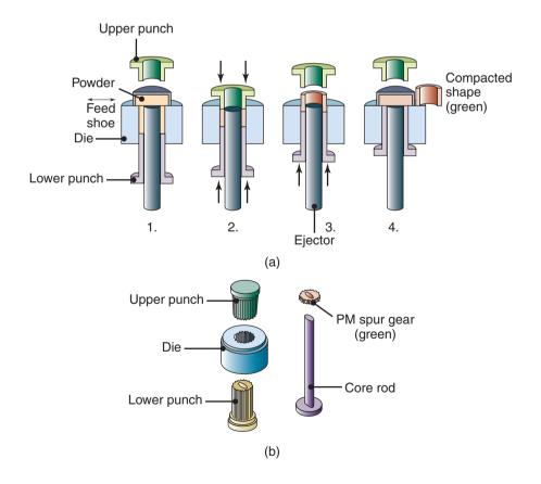
**Figure 17.9:** (a) Compaction of metal powder to form a bushing. The pressed-powder part is called green compact. (b) Typical tool and die set for compacting a spur gear. *Source:* Courtesy of the Metal Powder Industries Federation.
