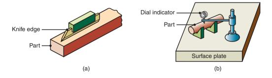
**Figure 35.6:** Measuring straightness manually with (a) a knife-edge rule and (b) a dial indicator. *Source:* After F.T. Farago.
