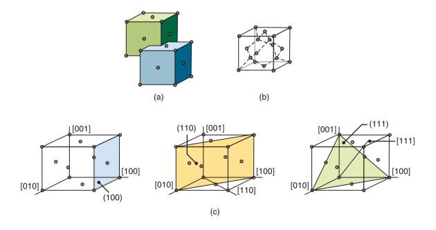
**Figure 28.5:** Crystallographic structure and Miller indices for silicon. (a) Construction of a diamond-type lattice from interpenetrating face-centered cubic cells; one of eight penetrating cells is shown. (b) Diamond-type lattice of silicon; the interiors have been shaded in color. (c) Miller indices for a cubic lattice.
