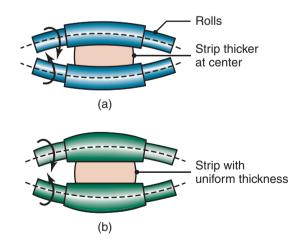
**Figure 13.4:** (a) Bending of straight cylindrical rolls caused by roll forces. (b) Bending of rolls ground with camber, producing a strip with uniform thickness through the strip width. Deflections have been exaggerated for clarity.
