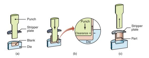
**Figure 15.14:** Schematic illustration of the impact-extrusion process. The extruded parts are stripped by the use of a stripper plate, because they tend to stick to the punch.
