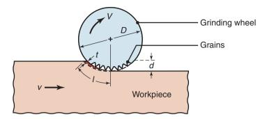
**Figure 26.11:** Schematic illustration of the surface-grinding process, showing various process variables. The figure depicts conventional (up) grinding.
