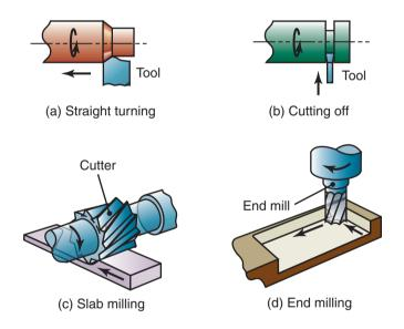
Figure 21.1: Some examples of common machining operations.
