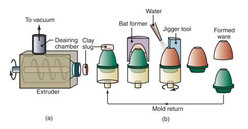
Figure 18.5: (a) Extruding and (b) jiggering operations.
