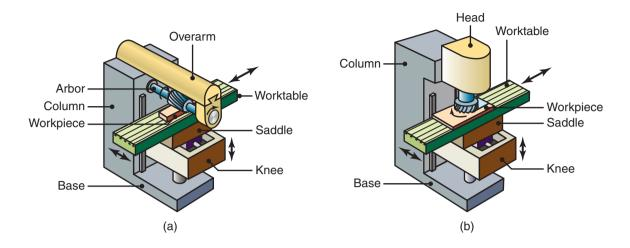
**Figure 24.18:** Schematic illustration of (a) a horizontal-spindle column-and-knee-type milling machine and (b) vertical-spindle column-and-knee-type milling machine. *Source:* After G. Boothroyd.
