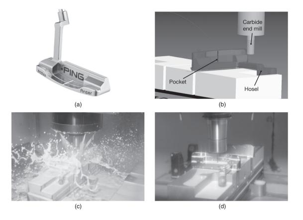
**Figure 24.38:** (a) The Ping Anser<sup>®</sup> golf putter; (b) CAD model of rough machining of the putter outer surface; (c) rough machining on a vertical machining center; (d) machining of the lettering in a vertical machining center; the operation was paused to take the photo, as normally the cutting zone is flooded with a coolant. *Source:* Courtesy of Ping Golf, Inc., Phoenix, Arizona.
