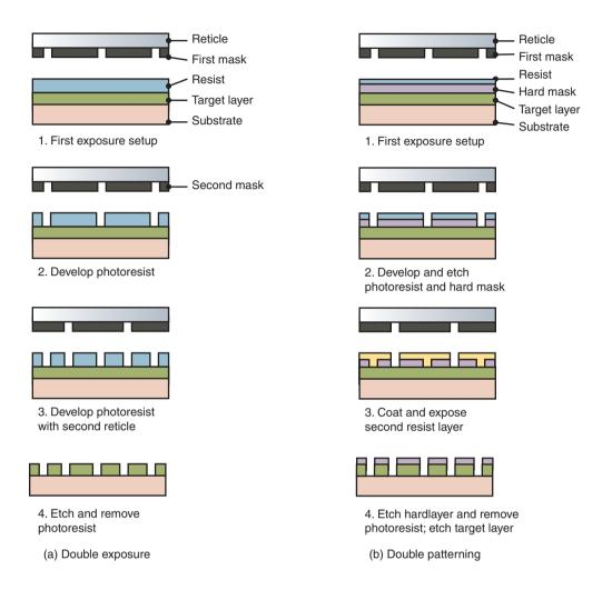
**Figure 28.14:** Pitch splitting lithography. (a) Double exposure (DE) process; (b) double patterning (DP) process, also known as the LELE (lithography-etch-lithography-etch) process.
