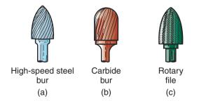
Figure 24.31: Types of burs used in burring operations.
