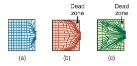
**Figure 15.6:** Types of metal flow in extruding with square dies. (a) Flow pattern obtained at low friction or in indirect extrusion. (b) Pattern obtained with high friction at the billet–chamber interfaces. (c) Pattern obtained at high friction or with cooling of the outer regions of the billet in the chamber. This type of pattern, observed in metals whereby their strength increases rapidly with decreasing temperature, leads to a defect known as *pipe*, or *extrusion defect*.
