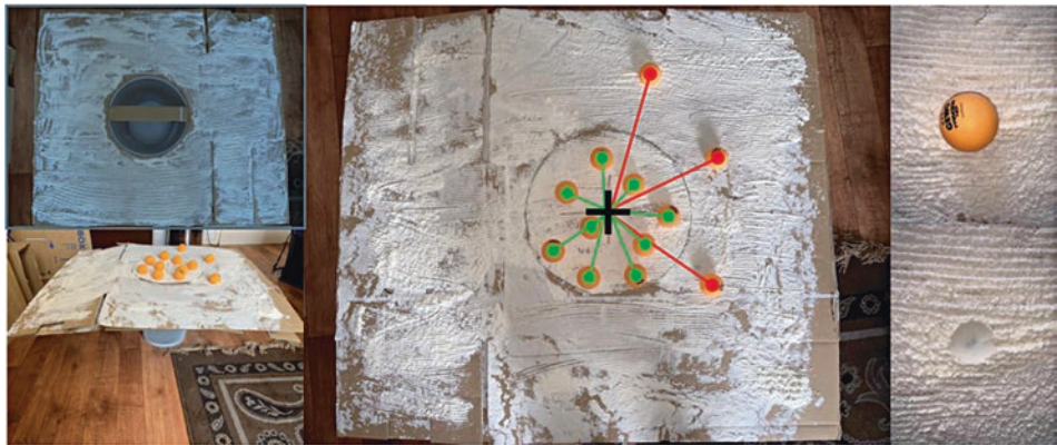
Fig. 3.25a–c Recording device for deviation determination
